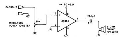
Figure 3: In the TONOUT electronics, an LM386 audio-amplifier chip is driven by the CASSOUT signal. The output of the LM386 drives a small speaker.
