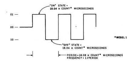
Figure 4: A timing loop turns on the CASSOUT signal and then turns it off. The same frequency count is used for both the on and off delays; hence, the period of the tone is twice the delay time.
