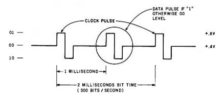
Figure 2: The recording technique for 500 bps uses a clock pulse spaced at 2-ms intervals. A data pulse at the midpoint between clock pulses represents a 1; the absence of a data pulse represents a 0.
