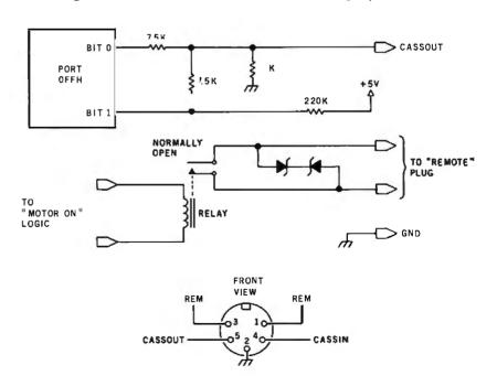
**Figure 1:** Model I/III cassette output is performed by a two-bit latch that generates three voltage levels. The three voltage levels can produce a square wave with a positive-going pulse, a negative-going pulse, and a zero level. A motor relay connects two normally open contacts.
