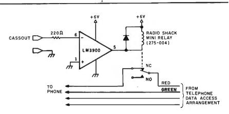
**Figure 10:** The telephone-dialing circuit uses an operational amplifier to trigger a small relay. The relay opens and closes the telephone line through the Data Access Arrangement to simulate a rotary-dial pulse.
