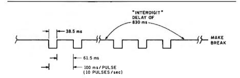
**Figure 11:** TELDIL breaks the circuit for 38.5 ms. Pulses are spaced at 100-ms intervals, representing 10 pulses per second. An interdigit delay of 830 ms separates the pulse trains for each digit.
