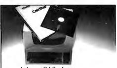
A glance at CalcStar features Runs on CP/M version 2.0 or above, with 80column screen, addressable cursor, and at least 48K memory. 56K or more is recommended for
