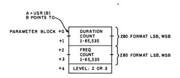
Figure 5: Three parameters are used to interface to TONOUT from BASIC. A duration count is held in two bytes, a frequency count in two bytes, and a level in one byte. The counts are in standard Z80 address format: least significant byte followed by most significant byte.
