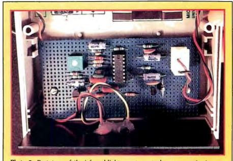
**Photo 2:** Prototype of the infrared-light remote-control or communication receiver of figure 4.
