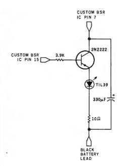
Figure 7: Modification of the hand-held ultrasonic transmitter of the BSR X-10 Home Control System that converts it to infrared-light operation.
