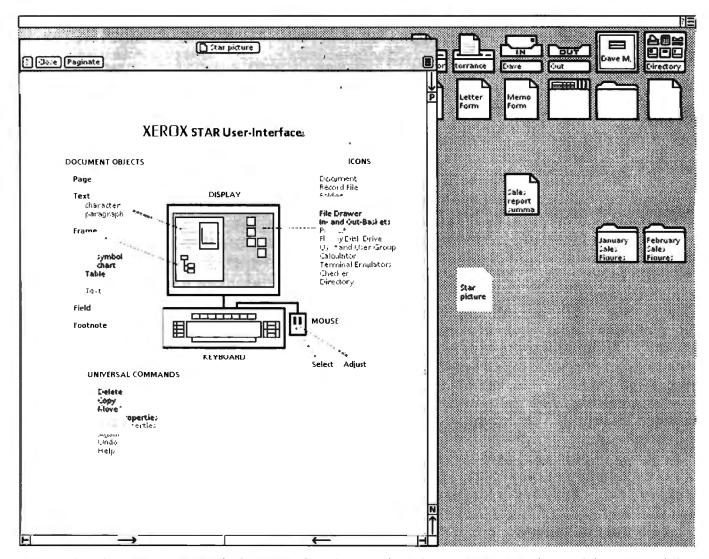
Figure 2: A Desktop as it appears on the Stur screen. Several commonly used icons appear across the top of the screen, including documents to serve as "form-pad" sources for letters, memos, and blank paper. An open window displaying a document containing an illustration is also shown.
