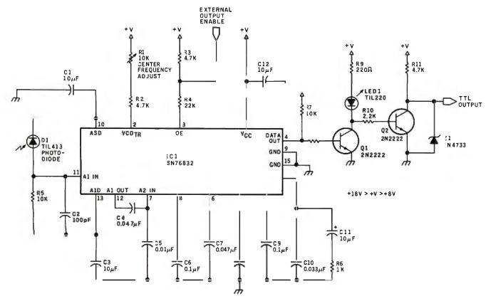
Figure 4: Schematic diagram of a remote-control or communication circuit based on the SN76832AN. This circuit is set up for use at 40 kHz, although the voltage-controlled oscillator can be adjusted from 20 kHz to 70 kHz. Any voltage from +8 V to +18 V may power the circuit.
