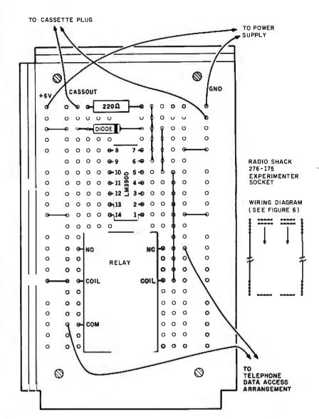
**Figure 13:** The TELDIL circuit is mounted on a project board. The relay leads can be trimmed, "built-up" with solder, and pushed into the project-board holes.
