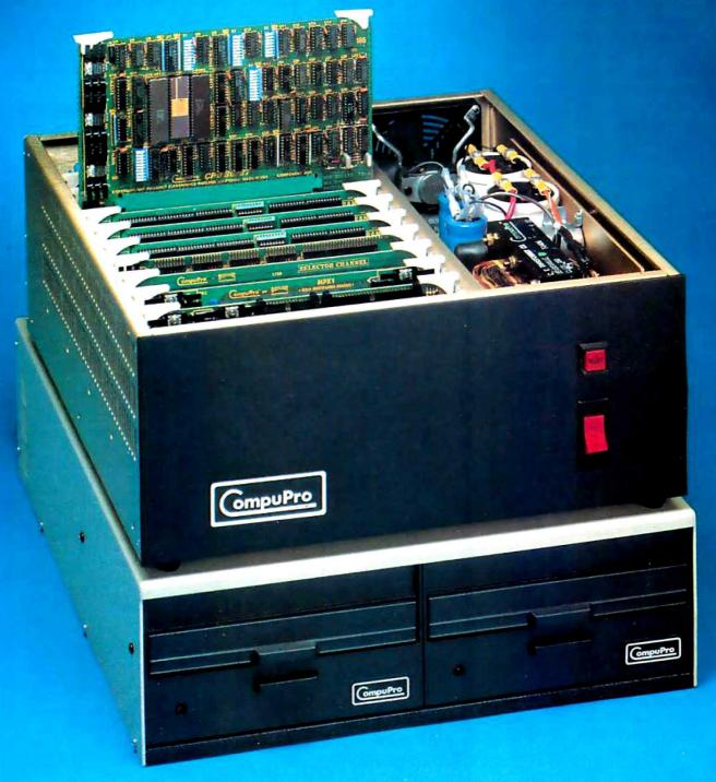
Pictured: CompuPro System Enclosure, Dual Disk Drive Enclosure, Disk 1, MPX, Selector Channel, and RAM 16.
