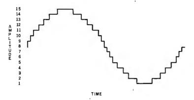
Figure 3: An amplitude-versus-time graph of the sine wave sound produced by listing 2.
