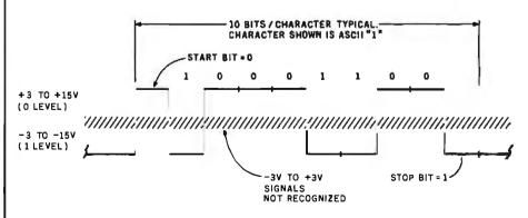
Figure 14: Logic is inverted in standard RS-232C signals. A 1 is represented by a negative voltage; a 0 by a positive voltage. Voltage levels from -3 to +3 V will not be recognized as legitimate values.
