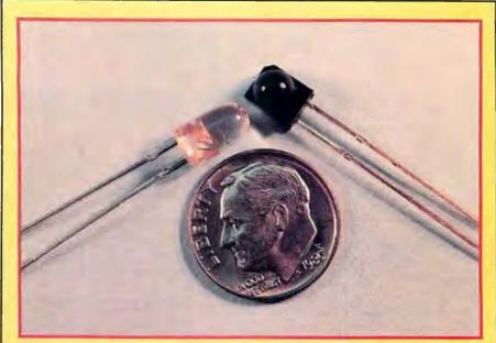
**Photo 1:** The TIL413 infrared-sensitive PIN photodiode (right) and the TIL39 infrared light-emitting diode (left).
