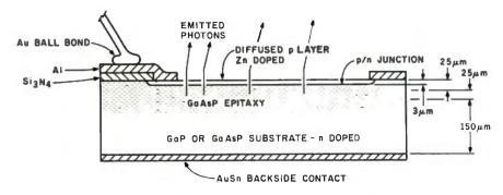
Figure 2: Cross section of the structure of a standard visible red light-emitting diode.
