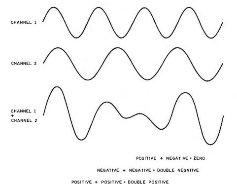
**Figure 1:** Complex waveform generation from the addition of waveforms.
