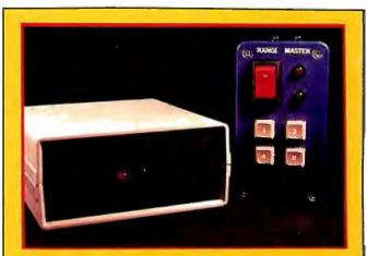
Photo 4: The assembled infrared remote-control/communication system. On the left is the infrared receiver; the transmitter is to the right. The TIL413 photodiode is the small projection to the right of center of the receiver's front panel; the small projection on the left is a visible red LED that lights when the infrared carrier is detected.
