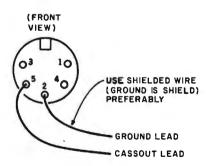
Figure 8: Two wires are connected to the 5-pin DIN plug for the cassette port. Shielded wire is preferable, but any wire will suffice.
