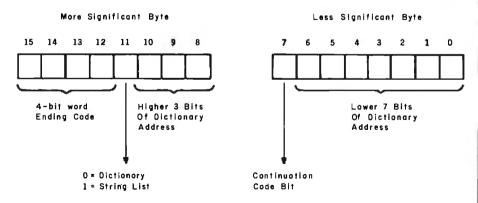
Figure 1: Diagram of a binary-coded text pointer. Of the 16 bits available, 10 are allocated to dictionary addressing, four define the word-ending code (given in table 1), one identifies the dictionary being addressed, and one is a continuation code. In a text stream, the less significant byte appears first. If bit 7 is a 0, this signals that the more significant byte is all zeros and that the next byte is the less significant byte of the next pointer.
