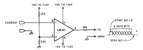
**Figure 15:** The SEROUT project uses an operational amplifier to generate a positive and negative voltage representing RS-232C data signals. Any convenient positive and negative voltage may be used.
