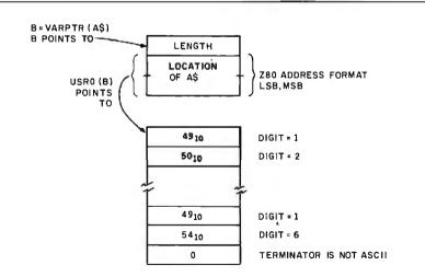
**Figure 12:** BASIC passes a pointer to TELDIL. The pointer references a list of ASCII digits representing decimal values; the list is terminated by any non-ASCII value, e.g., binary 0.
