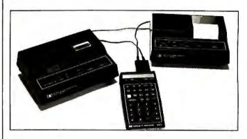
Photo 2: HP-41C connected to an HPIL Module, Digital Cassette Drive, and Thermal Printer/Plotter in the loop.
