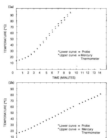
Figure 1: Tracking Strawberry Tree's thermometer probe versus a laboratory mercury thermometer. Figure 1a shows responses to an 8.89°C/minute rate of change; figure 1b shows responses to a 4.57°C/minute rate of change.
