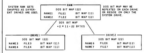
**Figure 8:** Swapping disk directories. As each disk is accessed, the disk directory is read from the disk and placed into RAM.
