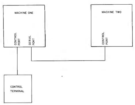
**Figure 1:** A simple RS-232C serial connection between two computers can provide the necessary communications interface to create a multiprocessing system.
