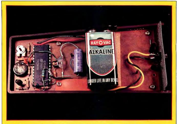
Photo 6: Interior view of the modified BSR X-10 hand-held transmitter, modified according to figure 7.
