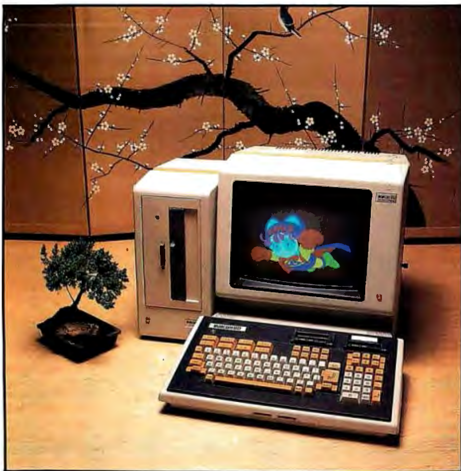
Photo 15: The Bubcom80's high-resolution monitor has a contour at the bottom that lets it fit snugly against the keyboard/processor enclosure. Slots in the top of the keyboard enclosure accept bubble-memory cartridges.
