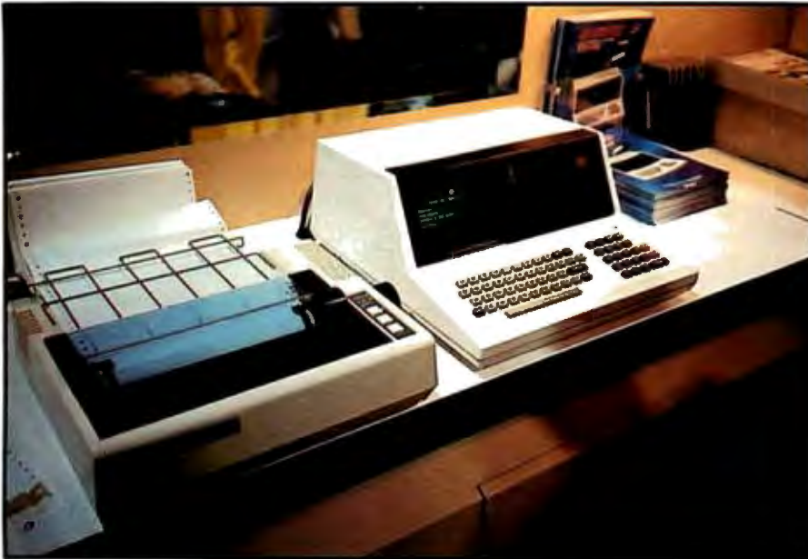
Photo 1: Casio's FX-9000P personal computer was finally introduced at the January Consumer Electronics Show. Using a Z80 look-alike, the basic unit comes with 12K bytes of ROM and one 4K-byte CMOS RAM pack with battery backup. RAM is expandable to 32K bytes, and a 16K-byte dynamic RAM pack is also available. The button-type keyboard contains only 67 keys but allows one-key access to many scientific and statistical functions. The printer is manufactured by Epson.
