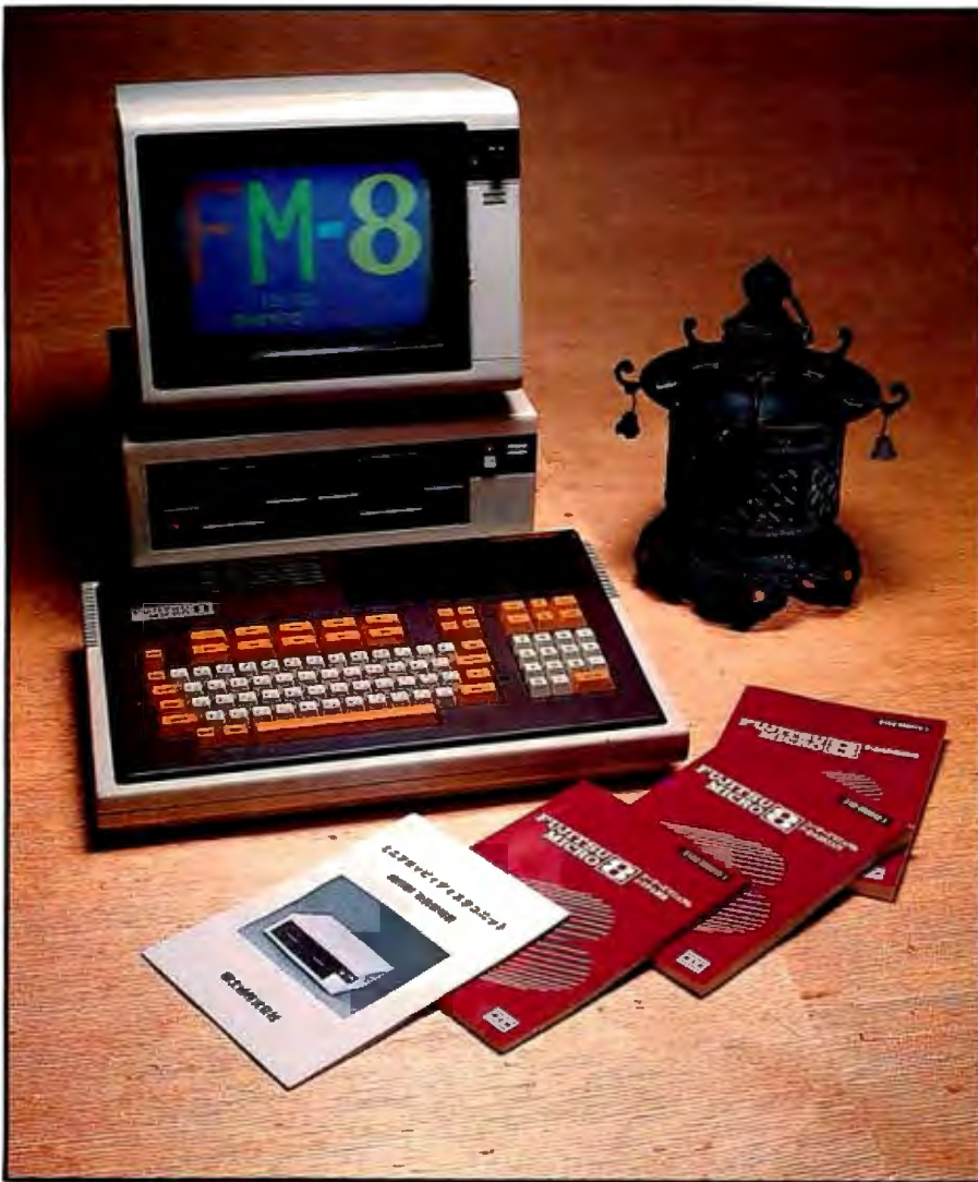
Photo 13: The Fujitsu FM-8 computer. Shown here are the keyboard/processor module, color monitor, and two disk drives, all connected together with lengthy cables for ease of rearrangement. Other optional hardware includes a printer, modem, joystick, and Z80-processor card.
