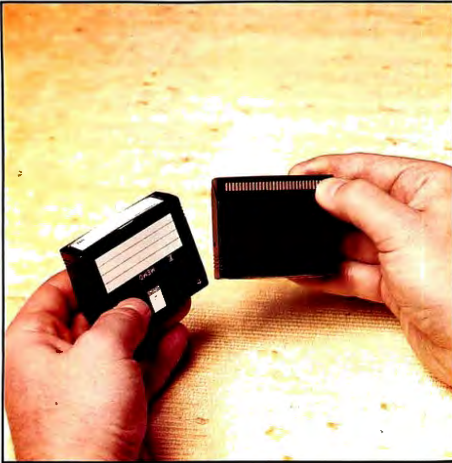
Photo 17: Each Bubcom bubble-memory cartridge holds 32K bytes. The white slide is a write-protect key.
