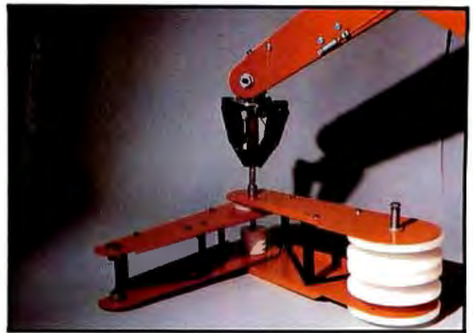
Photo 4: A mechanical assistant can speed the assembly of the arm.
