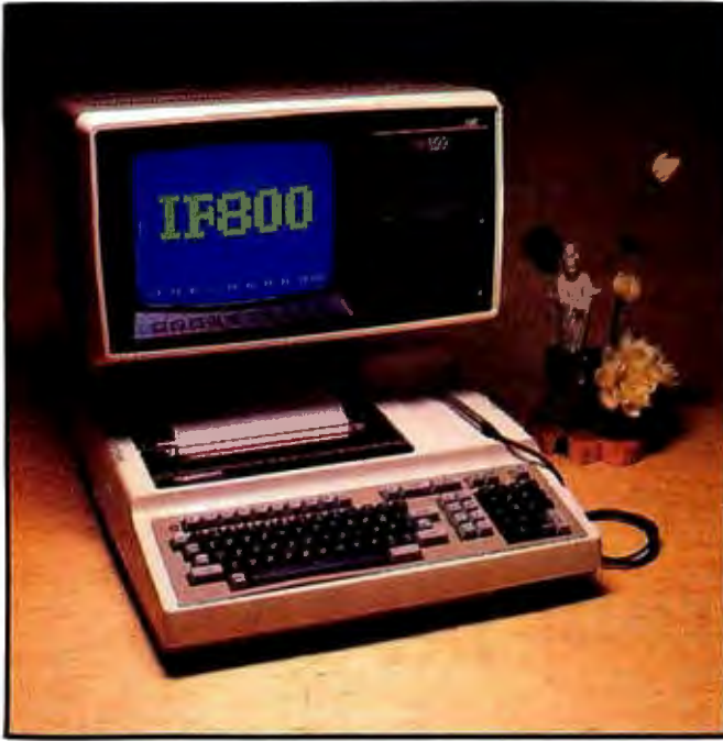
Photo 1: The BMC if800 computer. Shown here is the basic machine consisting of a keyboard/processor module, two floppy-disk drives, a color video monitor, and a unique built-in printer. Notice the 10 "super-function" keys along the bottom of the display screen. These are fully programmable function keys that can be used for menu selection or other forms of interaction in programs.
