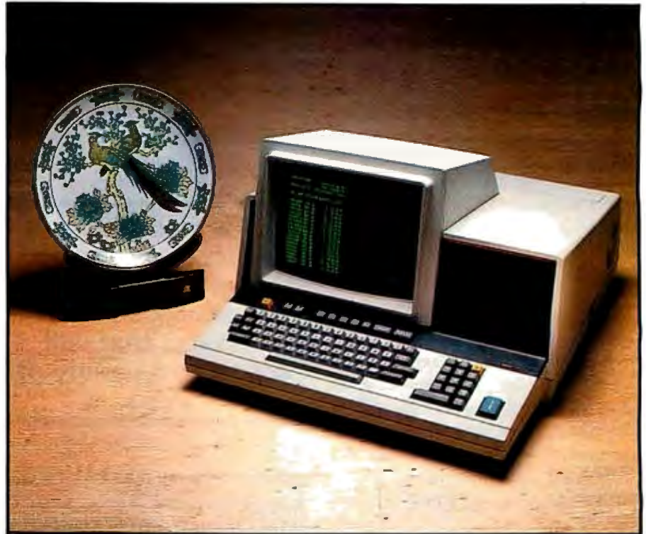
Photo 5: The Canon CX-1 computer. All the parts of the basic machine (keyboard, processor, two disk drives, and green video-display screen) are contained within a single molded plastic case.
