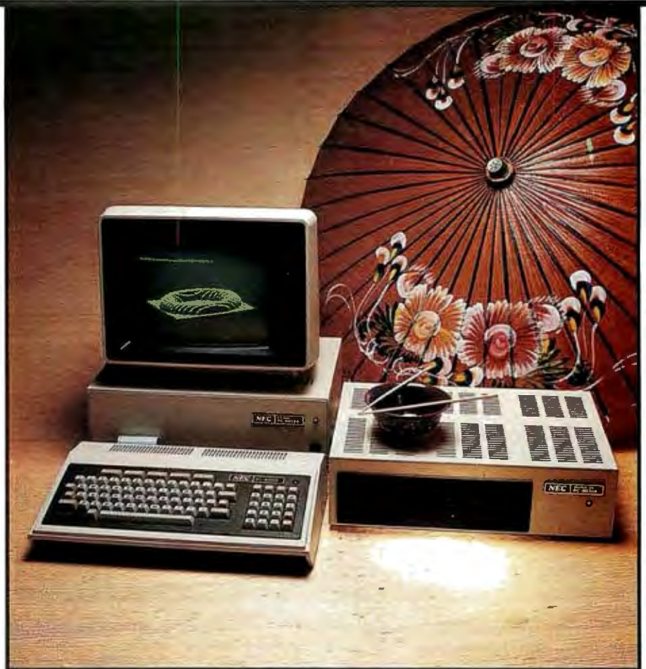
Photo 7: NEC's PC-8001A together with the color monitor, PC-8012 I/O unit, and PC-8032 dual floppy-disk drive.
