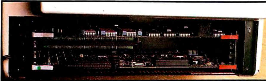
Photo 16: The Bubcom color-console/expansion box has slots for four 30.5-cm (12-inch) circuit boards.
