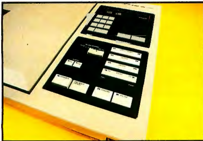
Photo 6: The Pioneer VP-1000's control panel. The VP-1000 is distinguished from other level-one players by its ability to directly access a videodisc frame and its remote-control unit.
