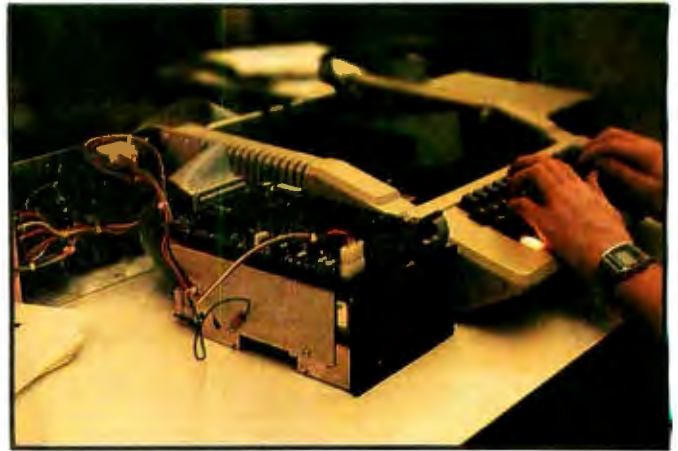
Photo 4: The Xebec 5-megabyte hard disk and controller kit for $1295.
