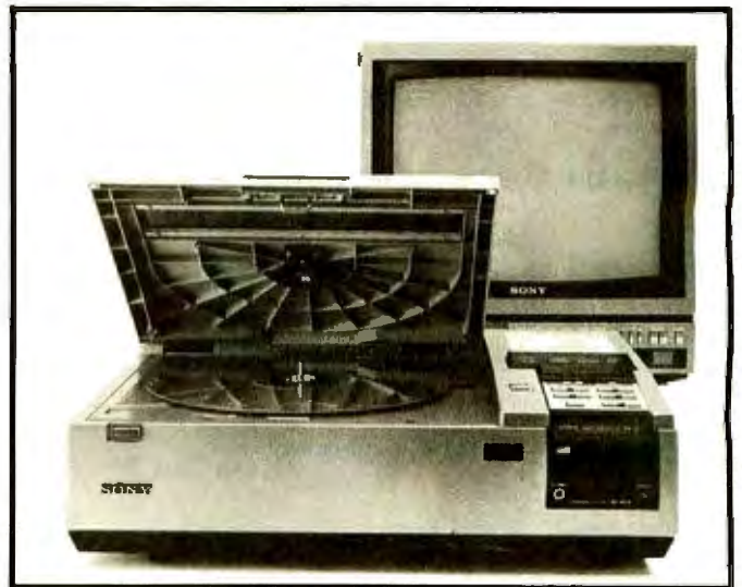
Photo 8: The Sony LDP-1000 (level-two) optical reflective videodisc player, which has a built-in RS-232C interface.
