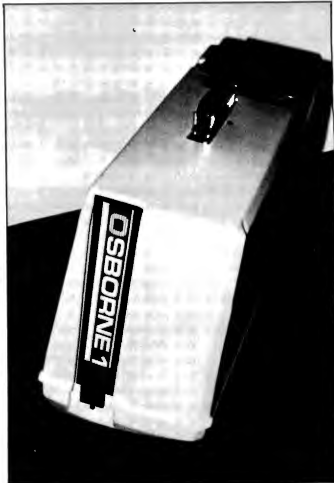
Photo 6: The Osborne 1 when closed up. The handle makes it easy to carry, but the sloping keyboard (which becomes the bottom) makes it sit at an angle. It has the feel of a lightweight sewing machine.
