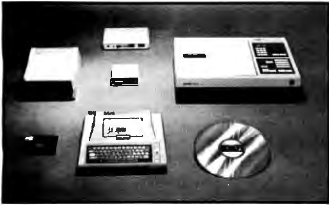
Photo 9: The Discmaster 5000 by New Media Graphics, a complete level-three system using the Pioneer VP-1000 and an Atari 400 computer.
