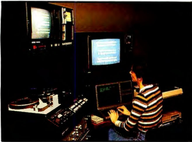
Photo 12: A videodisc simulator/editor developed by the Videodisc Design/Production Group. The Bosch BCN-50 1-inch helical VTR (left) serves as a surrogate disc player but with the added capability of offline insert edit capability with "broadcast quality."
