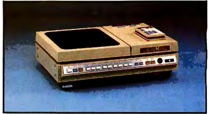
Photo 7: The Discovision Associates (DVA) PR-7820 "industrial" (level-two) optical reflective videodisc player. The DVA PR-7820's EPROMs have been updated twice (Models 2 and 3), resulting in faster search times and increased user-definable functions. Two-way communication between computer and disc is possible.
