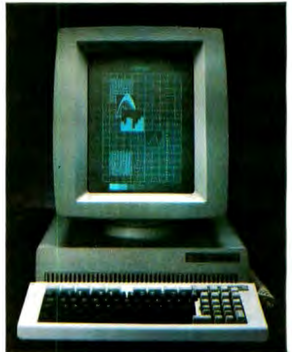
Photo 1: The Corvus Concept computer, which features a 68000 processor and a 120-column by 66-line display. Suggested retail price is $4995.
