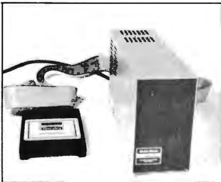
Photo 2: Color Computer disk drive, controller cartridge, and ribbon cable. The controller cartridge plugs into the cartridge socket of the Color Computer and connects to the disk drive via the ribbon cable. The disk drive has its own power cord.
