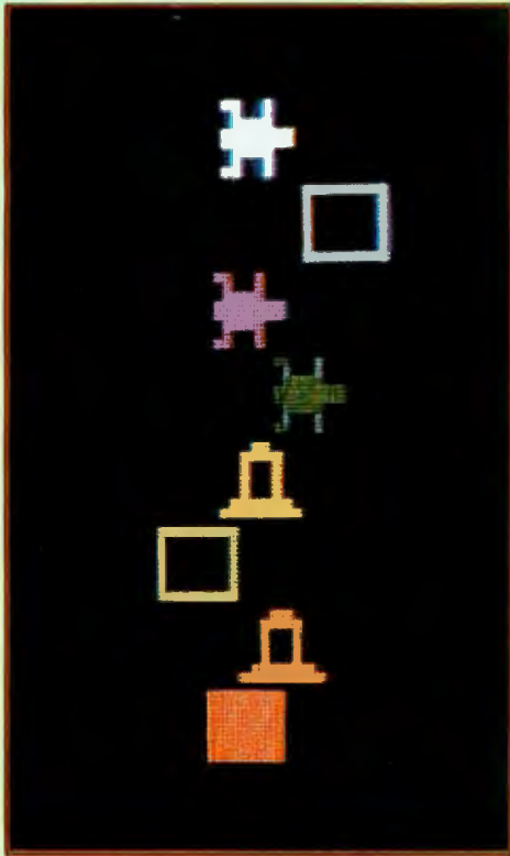
Photo 8: The Logo procedures developed at Terrapin Inc. provide you with commands such as SETSHAPE, SETCOLOR, and SXY. You can map out your own sprite shapes and incorporate them into the routines, but some predefined patterns are provided, including a box, a rocket, a turtle, and a block.
