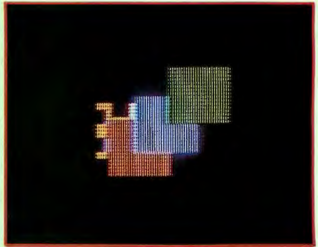
Photo 1: A step-by-step illustration of the use of sprites and the concept of plane priority. The yellow turtle (sprite 3) is programmed to pass from left to right past the green box (sprite 0), the blue box (sprite 1), and the red box (sprite 2). The transparent pattern plane and backdrop cause the background to be black.
