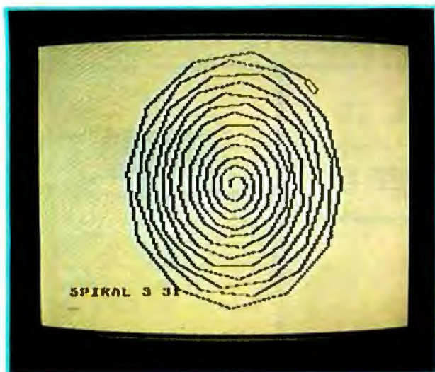
A spiral drawn with Color Logo turtle graphics. Note that text and graphics can be mixed on the same screen. The oblong object at the end of the spiral trail is the Color Logo turtle.
