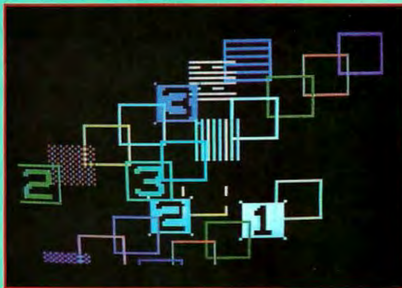
Photo 6: The display can get complicated when 24 sprites are visible.
