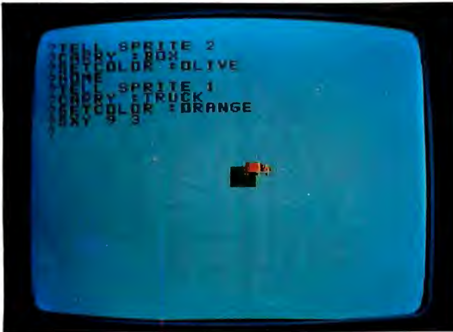
Photo 2: Priority in TI Logo sprites. The sprite with the lower number (a truck) appears to be on top of the sprite with the higher number (a box).
