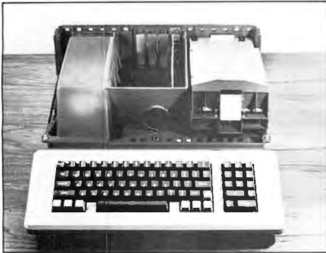
Photo 3: The Apple III with its main cover removed. The power supply is housed in the enclosure visible to the left, I/O card slots are in the center, and the disk drive is on the right. The entire Apple III is built around a single thin-wall aluminum casting that provides both support and shielding.
