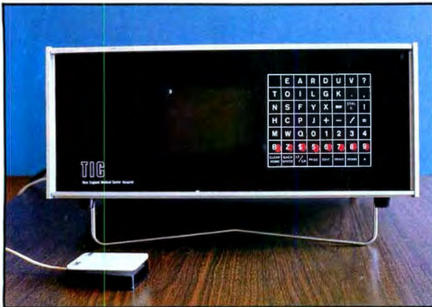
Photo 2: The Tufts Interactive Communicator, developed in 1972, was an early scanning communication device. It employed all TTL circuitry and used a dedicated 5-inch monitor to display 1024 characters.
