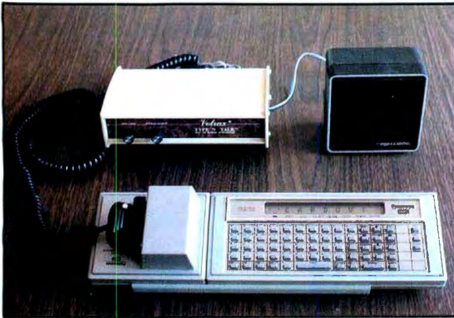
Photo 3: The HHC when used as a scanning communicator (a latter-day TIC) uses the LCD to display rows of characters. The Votrax Type-N-Talk and a Radio Shack speaker complete the communication device. A printer can also be added. (The first row of the TIC array is shown on the LCD.)
