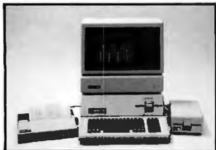
Photo 1: A view of the Apple III, the Profile hard-disk drive, and the Monitor III showing a sample of Visicalc III on the screen.
