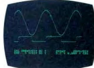
Cross-cursor indicates point where aScope™ digital voltmeter (DVM) is calculating waveform voltage for display at bottom of screen
