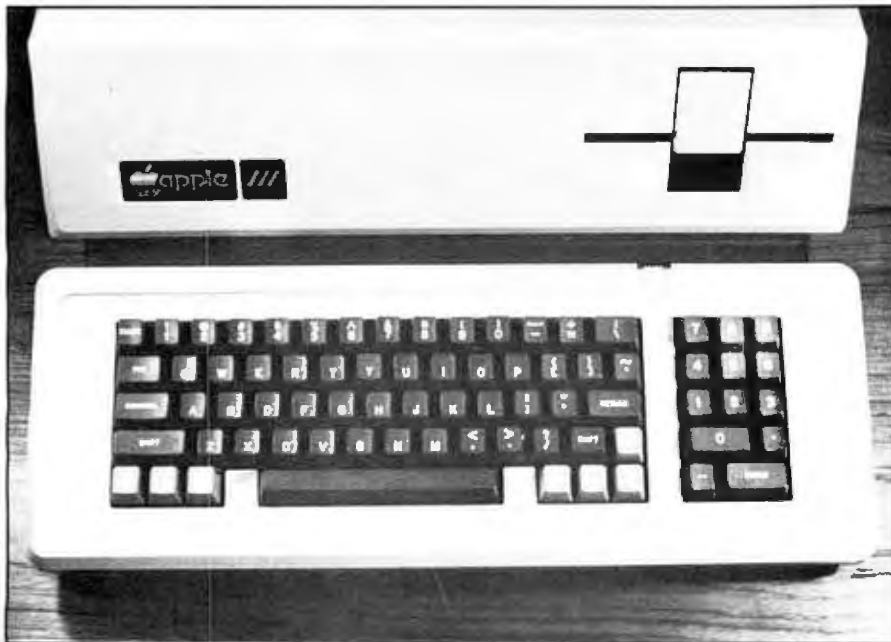
Photo 5: The Apple III keyboard. Although it looks separate, it is actually part of the Apple III main enclosure.
