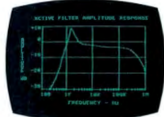
One example of a user-defined co-resident BASIC program: in this case designed to plot an amplitude response curve for an active filter.
