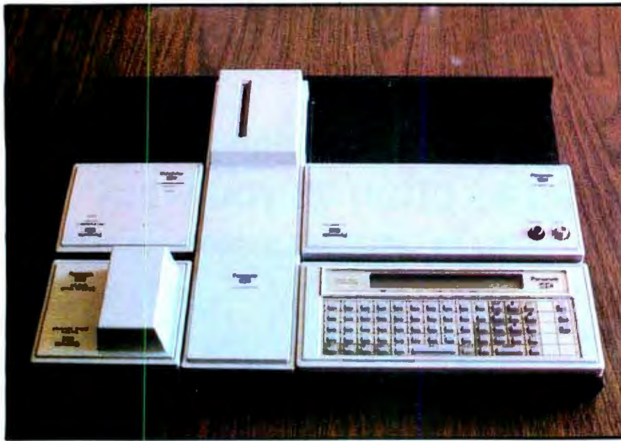
Photo 1: The Panasonic Hand-Held Computer (HHC) along with some of the available accessories. The HHC is in the lower right. Clockwise, the accessories are the I/O driver, the RS-232C port, the additional 8K-byte RAM module, and the video/television adapter.
