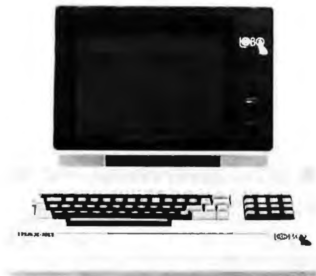
Photo 1: The Max-80 from Lobo Drives International is a 64K-byte computer system offering both CP/M and LDOS. It costs about $1000.
