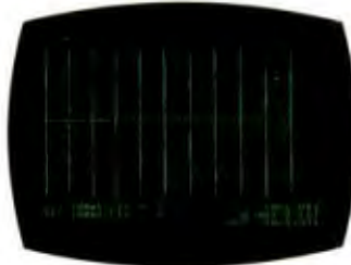
A reference waveform loaded from disk into Channel 2 for comparison with active signal on Channel 1.
