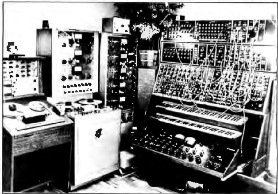
Photo 1: W. Carlos's electronic music production studio in 1968. There Carlos produced the recording "Switched-on Bach." At right is the modular Moog synthesizer. At left is a multitrack recorder, which was used to record the music one line at a time. Below the synthesizer is a 10-input mixer designed and built by Carlos.
