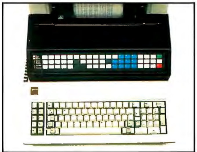
Photo 2: Close-up of the 57-key keypad (at top) and the 83-key keyboard on the IBM 9000.
