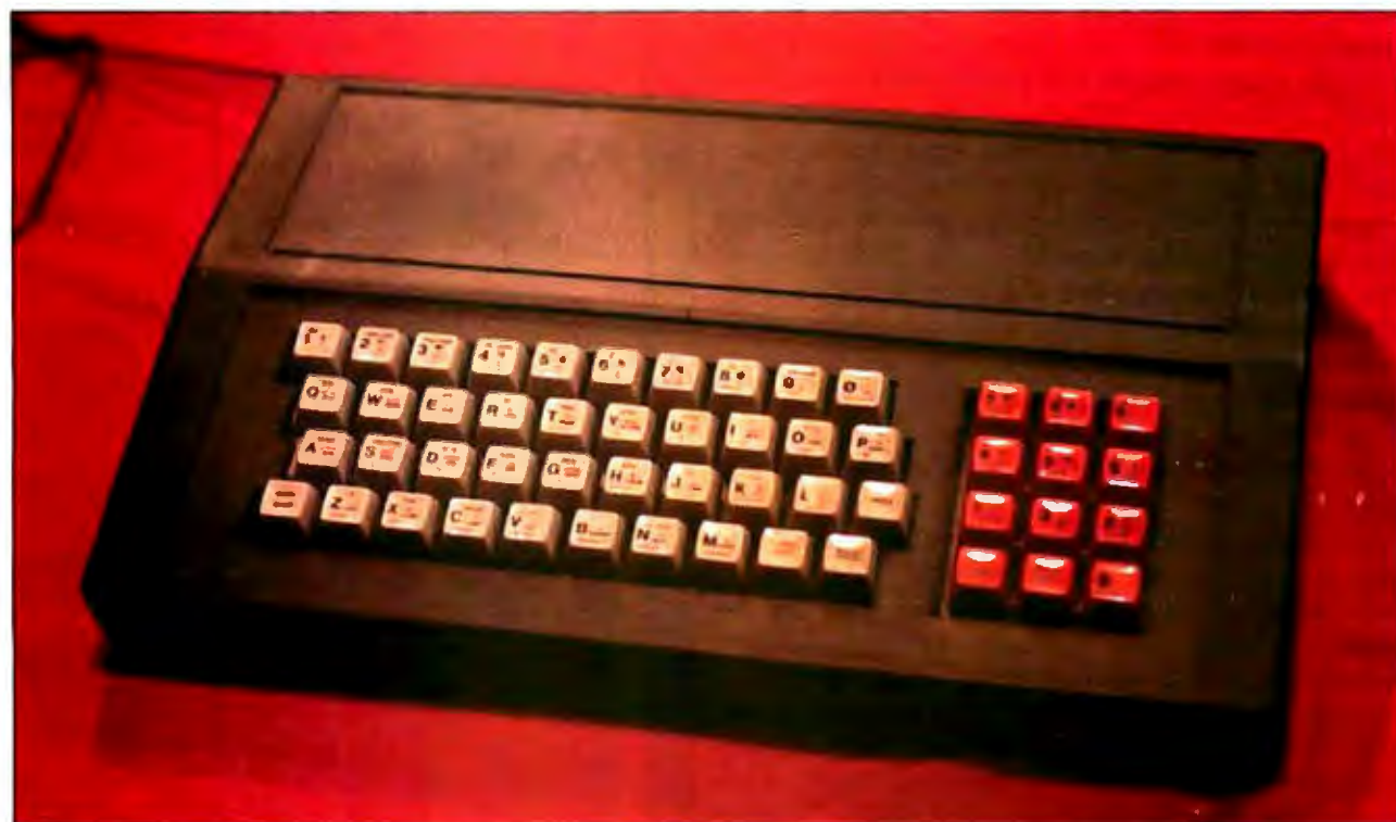
The Sinclair machines may be the most popular in Britain, but that doesn't mean that people like their keyboards—a brisk market exists for add-on keyboards and enclosures for Sinclair machines. This one, from DK'tronics, includes a full-size keyboard with keypad and an enclosure large enough to fit the computer board and other Sinclair peripherals. Its £45 price tag (almost as much as the £50 ZX81 computer) indicates the amount of interest in such products.
