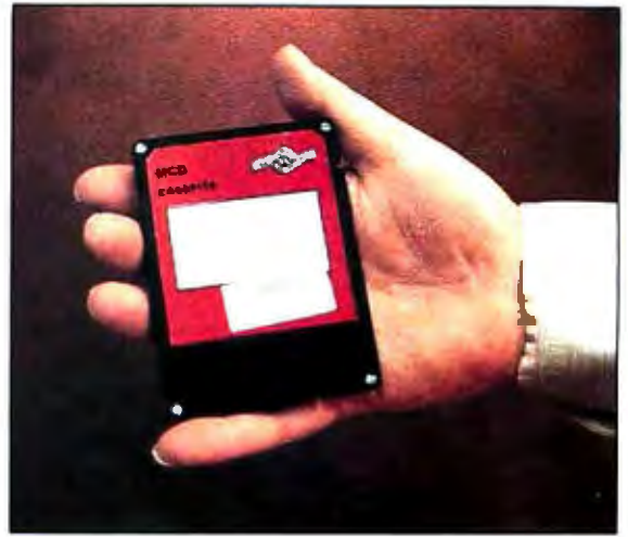
Here's a 3-inch disk pack for the Grundy Newbrain AD computer. The Newbrain disk-drive module houses two 3-inch disk drives in a small unit the size of the computer itself—in fact, the disk-drive module is meant to fit unobtrusively under the computer.
