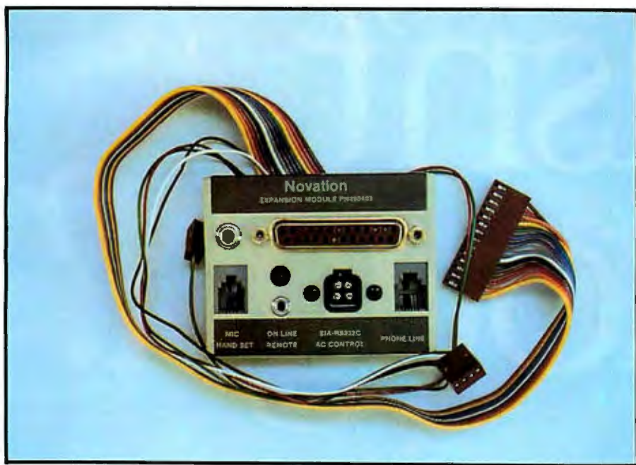
Photo 2: The Expansion Module contains sockets for a modular telephone line and handset, an RS-232C connector, a BSR X-10 controller, and a tape recorder. Also present is an LED to indicate an "off-hook" condition. The module mounts on the back of the Apple with double-sided tape and connects to the Apple-Cat II via the three cables shown here (the single pair for the phone line, the double pair for the handset, and the ribbon for the rest).
