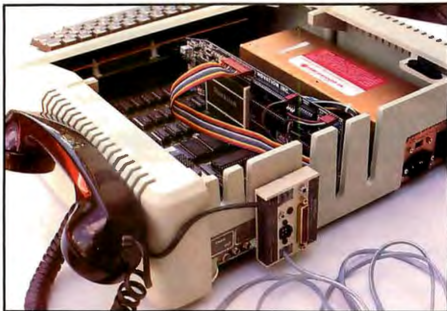
Photo 3: The Apple-Cat II and Expansion Module installed. Using the Expansion Module reduces cable clutter. The author has turned the unit sideways to permit full use of the adjacent slot on the back of the Apple.
