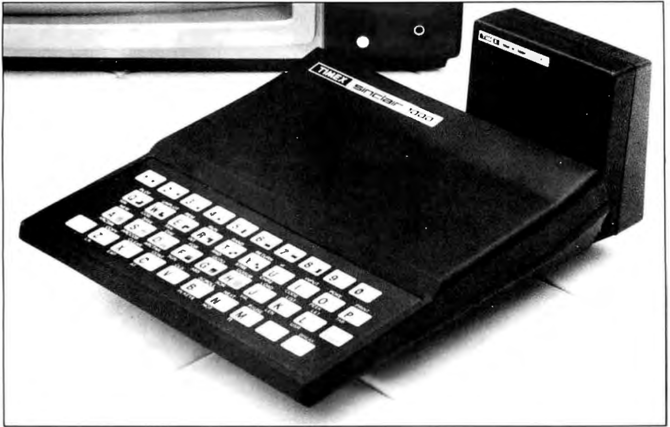
Photo 1: The Timex/Sinclair 1000 computer with the optional 16K-byte RAM pack, which attaches to a connector on the right rear of the computer. The basic unit powers the RAM pack. (Photo courtesy of Timex Computer Corporation.)
