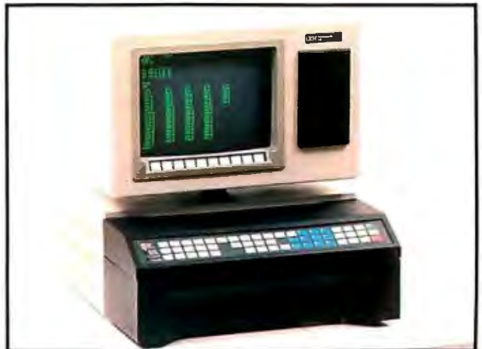
Photo 4: The stripped-down version of the IBM 9000, with CRT display, 57-key keypad, processor board, and chassis, retails for $5695.
