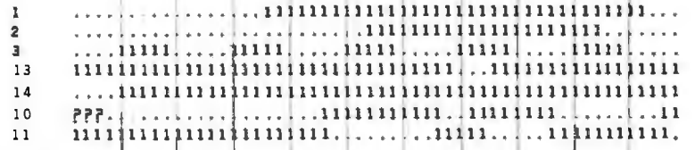
Figure 3: Simulation of the logic of a JK flip-flop. The design uses simple NAND and inverter gates and is presented to the simulator in the same way as in figure 1. The success of this model demonstrates the simulator's accuracy with sequential systems. (Cross-coupled gates used as latches present no problem.)
