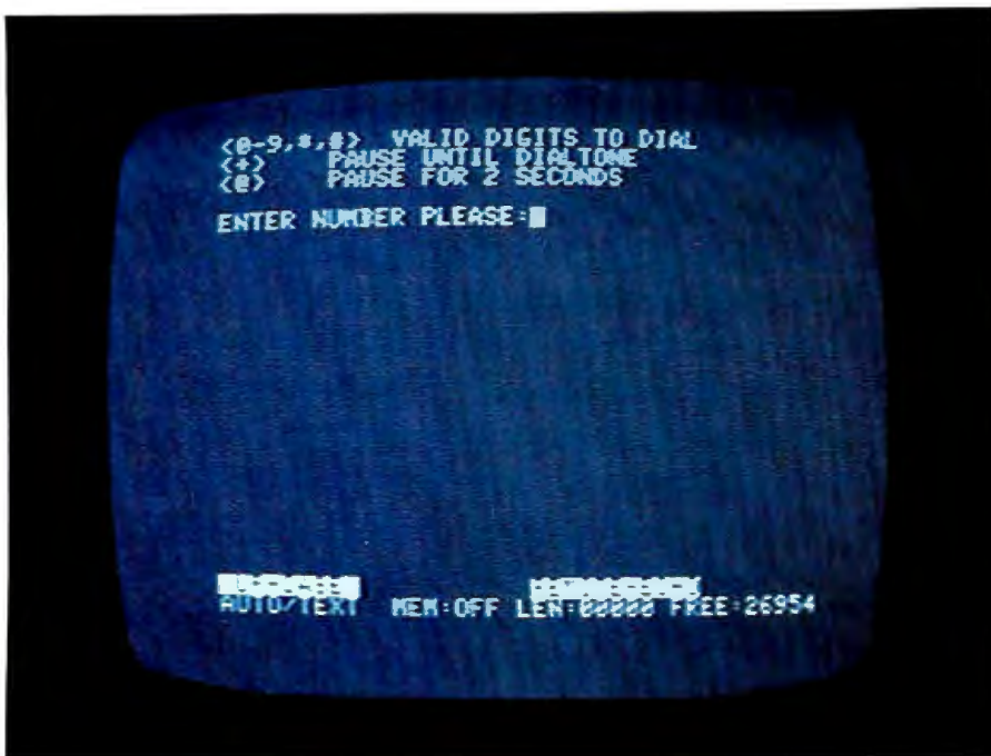
Photo 6: Selecting D from the previous screen (photo 5) gives this entry screen for phone numbers. Note that the options include pauses and waiting periods for a second dial tone. Since the Apple-Cat II can dial using either tone or pulse dialing, it can be used with private branch exchanges (PBX) or long-distance services that require tones, such as MCI. Most other modems do not function in both dialing modes.
