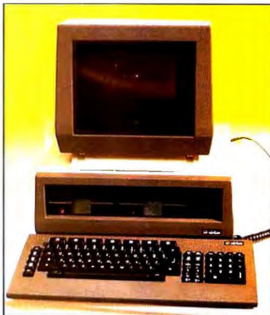
The ACT Sirius 1, as popular in Britain as the IBM Personal Computer is in the United States, is said to be the Victor 16-bit microcomputer in a different housing. An entire section of the show was devoted to ACT and third-party hardware and software vendors.
