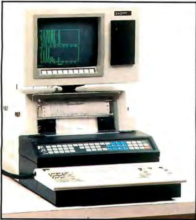
Photo 1: The new IBM 9000 Instrumentation Computer, manufactured by IBM's instrumentation division in Danbury, Connecticut. The machine uses the Motorola 68000 processor and includes (in this implementation) a 12-inch CRT display, a 57-key keypad with user-definable keys, an 83-key keyboard, four-color printer/plotter, custom IBM multitasking operating system, five I/O ports, disk controller for up to four 5¼-inch or 8-inch floppy-disk drives or hard disks, Versabus interface, and room for up to 5 megabytes of RAM onboard. The implementation shown in the photo costs close to $10,000.
