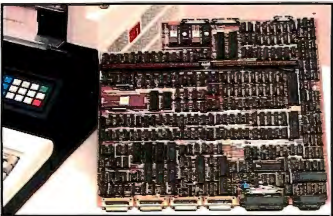
Photo 3: The IBM 9000 seven-layer planar processor board, showing the remarkably dense population of ICs and VLSIs. This state-of-the-art board has over 1600 test points and could not have been manufactured just over a year ago because of the density of the components. By plugging in an optional expansion board, up to five Versabus (a 32-bit bus standard developed by Motorola) cards can be plugged into the main board.
