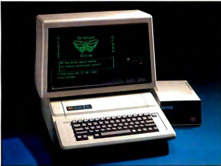
Photo 1: An Apple IIe system made up of the Apple Monitor III, the Apple IIe computer, and a Disk II 5¼-inch floppy-disk drive.
