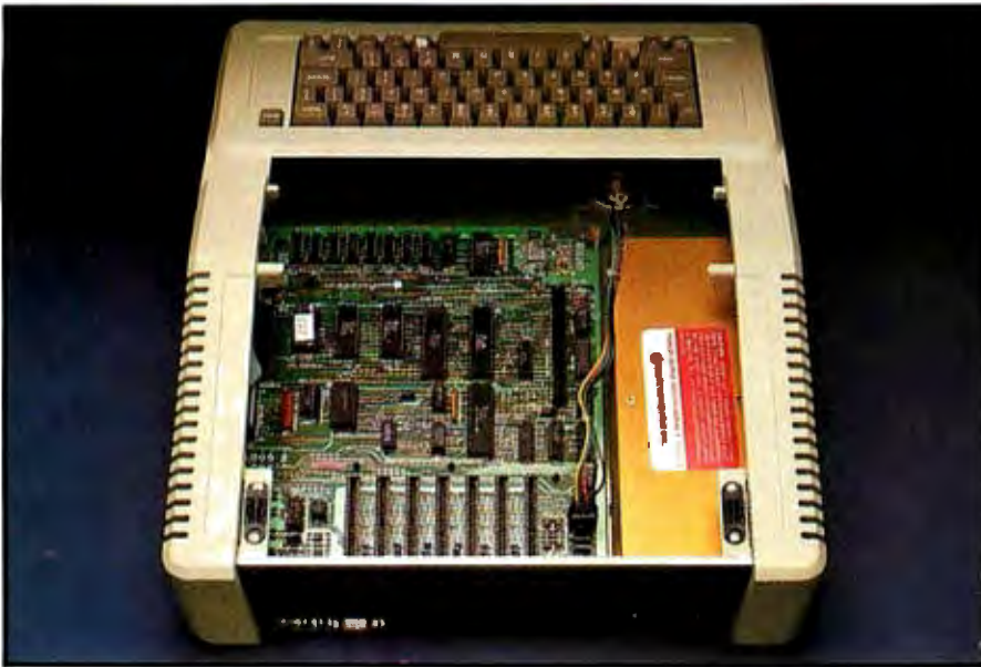
Photo 8: The Apple IIe main circuit board. The 31 ICs on this board replace the 120 ICs found in a standard Apple II, including a memory card, 80-column card, and keyboard enhancer, as well as providing a number of new features not available in the Apple II.
