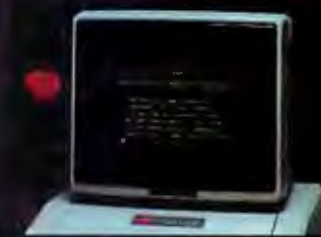
TAXAN 12" green phosphor monitor, model KG12N, features an 800 line resolution at center, 2000 character display
