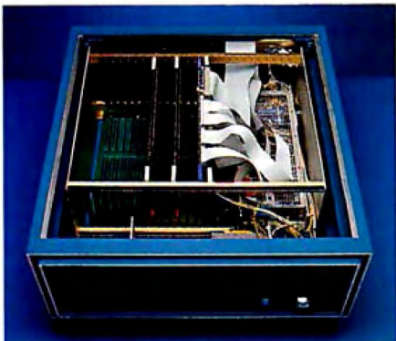
A LMC MC68000 system with 1.5 megabytes of error-correcting RAM.
