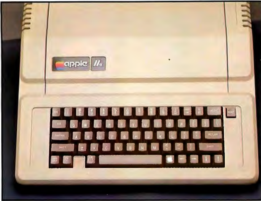
Photo 3: The Apple IIe keyboard. With uppercase and lowercase characters, N-key rollover, auto-repeat on all keys, and special-function keys, it provides a mix of functions found on both typewriter-style and computer keyboards. Unfortunately, the left-arrow key is inconveniently placed for its use as a backspace key while using BASIC. The special Open-Apple and Solid-Apple keys are used to invoke the self-test routines, simulate a power-up cold start, and may be read as paddle push buttons 0 and 1.
