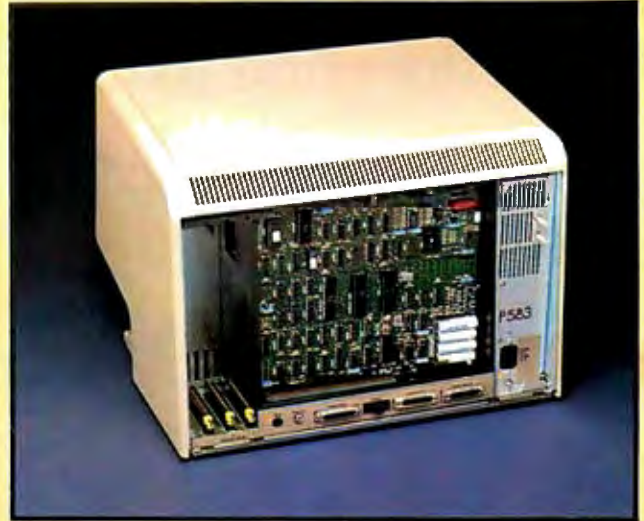
Inside the Lisa computer. Note the three connectors for expansion boards.
