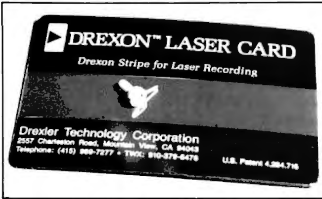
Photo 1: The Drexon Laser Card. This card can store 2 million bytes of data. The small object resting on the card's recording stripe is the semiconductor diode laser required to write data on the stripe. Either a diode laser or a photodetector array can read the data.
