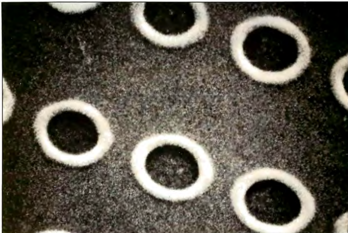
Photo 4: Recorded surface of a Philips Air-Sandwich optical disk. In this photo, taken by a scanning electron microscope, the 0.7-micron holes are magnified 40,000 times. The Philips disk has a capacity of 1.25 gigabytes per side. See figure 1 for a cross section of the Air-Sandwich disk.
