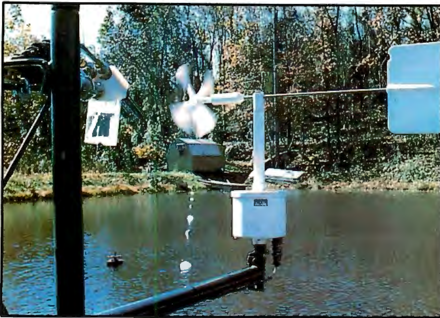
Photo 2: The buoys leading to shore support the wires that send analog signals to the cabin. The wire for transmitting the signals would have been the most expensive item of the whole installation if we had not bought it as military surplus.
