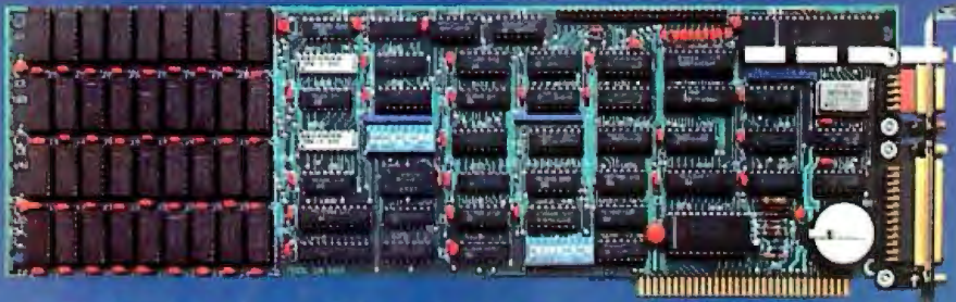
The IDEboard: Multifunction combination board. Memory up to 256KB. Options include serial interface, parallel interface (printer or SASI hard disk) and/or clock/calendar with battery backup. Prices range from $350 for 64KB with 1 option to $725 for 256KB with 3 options.
