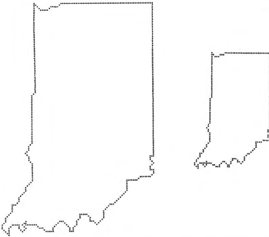
Figure 1: An example of an incremental-line drawing. The size can be changed simply by changing the values of the relative coordinates dx and dy . This drawing was done on a Diablo 630.
