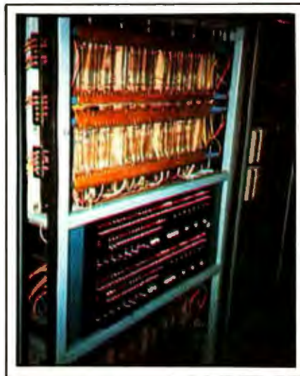
Photo 9: Front panel of a 32-bit minicomputer made at the Beijing Wire Communications Factory.
