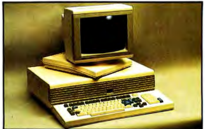
Photo 1: Fortune's 32:16 computer system. The processor unit and keyboard and video display for a single user are shown.
