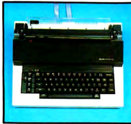
Photo 1: The Olivetti Praxis 30 electronic typewriter. The two cables in the rear connect to a parallel port on a microcomputer.
