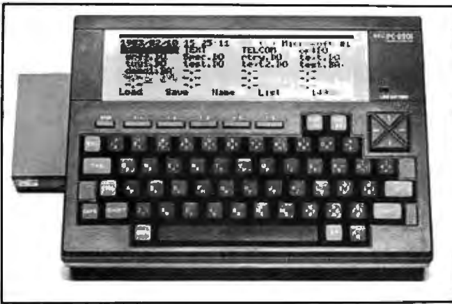
Photo 3: Screen display and keyboard layout of the PC-8201. Note that the keytop legends show both English characters and Japanese katakana characters. The special-function keys are labeled by the last line of the display.
