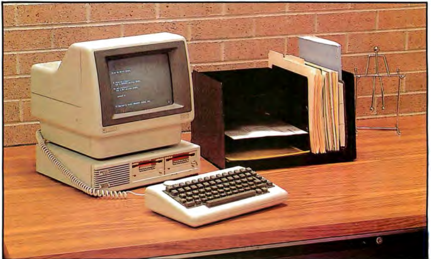
Photo 1: The Hewlett-Packard Series 200 Model 16 microcomputer (formerly the HP 9816). Even with the optional dual microfloppy-disk drive (3½-inch disks), the unit is extremely compact.
