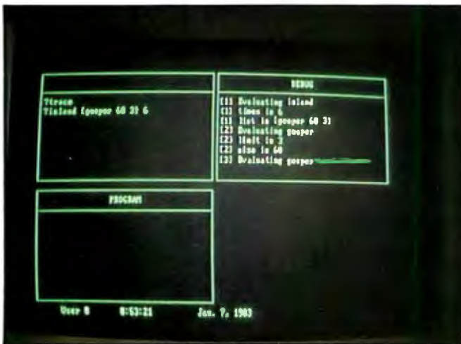
Photo 2: Multiple text windows in the debugging mode, with the trace function turned on. The upper left window is the Logo interpreter where you enter Logo commands. The debug window in the upper right displays information on the current program that is running. Output from the program and input that it requests are handled by the program window at the bottom. The trace function follows the program as it runs, showing the level at which a procedure is called, the name of the procedure, and the values of variables as they are defined. The island procedure being traced has two inputs: a list and a number. This shows up as level 1 in the debug window. The gosper subprocedure is called and begins to execute at level 2 with its variables, size and limit. The gosper subprocedure is recursive and calls a copy of itself that begins executing at level 3.
