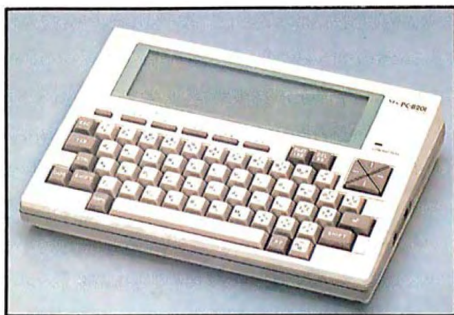
Photo 1: The NEC PC-8201 Portable Computer features a 40-character by 8-line LCD, software in ROM, and your choice of a red, white, or silver case.
