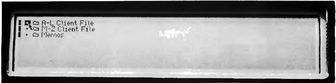
Photo 3: After the file drawer is opened, the screen displays the three file folders in the drawer. Each folder's name is preceded by a bar that indicates one level of nesting within the drawer, by a + sign that indicates the folder is closed, and by the symbol for a file folder. The + sign preceding the folder "A-L Client File" is highlighted because the pointer is on it. If you touch the pad now, the operating system will open the file folder and change the + sign to the open box that symbolizes an open folder.
