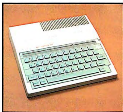
Photo 1: The Texas Instruments Basic Computer 99/2 is designed to compete directly with low-priced computers such as the Timex/Sinclair 1000. BASIC programs written on the 99/2 can run on the TI-99/4A, but the reverse is not true.
