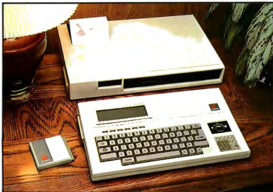
Photo 1: The C8/16 computer system from Sunrise Systems. The KP-C8 keyboard processor in the foreground with a 40-character by 6-line LCD is a prototype with six function keys instead of 10. The microcassette tape recorder is on the right side of the unit, above the speaker grill. The ROM pack on the left plugs into the side of the keyboard by the display. The FP-8/16 flat pack in the rear has two half-height 5¼-inch disk drives and a P-4/4 color graphics printer.
