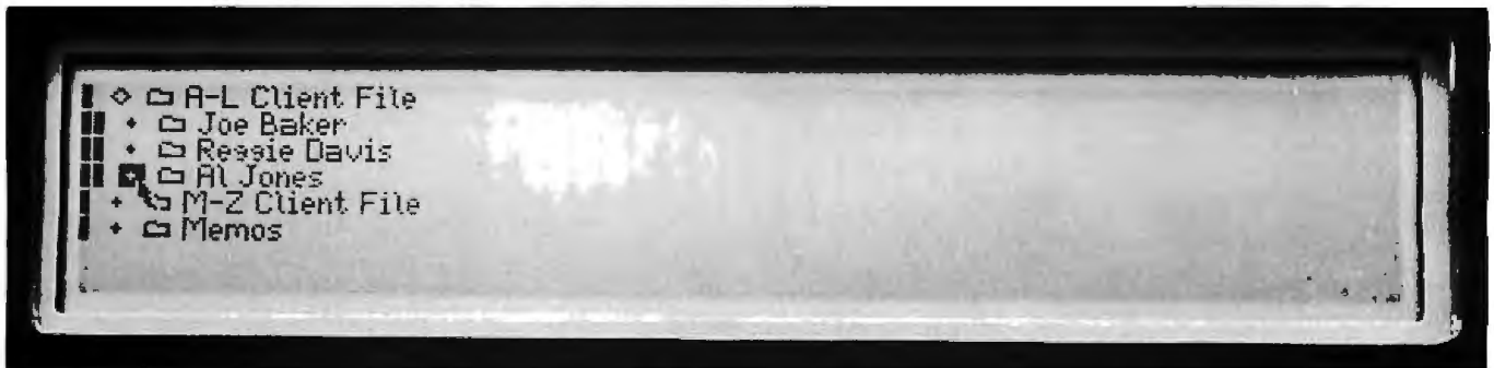
Photo 4: The A-L Client File is now open, and three files are shown inside it. Each of these three files is preceded by two bars, which indicate the level of nesting with the file drawer, and by the + sign that indicates a closed file. The operating system will open the Al Jones file, now highlighted, if you tap the touch pad.
