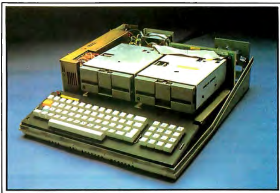
Photo 3: The M20 with its cover removed. Note the modular construction.
