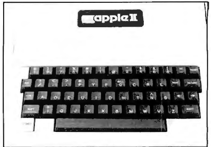
Photo 2: After gently prying the key caps off and rearranging them, you have the Dvorak simplified keyboard. The arrangement of the numerals shown here is the classic Dvorak arrangement. The recently approved American National Standards Institute Dvorak-layout keyboard standard (X4.22-1983) specifies that the numerals be in ascending order, as in the common QWERTY arrangement.
