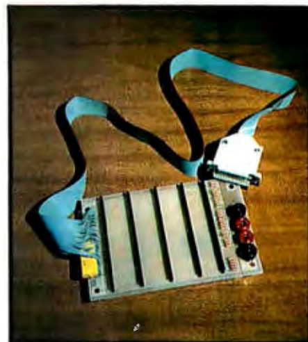
Photo 5: The new port-bus assembly, fitted with female 0.1-inch bus connectors and 10-kilohm termination resistors. Insert circuit boards beginning with the connector farthest from the cable end. The separate power supply is not shown.
