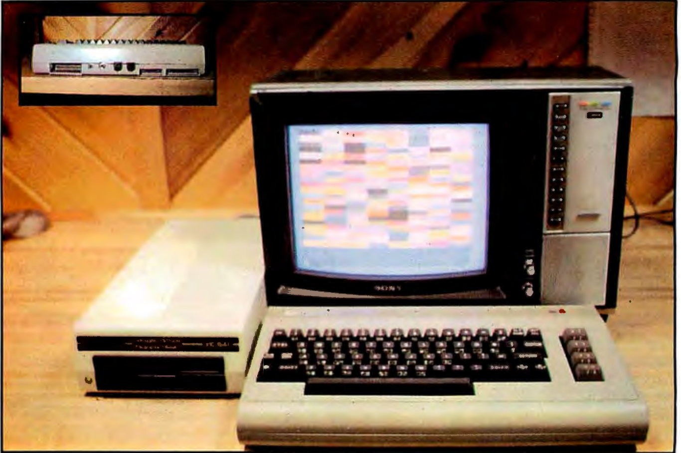
Photo 1: The Commodore 64 and 1541 disk drive. Inset shows rear view of the 64. From left to right, the cartridge slot for game or program cartridges; channel selector and TV output connector; the direct audio and video connector; serial port for disk drives or a printer; cassette interface; and the user port for peripherals such as the VICmodem.
