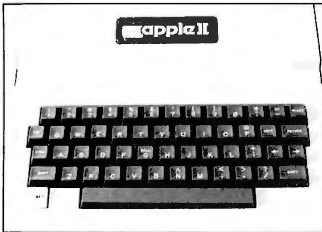
Photo 1: The standard Apple II keyboard with the QWERTY key arrangement. Note that many frequently used keys (E, T, R, etc.) are not on the row where the fingers normally rest.
