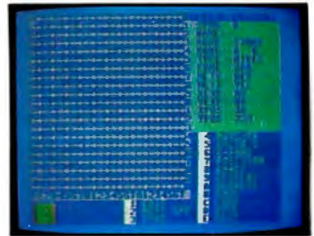
Photo 3: Sprite editor display. Defining a sprite is just a matter of turning dots on or off. The actual size of the sprite is shown in the lower left corner.
