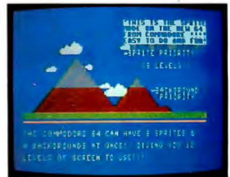
Photo 4: Sprite Priorities. In this still shot from an animated sequence, some of the sprites appear to pass in front of or behind the mountain. All of the sprites on the screen have different priorities to give the effect in three dimensions.
