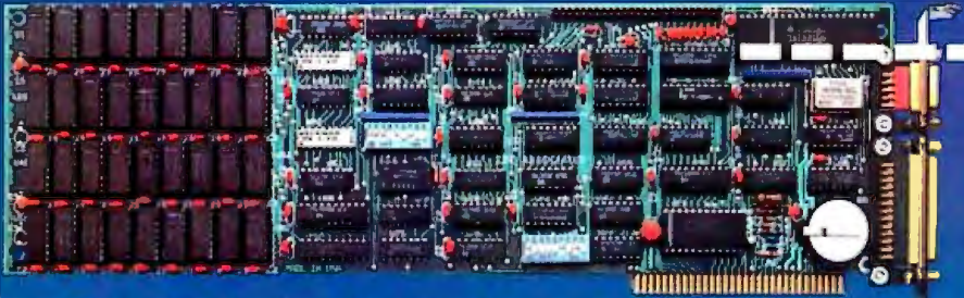
The IDEBoard: Multifunction combination board. Memory up to 265KB. Options include serial interface, parallel interface (printer or SASI hard disk) and/or clock/calendar with battery backup. Prices range from $320 for 64KB with 1 option to $695 for 256KB with 3 options. All prices include RAMFLOPPY disk emulation software.
