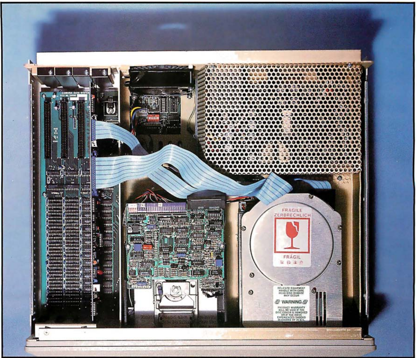
Photo 8: Inside the Corona. A Seagate hard-disk drive is on the lower right and the expansion slots are on the left. One of the slots is taken up by the hard-disk controller. The power supply is on the upper right.
