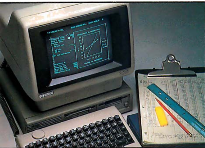
Photo 3: The Model 16, shown here with a dual 3½-inch floppy-disk drive, takes up a small amount of desk space. Note the "knob," a one-dimensional track ball, on the upper-left corner of the keyboard.
