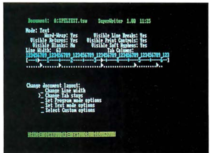
Photo 5: By issuing the Escape G extended command, you can get to a menu for changing the global document settings. Two major groups of settings are available, one mode for editing text (used in these examples) and another for editing program code. You can mix and match the settings to your taste.
