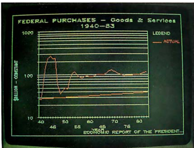
Photo 6: Performing regression with Chartmaster's logarithmic scale results in an error in the regression line.
