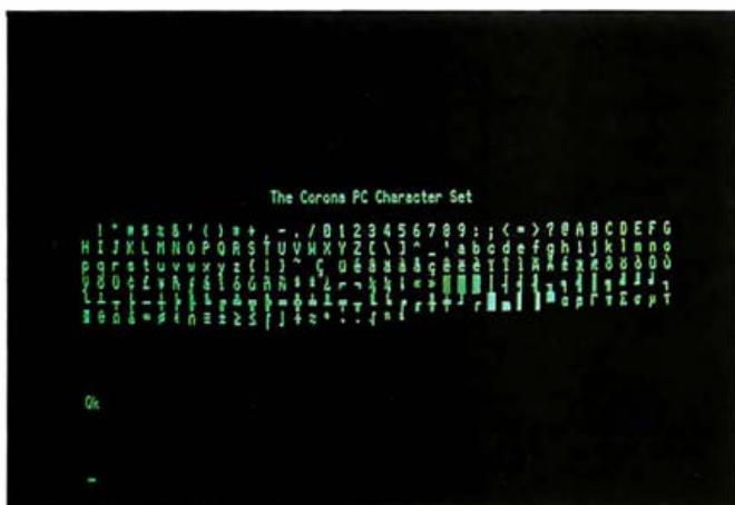
Photo 3: The character set of the Corona PC. The Corona has the same variety of characters as the IBM PC.
