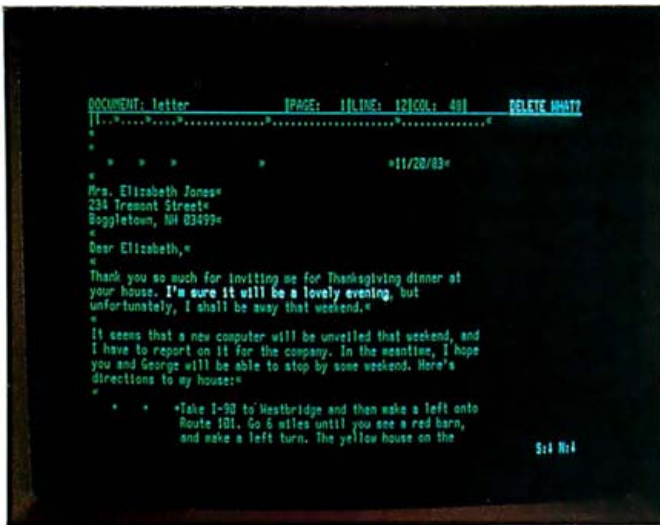
Photo 9: An example of a document being edited by the Multimate word processor. Note the format line at the top of the screen and the non-ASCII characters to indicate tab stops, carriage returns, and indents. Also note the highlighted area that is to be deleted.
