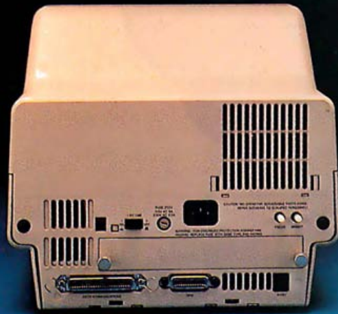
Photo 2: The rear panel of the Model 16. Note the HP-IB connector at the center of the bottom part of the panel and the serial connector in the lower-left corner.
