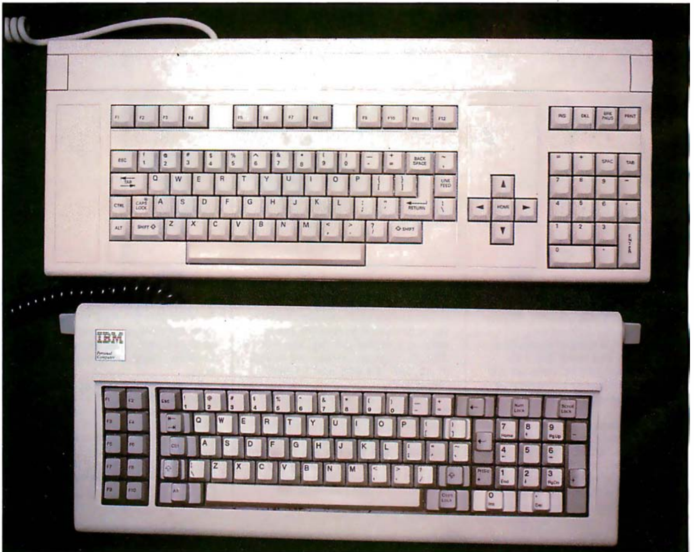
Photo 1: The TI PC (top) and IBM PC (bottom) keyboards. Notice the larger number of keys on the TI PC keyboard (photo by Randy Bullard).
