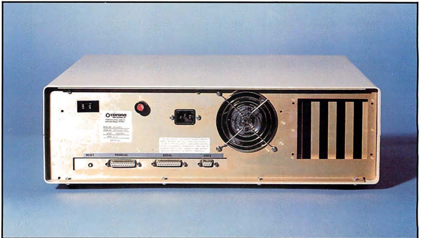
Photo 7: The back panel of the Corona. Note the Reset switch on the left, the parallel-printer port, the serial port, the video-display port, and the openings for the expansion cards.
