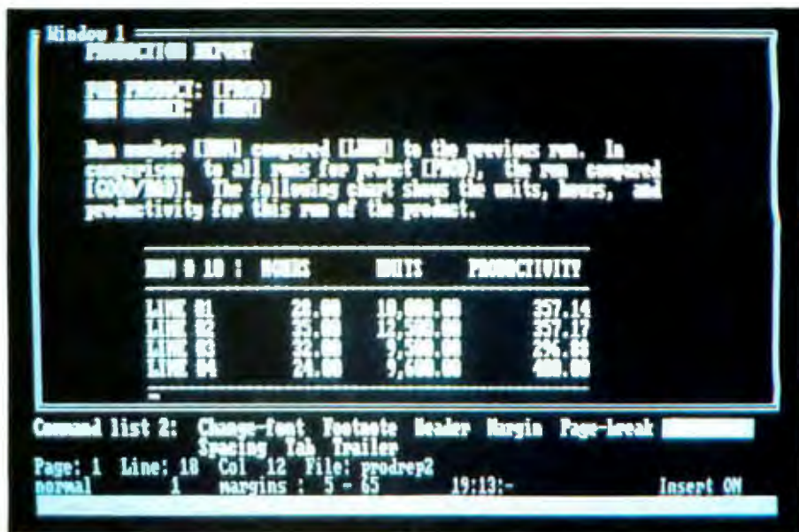
Photo 3: An example of merge-print word processing; a portion of the production spreadsheet has been inserted within the text of this production report.
