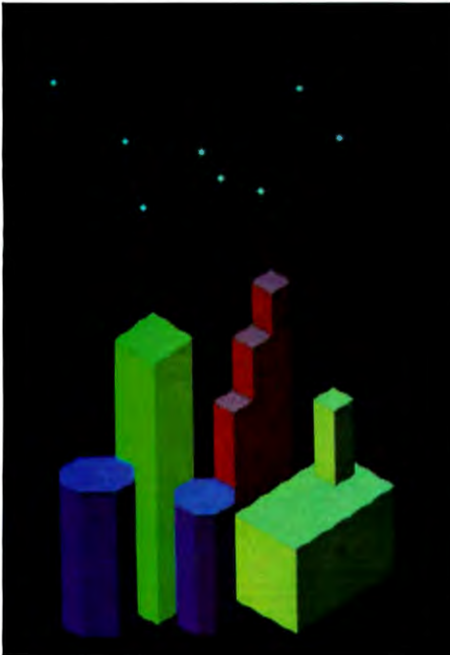
Photo 3: Low-resolution graphics are not a serious limitation for fine-art applications because of the double-screen mode and shading capabilities. These simulated three-dimensional structures are nothing more than juxtaposed parallelograms and other shapes with varying shades, drawn on alternate screens. Diagonal edges are formed where complementary right triangles on alternate screens share a diagonal series of pixels.
