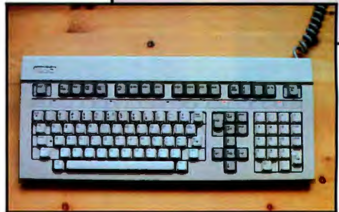
Photo 2: The Wang's sculptured keyboard contains 101 sculptured keys, including 16 programmable function keys. Note the indicator lights, which can signal problems even when the display is not working.
