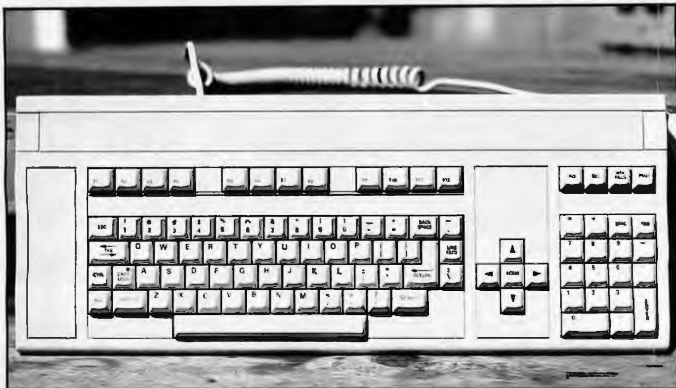
Photo 4: The low-profile keyboard unit has a more familiar layout than IBM's. Indentations on the J and F keys help you find the home row. The tabs on each side of the unit near the top control a flap on the back that elevates the keyboard.
