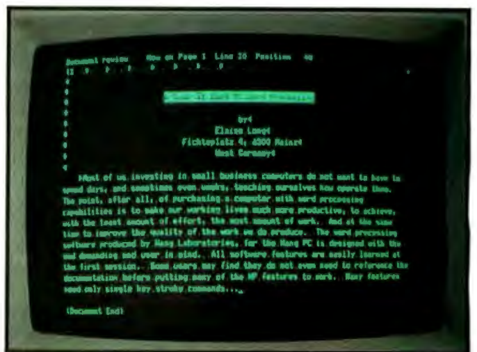
Photo 5: An example of text produced by Wang's word-processing program. The summary line and format line are at the top. Spaces are indicated with half-intensity periods.
