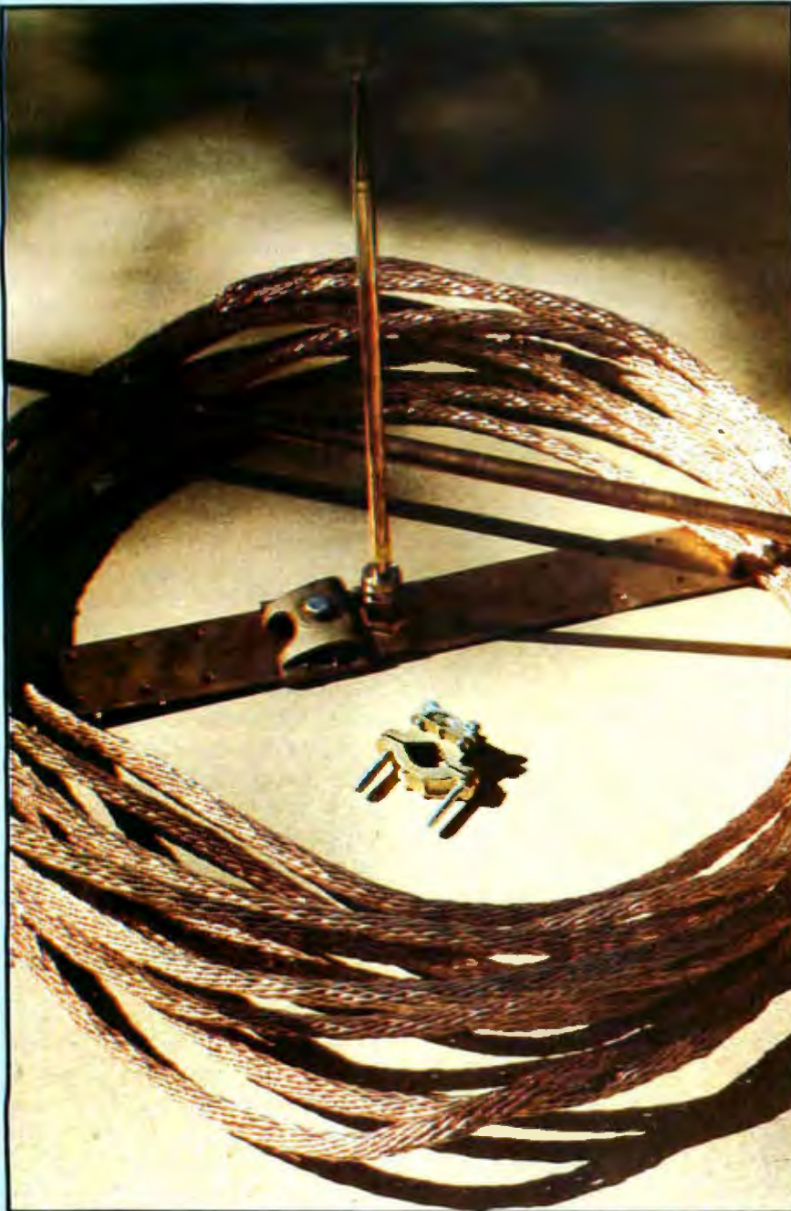
The important element in lightning protection is the lightning rod, a pointed shaft of copper to which a half-inch copper cable is fastened. The cable runs down the side of the building, where it is clamped to an 8½-foot copper-plated steel rod driven into the earth. The rod system pictured here costs $150.
