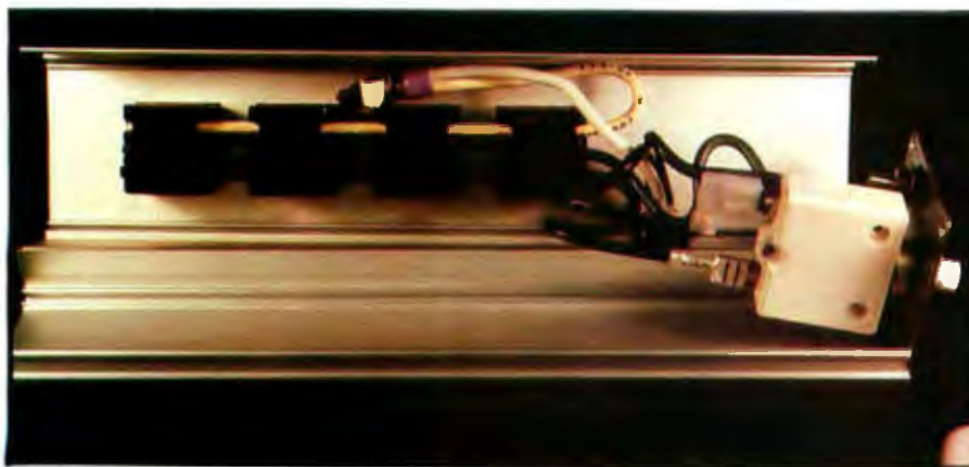
Photo 3: Open the strip case, exposing the four receptacles and the white circuit-breaker block. The three wires conducting power run the length of the strip: black is the hot side, white is the neutral return, and the green wire is earth ground.
