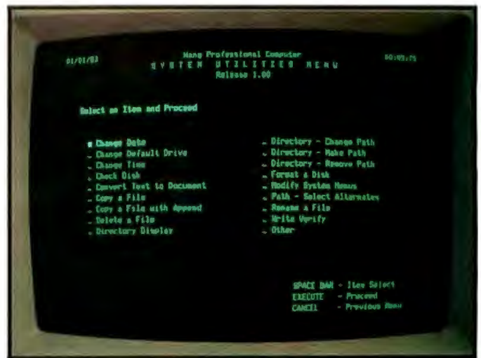
Photo 3: The menu of utility programs included in Wang's version of the MS-DOS operating system.
