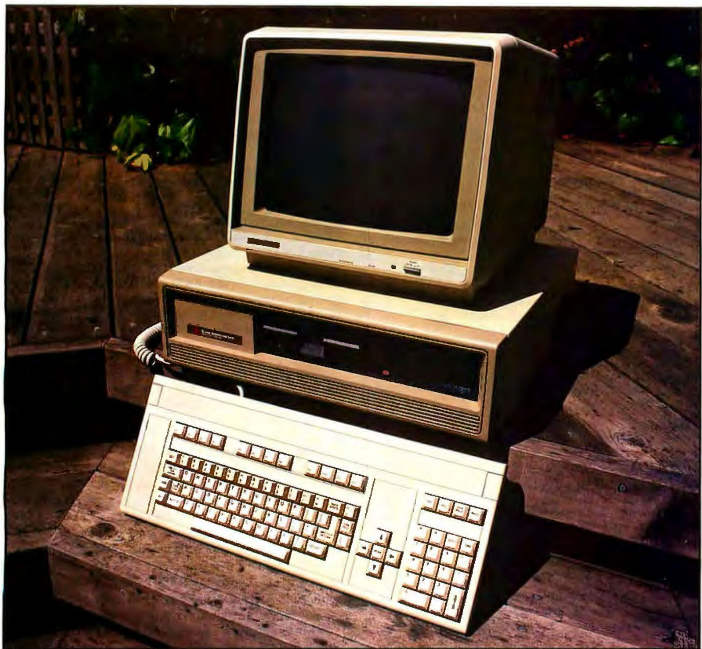
Photo 1: The TI Professional Computer is made up of the system unit, the display, and the keyboard. This computer also has a 5-megabyte Winchester-disk drive installed to the right of the 320K-byte floppy-disk drive.
