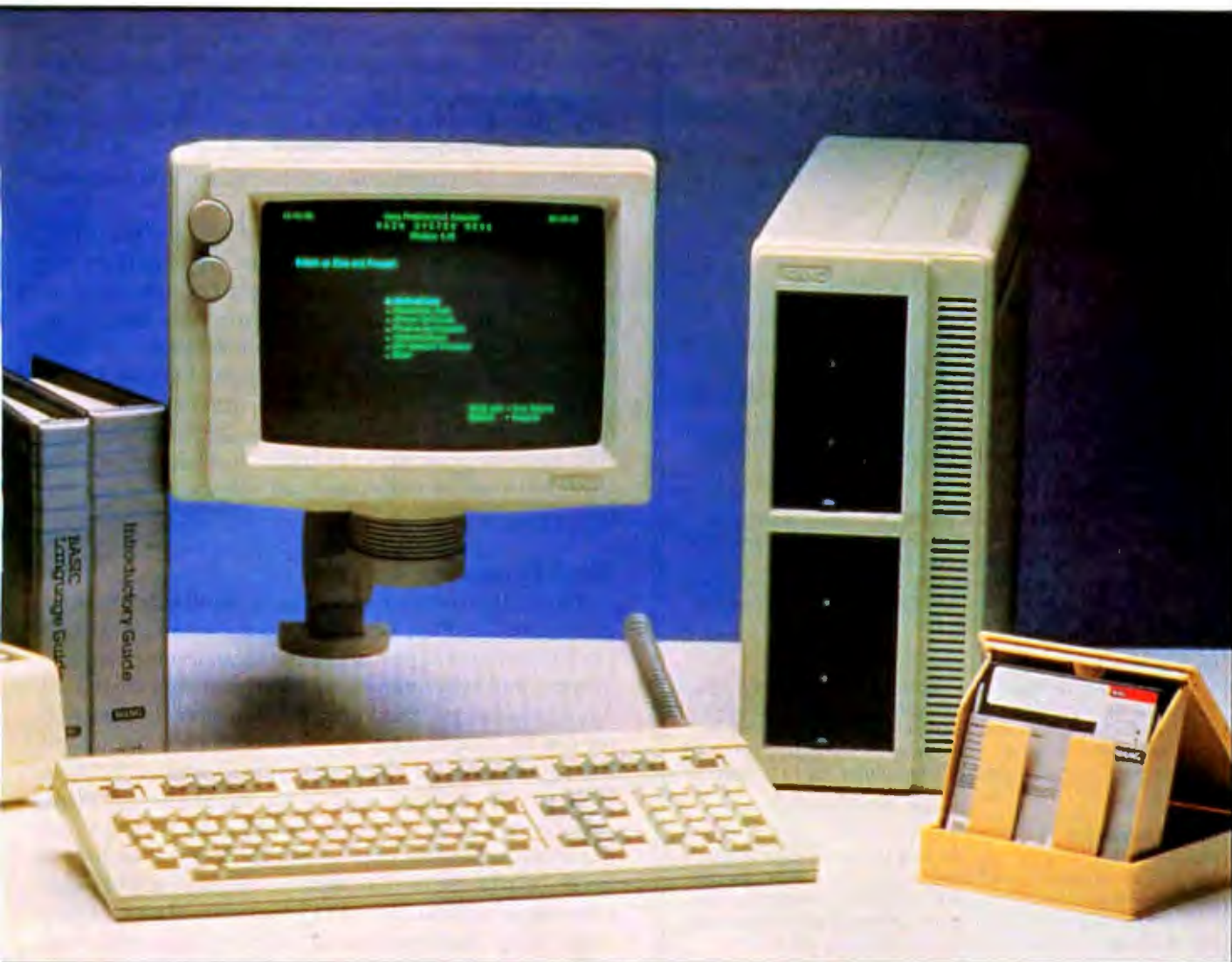
Photo 1: In this configuration, the Wang Professional Computer rests on an optional stand (the PC Arm, $150). A daisy-wheel printer (Model PC-PM010, approximately $600) is on the left. Interestingly, the system unit, which houses two floppy-disk drives, can be placed either horizontally or vertically on a desk or it can be clamped to the side of a desk with the PC Clamp (which comes with the PC Arm).
