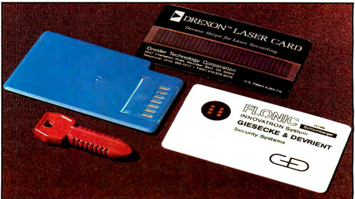
Photo 1: Four memory cards incorporated into different carrier packages. The bottom three cards are active devices, containing embedded microcomputers. Note the metal contact points on their surfaces (or, the "key," the contacts are between the ridges). The top card is a passive device that uses an optical stripe for laser recording and playback.
