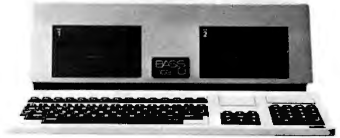
Photo 1: The Basis ("Bah-zis") 108 is a microcomputer, configured like an Apple II, with Z80 and 6502 microprocessors and 128K bytes of RAM. The 108 comes with two Basis disk drives. The earlier model (shown here) has Micro-Sci drives. The keyboard provides all the features required of a business system.
