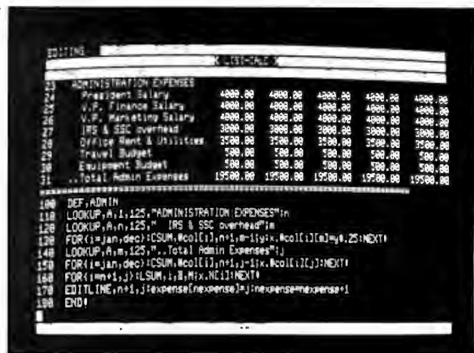
Photo 2: The spreadsheet shown with the program it automatically generates. Programs in the Laplace interpreter can generate spreadsheets, and use of the spreadsheet generates programs.
