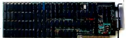
The PC640 Professional Color™ board delivers superior resolution at 640 × 480, and the simultaneous use of 16 out of 4096 colors.
