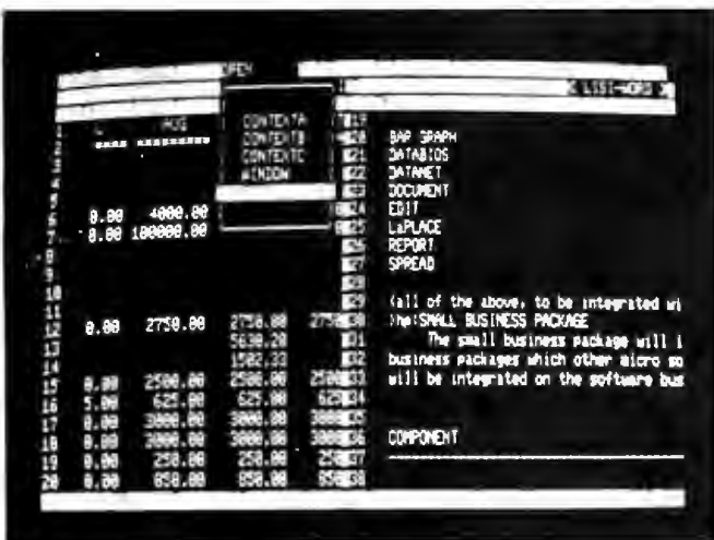
Photo 5: The spreadsheet and word processor in different windows. The user is preparing to copy the title "SMALL BUSINESS PACKAGE" from the text file at right directly into the spreadsheet at left. Large blocks of text can also be moved.
