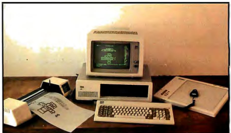
Photo 4: One example of a CAD system, an IBM PC with a Houston Instrument Hipad 11 by 11 digitizer and DMP-40 plotter.
