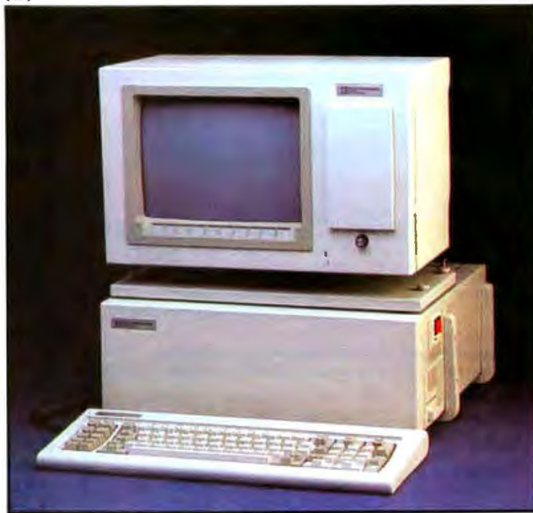
Photo 1: At left (1a) is a front view of a typically configured IBM CS-9000 with the built-in dot-matrix printer. The rectangular plate covers a mount for a single 5¼-inch floppy disk. Notice the paper tray under the keyboard. The handle below the video display connects to the mounting yoke (see text). Photo 1b shows a front view of the business configuration of the CS-9000. Note that the built-in printer and softkeys have been removed.
