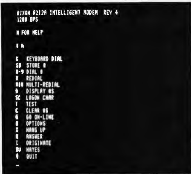
Photo 2: The help display generated by the R212A. Note the sign-on message at the top of the screen. The dollar sign is the modem's prompt character. Each of the commands shown is accessed by its one- or two-character mnemonic.
