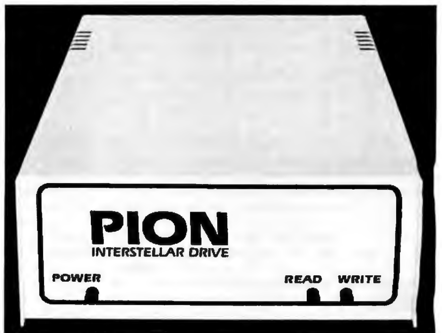
Photo 1: RAM disk emulators for the Apple. The units shown are, top to bottom, the Axlon Ramdisk 320, the Syntex 2202 Solid State Disk Emulator, and the Pion Interstellar Drive. Not shown is the Legend 128K DE Softdisk, which somewhat resembles the Syntex card.
