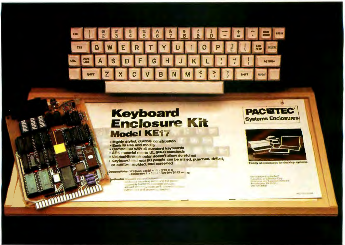
Photo 2: The Term-Mite ST can be connected to the stack-pole keyboard shown here, but the NS455A can be used more easily with an Oak full-travel membrane (FTM) keyboard from Oak Switch Systems Inc., POB 517, Crystal Lake, IL 60014. An enclosure from Pac Tec (Enterprise and Executive Aves., Philadelphia, PA 19153) enhances the terminal's appearance.
