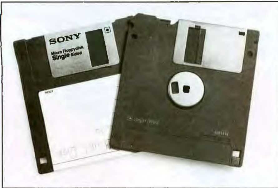
Photo 4: The Sony 3 1/2-inch disk is encased in a rigid plastic housing, and the oval window through which the magnetic medium is accessed is protected by a metal shutter that slides out of the way when the disk is inserted in the drive. These factors help protect the disk from casual use.
