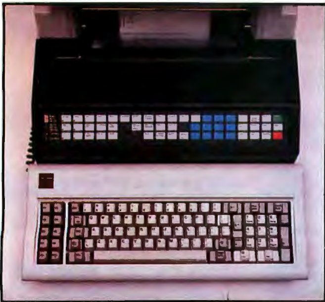
Photo 3: The CS-9000 keyboards. At the top, on the front of the main processor box, are the 57 programmable, pressure-sensitive keys.
