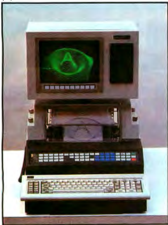
Photo 1: At left (1a) is a front view of a typically configured IBM CS-9000 with the built-in dot-matrix printer. The rectangular plate covers a mount for a single 5¼-inch floppy disk. Notice the paper tray under the keyboard. The handle below the video display connects to the mounting yoke (see text). Photo 1b shows a front view of the business configuration of the CS-9000. Note that the built-in printer and softkeys have been removed.
