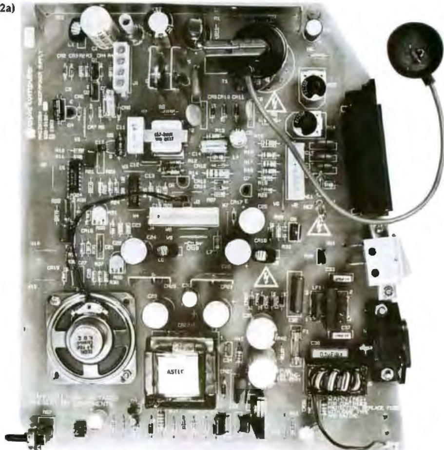
Photo 2: The Macintosh circuit boards. Photo 2a shows the analog board, while photo 2b shows the digital board. These two boards plus the video display, 3½-inch disk drive, and housing make up the main unit; only the keyboard and mouse are needed to make a complete Macintosh system.
