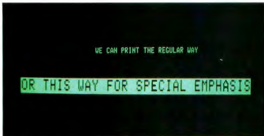
Photo 3: The Term-Mite can display several character attributes singly or in combination, such as reverse video (3a) and reverse, double width, double height (3b).
