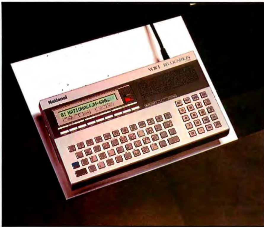
Photo 6: Matsushita ("National" in Japan, "Panasonic" in the U.S.) showed its new portable voice-recognition module, the JH-600. The unit can be used by itself to recall short memos related to spoken inputs or can be connected to other systems as a controller or data-entry device.
