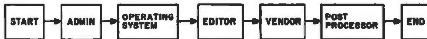
Figure 3: Layers of software between the user and graphical output. Lack of knowledge of software layers denies most users access to graphics.
