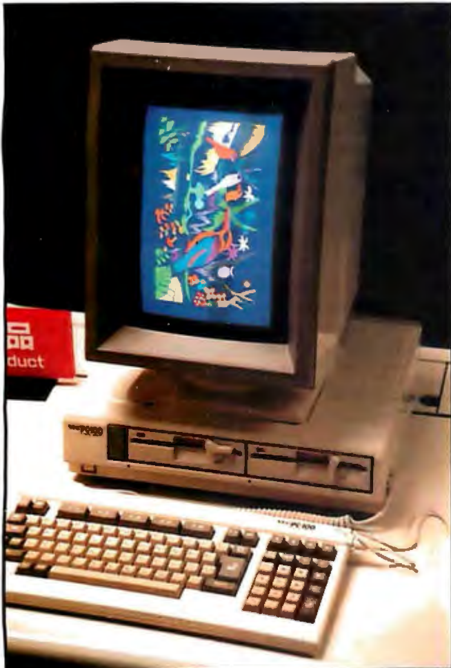
Photo 2: NEC's new PC-100 8086-based system with a color display. A monochrome display is also available. Both CRTs can be turned horizontally.
