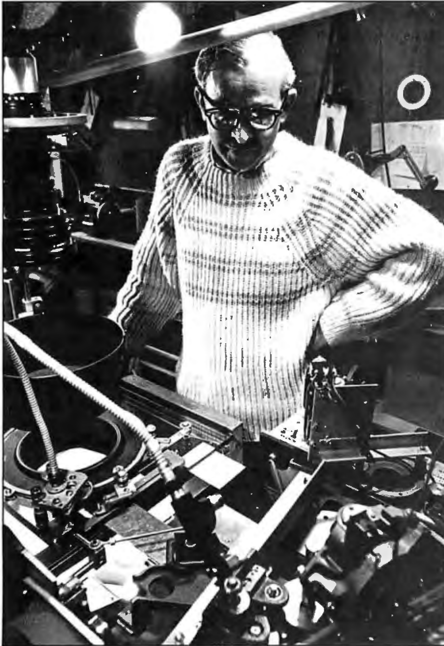
Photo 9: Pioneer computer animator John Whitney Sr. in 1959, operating one of the first computer-graphics engines, a mechanical analog computer built largely from surplus World War II anti-aircraft guidance hardware. The camera is in the upper left, aiming down through the apparatus that "paints" the film with light. (Photo by Charles Eames.)
