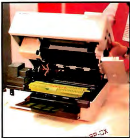
Photo 8: Canon's new low-cost laser printer is shown in 8a. The unit has many similarities to the company's line of personal cartridge copiers. Although Canon plans to sell only the mechanism (8b), a prototype of a complete printer was on display at the Data Show.
