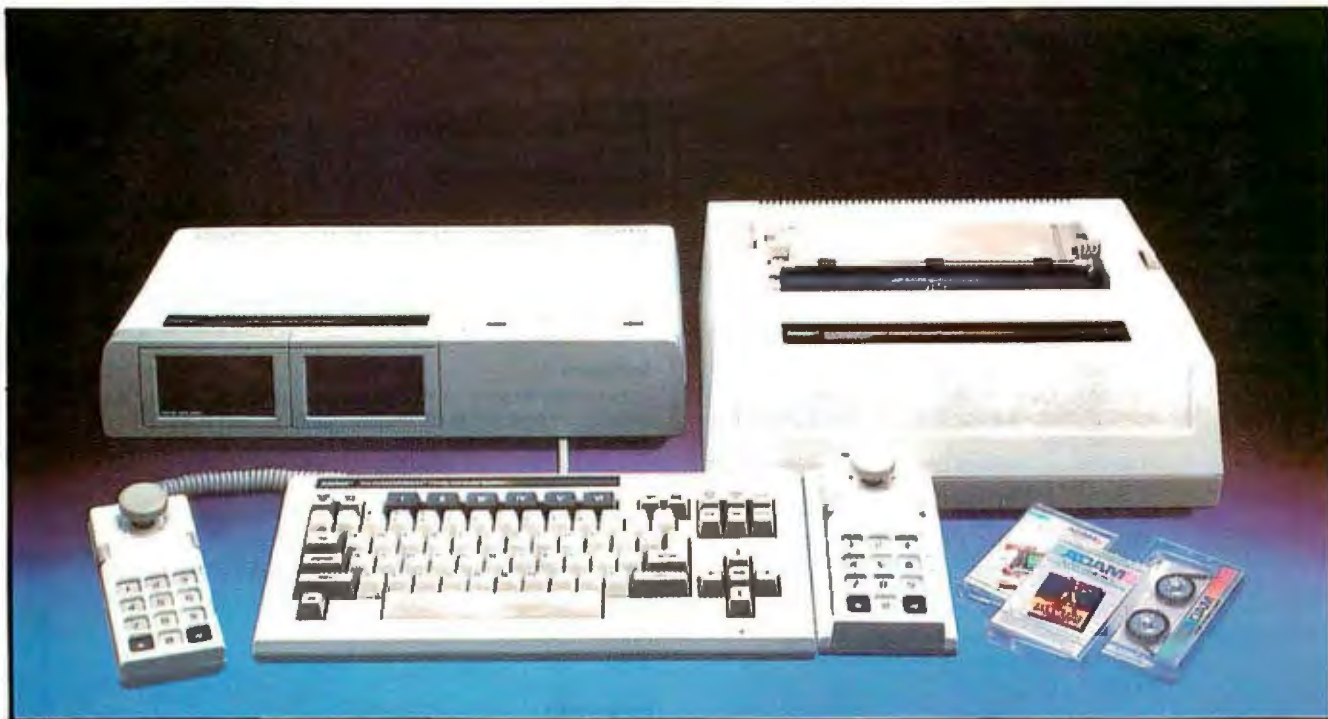
Photo 1: The Coleco Adam includes a tape drive, a printer, 64K bytes of RAM, a keyboard, a Colecovision game system, and two joysticks.
