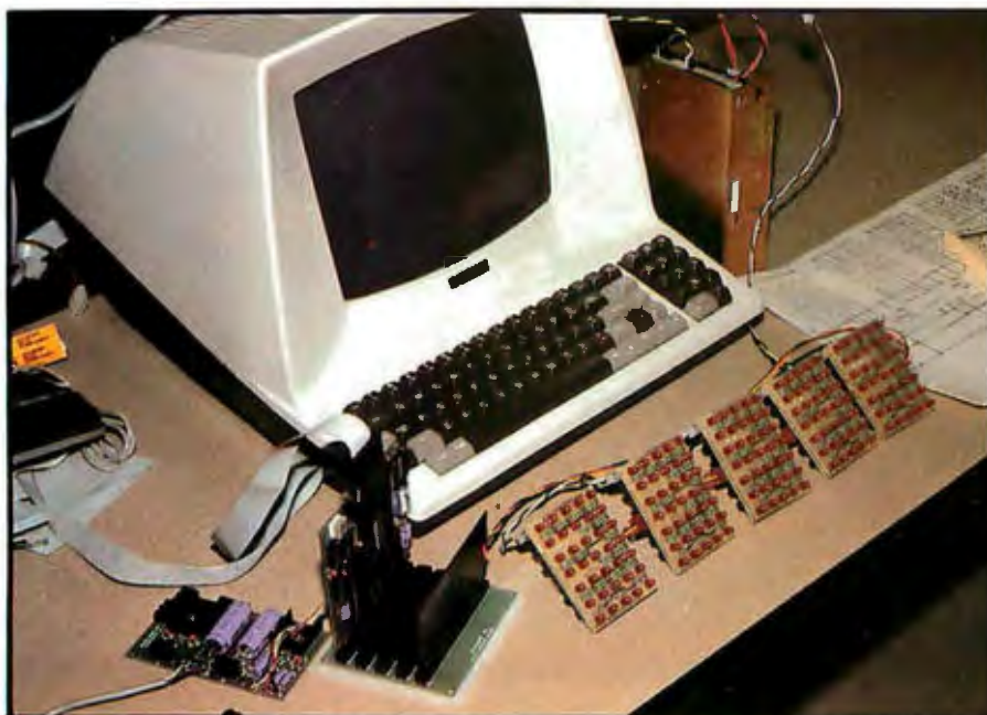
Photo 5: In my first attempt, several display segments were attached to the Z8 board; the message content of the display can be changed interactively from the video terminal.
