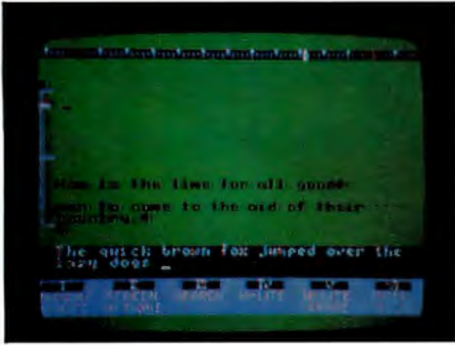
Photo 5: The Adam's word processor is built into the system's ROM chips. Although limited, the Smartwriter word processor should be adequate for home use.
