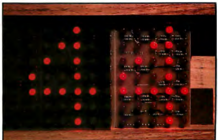
Photo 4: These examples of the numeral "4" were produced by the same bit pattern used in listing 1, but under the control of the Z8-BASIC System Controller. The red plastic filter over the left segment greatly improves the appearance of the display.
