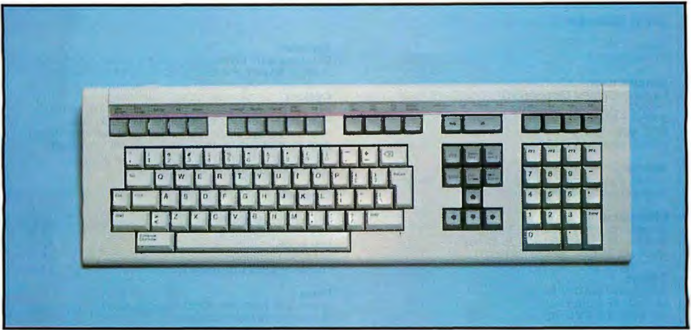
Photo 3: The Rainbow's 105-key keyboard. Label strips (along the top of the keyboard) may be changed. Note the division of keys into four groups: the standard typewriter keys, a set of editing keys (including cursor control), a numeric keypad, and, along the top, a row of special-function keys.
