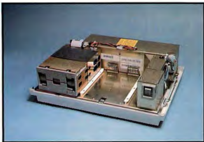
Photo 4: A look under the Rainbow's cover. The power supply is along the rear edge. The RX50 drive is on the right. The empty spot in the middle will accept another RX50 drive or a 5¼-inch 10-megabyte hard-disk drive.
