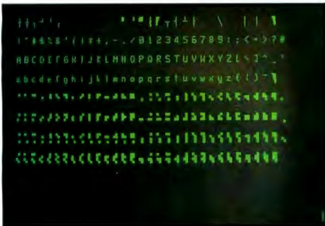
Photo 2: The complete character set of the Kaypro 10. The 10 includes a good collection of graphics characters.
