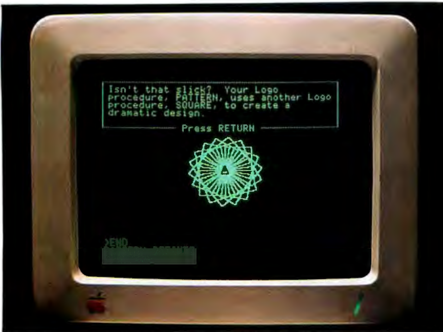
Photo 7: Part of the Apple Logo tutorial. Apple has limited the amount of printed documentation and increased the interactive on-line tutorials available with the IIc. The basic system comes with four disks of tutorials designed to offer 10 to 12 hours of instruction.
