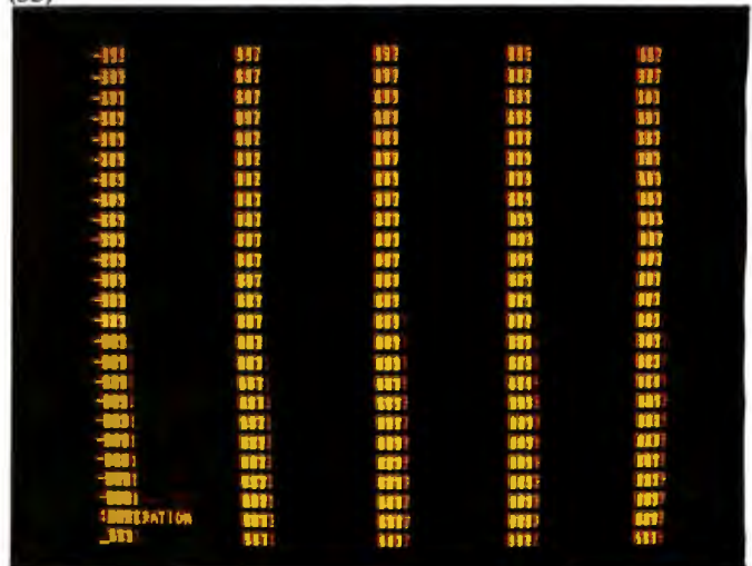
Photo 3: Execution-time visual comparison. (3a) Without Trump Card—a two-second exposure of the display while running the BASICA program in listing 1. The program has executed the PRINT statement and still is dimensioning the arrays. (3b) With Trump Card—the same two-second exposure of the program execution (with PRINT statement added) shows the arrays have been dimensioned and the prime numbers are being overprinted so fast that they blur.
