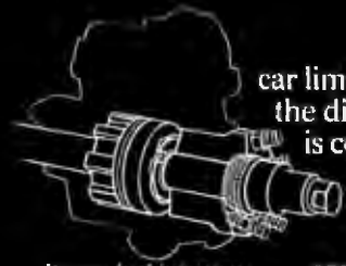
Rotary fuel injection pump precisely measures fuel for each cylinder.
