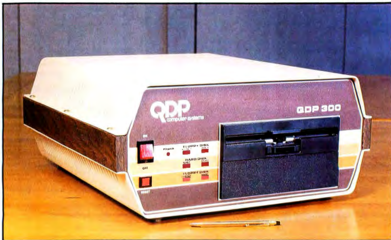
Photo 1: The QDP-300 with a 10-megabyte hard-disk drive and one 8-inch floppy-disk drive.
