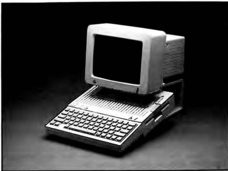
Photo 2: An optional 9-inch monochrome monitor is available for the IIc. When separated from the monitor, the system can be carried in a briefcase-size carrying case that includes room for the flat-panel display.
