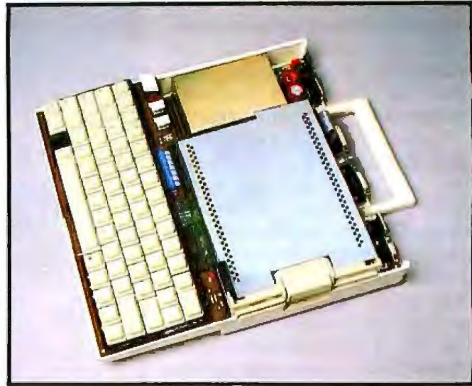
Photo 6: View of the IIc's internal 5¼-inch disk drive. The drive was initially designed to face backward but in the final design faces the side of the case. The drive is heavily shielded and ventilated.
