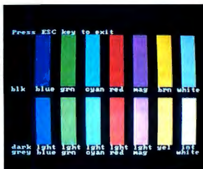
Photo 2: Color (2a) and graphics (2b) tests demonstrate TBASIC's support of colorgraphics commands normally associated with BASICA.
