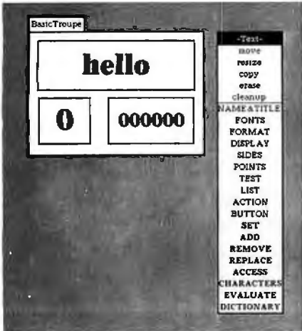
Figure 3: A BasicTroupe, containing a Text, a Number and a Counter, and a category menu for the Text performer.
