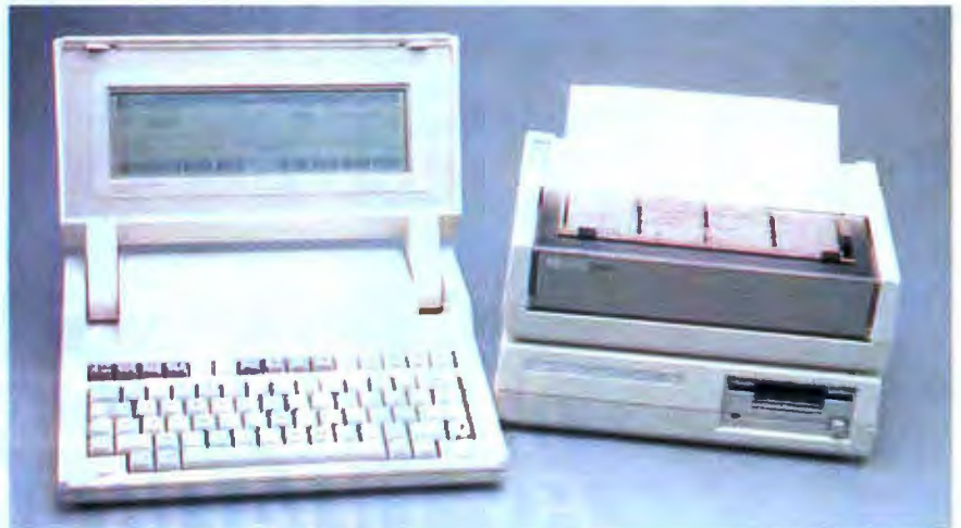
Photo 1: The HP 110 links to two optional battery-powered peripherals, the HP 2225B ink-jet dot-matrix printer and the HP 9114 single 3 1/2-inch disk drive.
