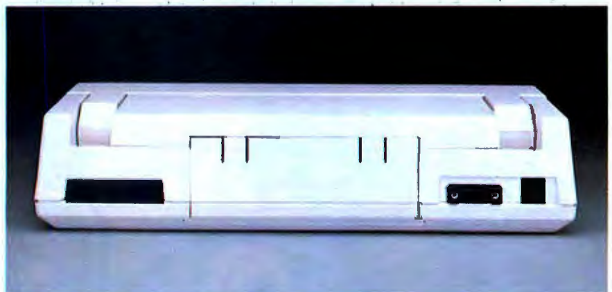
Photo 2: The back view of the HP 110. Shown from left to right are the two connections for the HPIL serial interface, the socket for the plug-in recharger, a nine-pin RS-232C port, and a modular phone jack for the internal modem. The removable panel in the center provides access to the lead-acid batteries.
