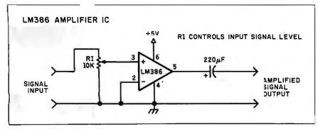
Figure 4: The sound-amplifier circuit.
