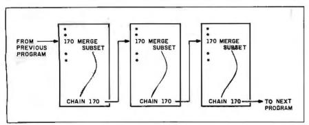
Figure 2: Chaining the demonstration modules.
