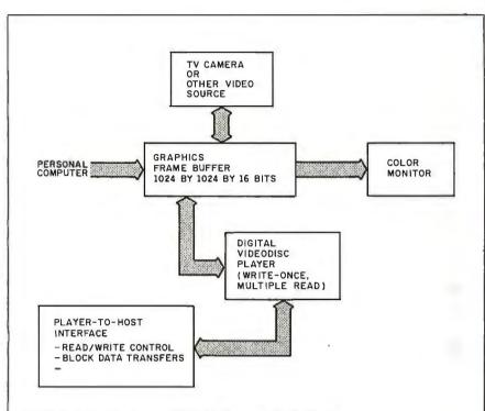
Figure 2: A second-generation interface built around digital television.
