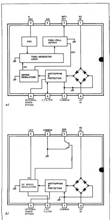
Figure 2: Texas Instruments CMOS ring-detector chips. (2a) Block diagram of the TCM1501A, TCM1505A, TCM1506A, and TCM1512A versions. (2b) Block diagram of the TCM1520A version.
