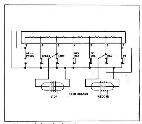
Figure 1: An example of external switch connection.
