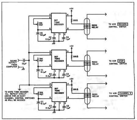
Figure 2: The computer-VCR interface circuit.
