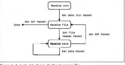
Figure 1: A simple state diagram for Kermit receiving files.
