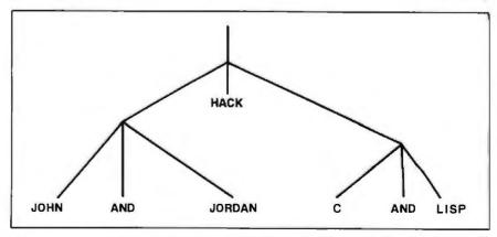
Figure 1: A list can be visualized as a tree; the terminal nodes are atoms, the nonterminal nodes are lists. The tree shown represents listing 1.
