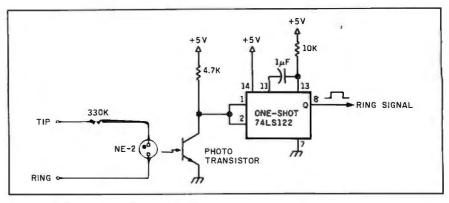
Figure 1: A simple ring-detector circuit.
