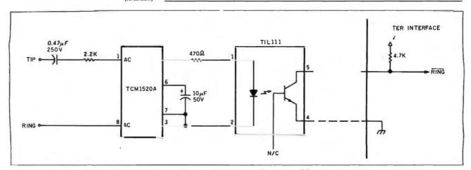
Figure 4: A two-chip ring-detection circuit that provides an optoisolated ring-detector signal for your computer.
