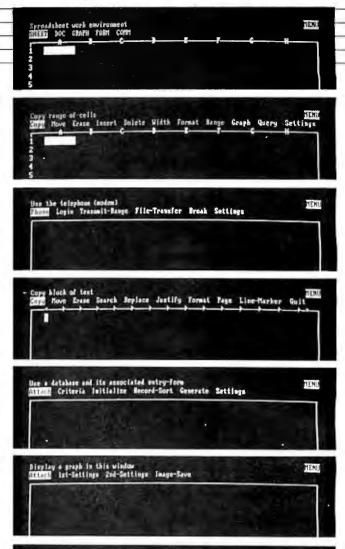
Photo 2: A full complement of Symphony menus, beginning with a start-up menu followed by spreadsheet, communications, word processing, database, graph, and a window-management menu.
