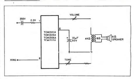
Figure 3: A typical ring detector using the TI ring-detector chip.
