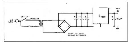
Figure 3: The regulated power-supply circuit.
