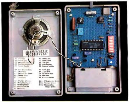
Photo 2: A view inside t Whimsi-Bell prototype. The doorbell synthesizer chip can play 25 different tunes.
