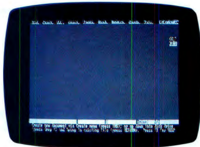
Photo 1: The Framework desktop in its initial state. Menus along the top edge can be accessed by holding down the control key and the first letter of the menu title.
