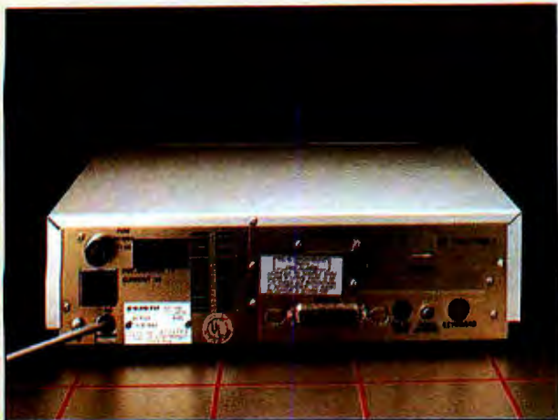
The rear panel of the Sanyo MBC-550. Note the parallel printer connector.
