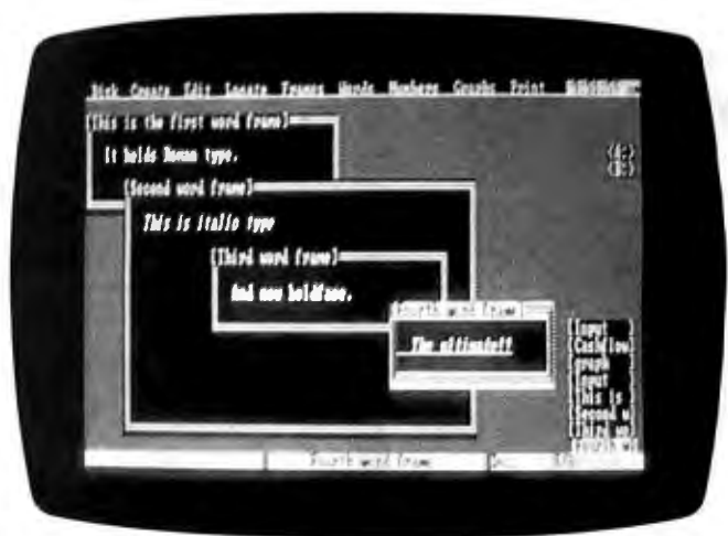
Photo 3: The stack of "trays" (bracketed titles) to the lower right shows all frames available on the desktop in the order in which they were created or opened.
