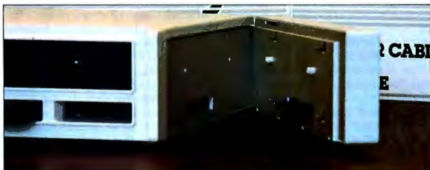
Photo 5: Some options, such as the parallel-printer adapter shown here, attach to the bus connector on the right-hand side of the PCjr.
