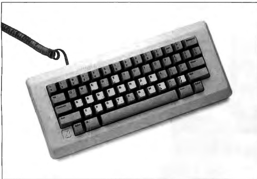
Photo 3: The Macintosh keyboard. Note the absence of a control key, but the presence instead of a "cloverleaf" key just to the left of the space bar. This key performs several of the functions usually performed by a control key.
