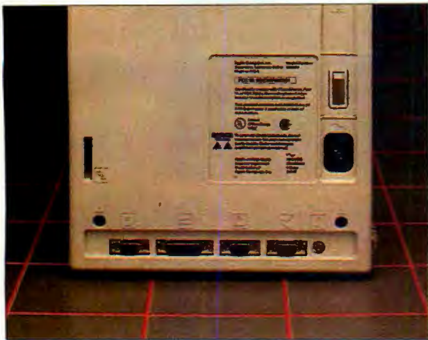
The rear of the Mac. Note the icon labels. The bottom row of connectors is for (from left) the mouse, second floppy disk, printer, modem, and speaker.
