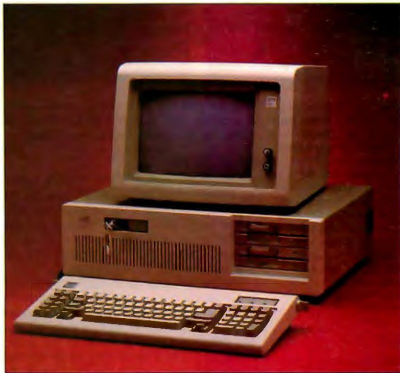
Photo 1: The IBM PC AT with a 20-megabyte hard-disk drive. This unit is equipped with an IBM monochrome monitor and a second, 360K-byte floppy-disk drive. Note the switch lock on the front panel.
