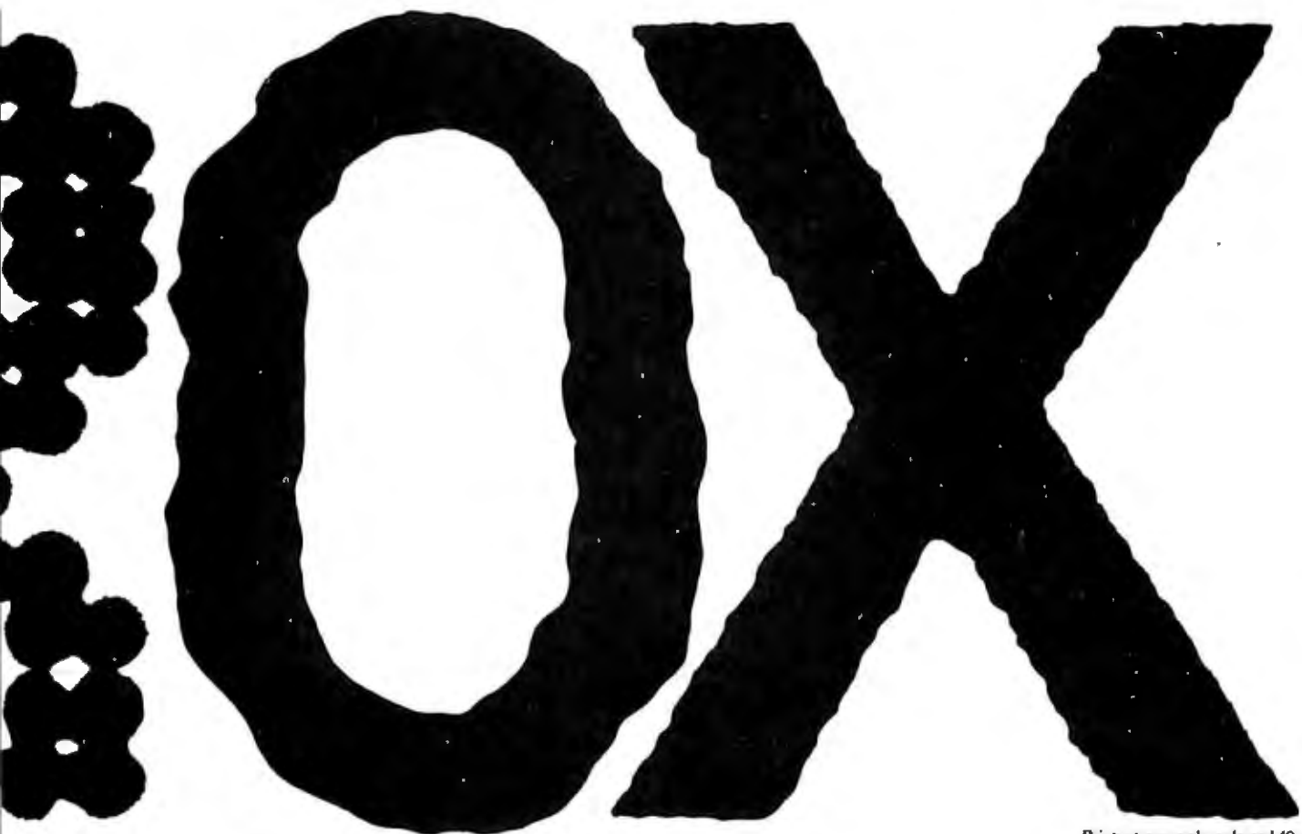
Printer typography enlarged 40x.
