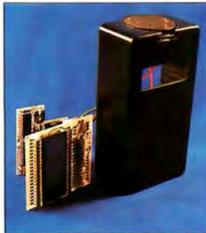
Photo 5: A front view of the disassembled tape measure.
