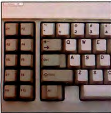
Photo 2: Inside the IBM PC AT. The expansion bus is at the left. Note the connectors for extra address and data lines. A 20-megabyte hard disk is in the lower middle. The power supply is in the upper right. Photo 3: Close-ups of the IBM PC AT keyboard. Note the proper position of the Shift key (left). Also note the indicator lights in the upper right and the large size of the Return (Enter) key (right).
