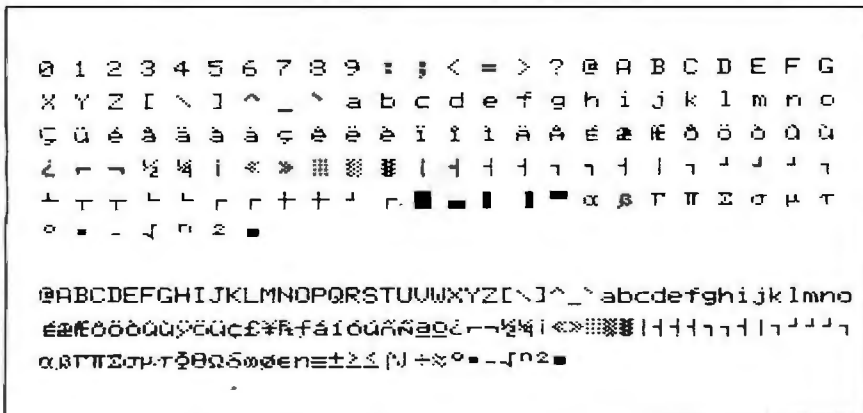
Figure 1: An example of text characters printed in 10 cpi (characters per inch) by Panasonic's internal thermal printer.
