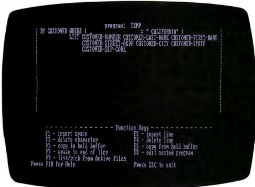
Photo 4: When SALVO finds a word it doesn't know in an otherwise acceptable query, it allows dropping into source code and entering the needed information.
