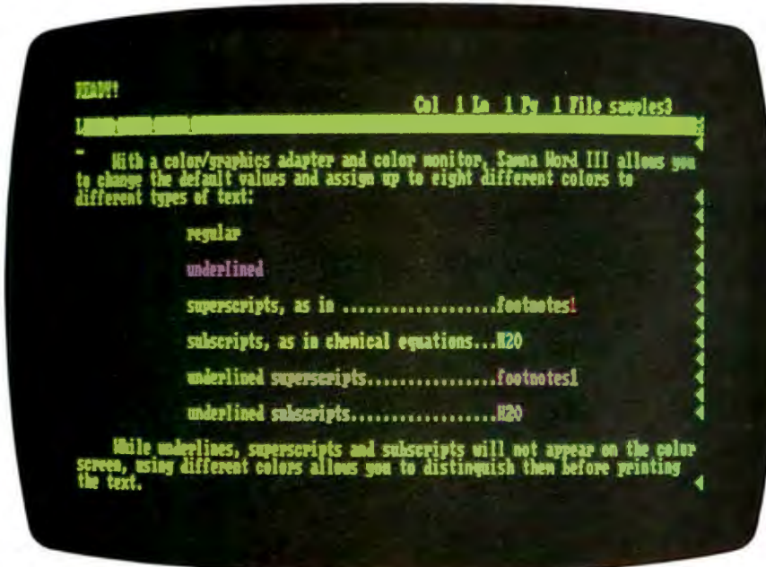
Photo 2: With a color graphics adapter and a color monitor, Samna Word III can mark underlined, superscript, and subscript text in different colors.
