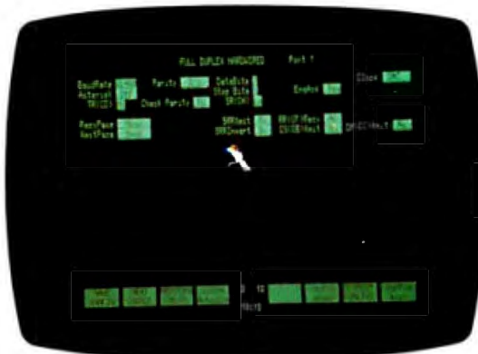
Photo 3: The configuration screens that allow you to configure ports 1 and 2 are identical, and each can be configured as either full-duplex hard-wired, shown here, or full-duplex modem.
