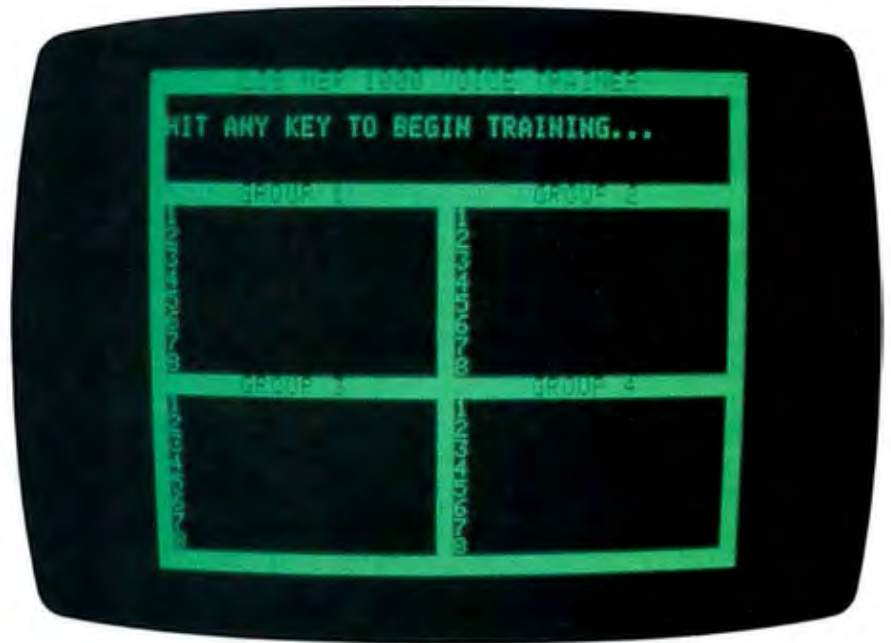
Photo 4: In this training mode, you select and train up to 32 words at a time. Multiple overlays of these template dictionaries result in potential recognition vocabularies of thousands of words. In practice, 64 concurrent-available words is a reasonable search vocabulary that maintains a high response reaction time.
