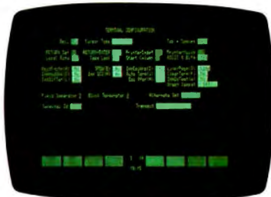
Photo 5: The terminal configuration screen controls the basic keyboard and display functions of the HP 150.
