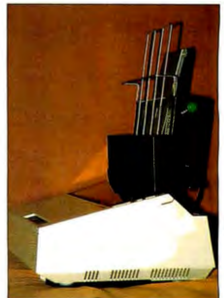
Photo 2: The Brother HR-15 printer with the optional cut-sheet feeder attached.
