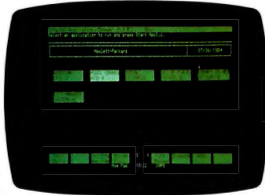
Photo 8: The PAM screen. The highlighted box is the currently selected application. The small arrow over these boxes is controlled by the cursor keys and points to a new application. Touching the leftmost softkey would start the selected application.
