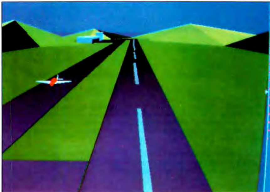
Photo 1: This is a frame from a real-time flight-simulation display. A simulator based on the GMP might be affordable by small airports and flight schools. The screen is updated at 30 frames per second to provide a realistic, moving view corresponding to the plane's position in space. The objects in the scene are defined as polygons in a three-dimensional space.
