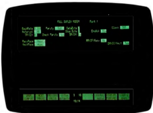
Photo 4: The full-duplex modem configuration, which is slightly less complicated than the full-duplex hard-wired configuration and has the receive and transmit signals reversed.
