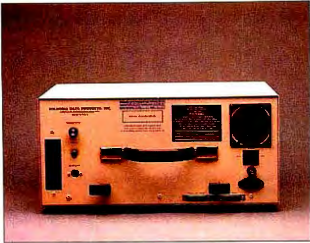
The rear panel. The parallel and serial ports are at the lower right. The expansion slot protector plate is at the far left.
