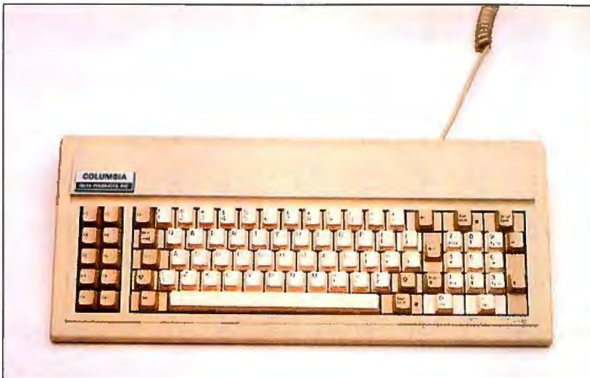
Photo 3: The VP's keyboard. Except for the Shift Lock and Num Lock key LEDs, the keyboard is laid out like the IBM PC's.
