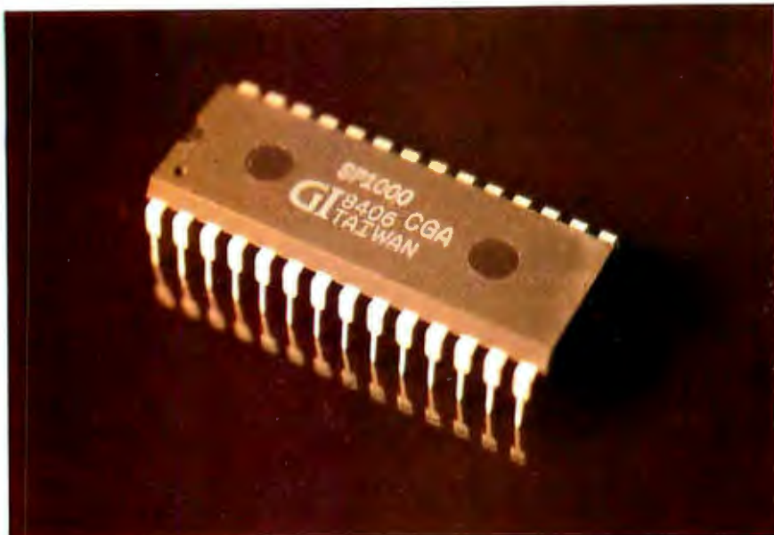
Photo 1: The General Instrument SP1000 voice-recognition chip.
