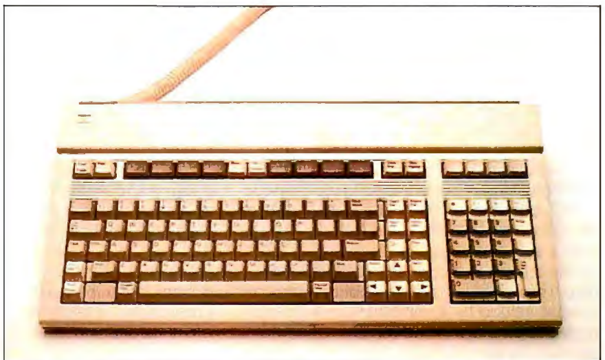
Photo 7: The keyboard of the HP 150 contains 107 keys arranged in seven groups. It connects to the back of the system processor/display unit with an RJ-11 plug.
