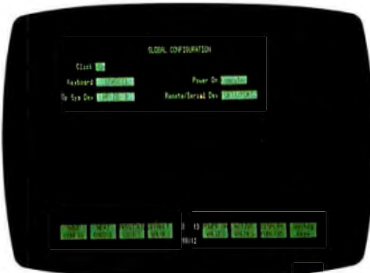
Photo 2: The Global Configuration screen allows you to set up the basic functions of the HP 150.
