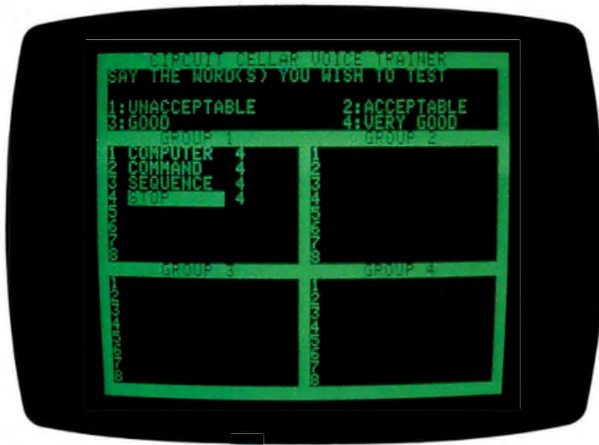
Photo 6: One of the features of the Lis'ner software is the ability to make and test a recognition vocabulary. In the modified editor program shown here, as the words are spoken, the acceptance level is noted so the user can select words with less interference. Words like "computer" and "sequence" have few differentiation problems. "Nine" and "mine" would present difficulties, as would "next" and "text."
