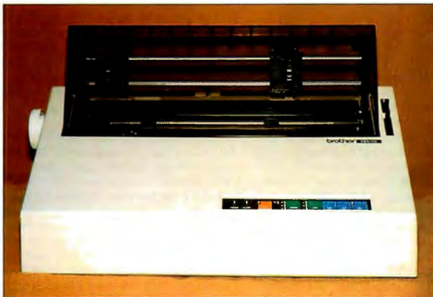
Photo 1: The Brother HR-15 printer with the optional tractor-feed mechanism attached.
