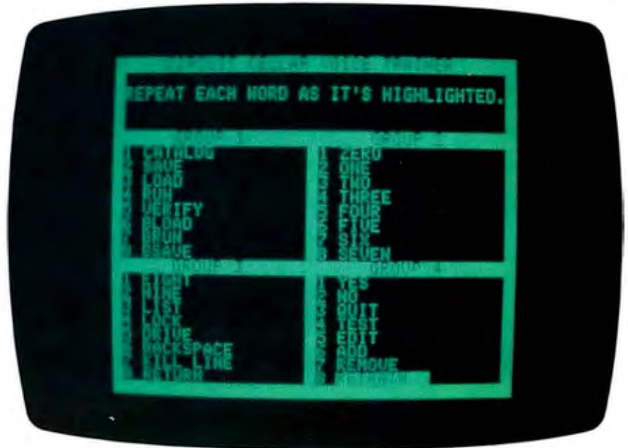
Photo 5: These standard DOS commands comprise one of the vocabularies that the user is directed to train. Once trained, many keyboard entries can now be verbal.
