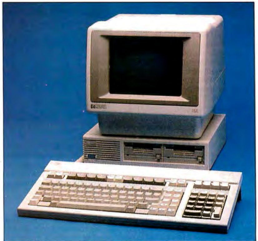
Photo 1: The HP 150 with a 9121 disk-drive unit.
