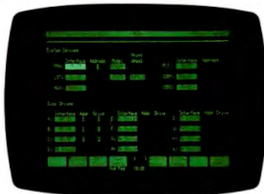
Photo 6: Hewlett-Packard has further developed MS-DOS by providing the user with this handy configuration screen. Here the user can relate MS-DOS's logical device names (PRN:, COM2:, etc.) to the actual physical devices and where they are connected to the computer (port 1, HPIB, etc.).
