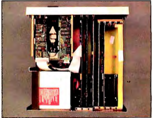
The inside of the Z-150. Note that there is no motherboard in this computer.
