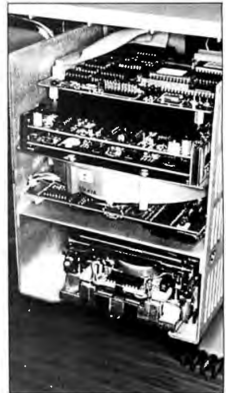
Photo 3: A close-up of the 10-megabyte drive and the Sony Micro-drive on the Lisa 2/10.
