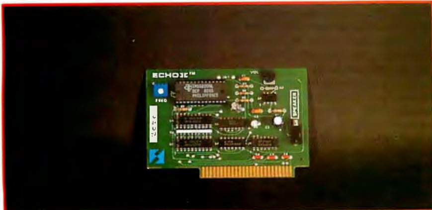
Photo 2: The Echo II circuit card includes the speech chip from Texas Instruments.
