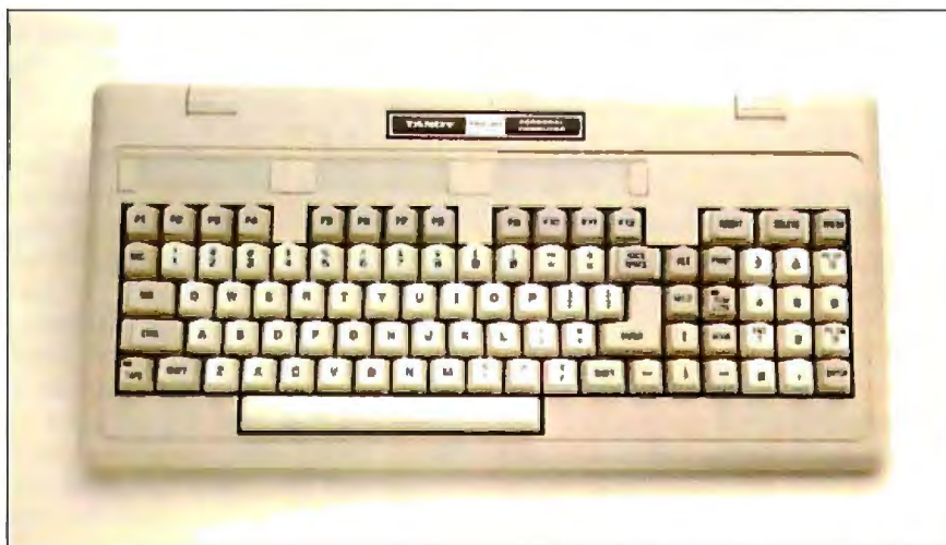
Photo 2: The Tandy 2000 keyboard features 12 function keys, Caps and Num Lock keys with lighted indicators, and a large Enter key.
