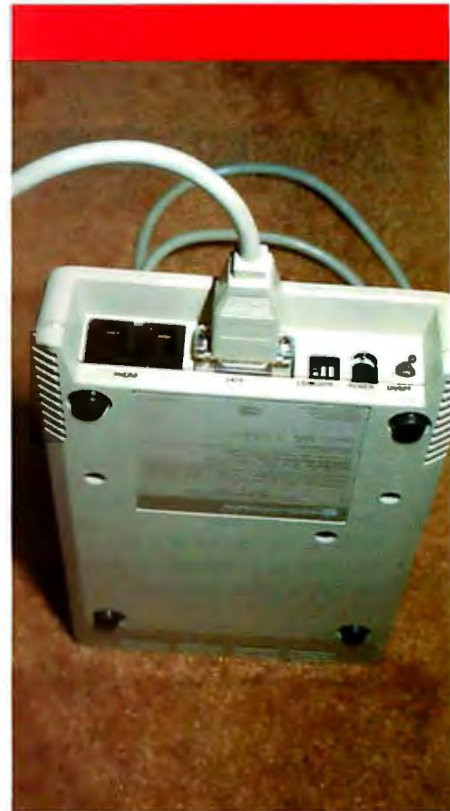
Photo 2: The modem's rear panel serves as the mounting space for incoming and outgoing modular telephone jacks, three DIP (dual-inline pin) switches, power plug, on/off switch, and DB9 female connector. DIP switches control carrier-detect mode, balance capacitor insertion, and respond to data-terminal-ready signal.
