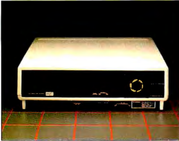
The back panel of the Tandy 2000. The serial and parallel ports are along the bottom.
