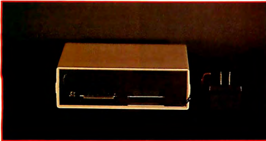
Photo 3: The Intex Talker rear panel features a serial and parallel port, as well as an external speaker jack.
