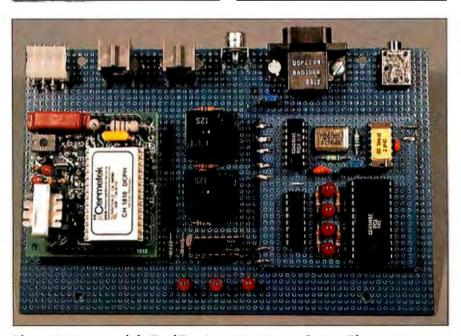
Photo 3: Prototype of the Touch-Tone Interactive Message System. The connectors from left to right are the power supply, answering-machine connector, telephone-line input. Microvox speech-synthesizer output, parallel I/O interface to computer, and the answering-machine earphone output.
