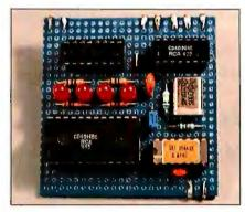
Photo I: Prototype of the DTMF receiver board.
