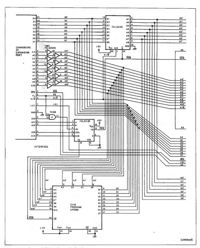
Figure 2: A schematic of the 80-column video board.
