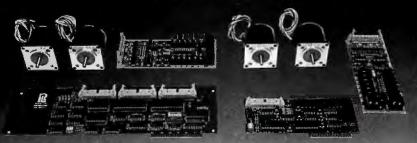
Complete 2 axis systems using 2 size 23 stepper motors with R2D23 dual-axis driver; cable & powerful system software, expandable to 4 axis.
