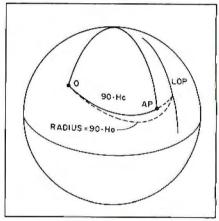
Figure C: In this case 90–Ho is greater than 90–Ho. Your actual position lies on an arc (LOP) of a circle of center 0 and radius 90–Ho.
