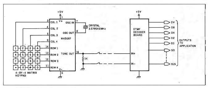
Figure 5: DTMF encoder/decoder remote-control circuit.
