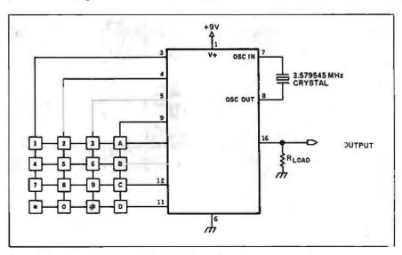
Figure 2: Schematic diagram of a DTMF-encoding circuit.
