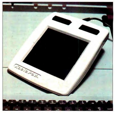
Photo I: The KoalaPad provides a method for entry of data or for making selections from the screen using touch rather than the keyboard.
