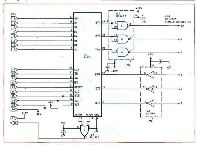
Figure 1: The serial-card schematic for the Sanyo MBC 550.
