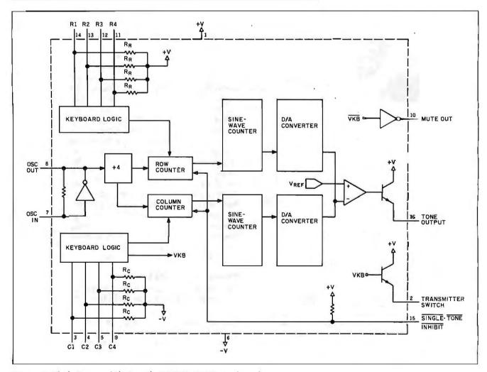
Figure 1: Block diagram of the Mostek MK5087 DTMF-signal encoder.
