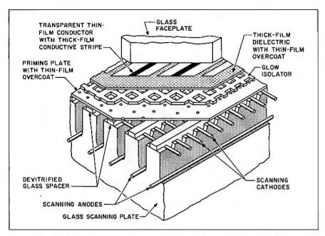
Figure 2: The hybrid AC/DC gas-plasma display developed by Burroughs Corporation to combine the virtues of the two types. An AC section serves as the display's memory, while the DC section is used for scanning the matrix.
