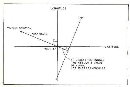
Figure D: Your assumed longitude and latitude form a coordinate system that contains the lower right corner of the triangle in figure B. The corner is formed by 90–Hc and your longitude. The LOP is a line drawn perpendicular to the radius of length 90–Ho. This drawing is hypothetical in that it assumes 90–Ho is greater than 90–Hc.
