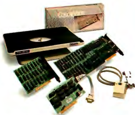
Princeton accessory product line. Undergraduate tilt/swivel monitor base, ColorView card, Green/Amber switch, RGB-80 card and Scan Doubler card.
