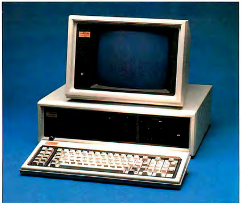
Photo 1: The Compaq Deskpro Model 4 with 10-megabyte hard-disk drive, 10-megabyte tape-cartridge system, optional second floppy-disk drive, and optional 12-inch green monitor. Note the clock-speed indicator light and keyboard plug to the left of the disk drives.
