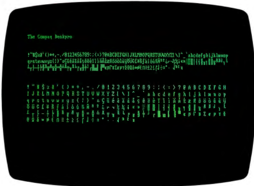
Photo 3: A display of the high-resolution, monochrome-text-mode character set on the Compaq Deskpro.
