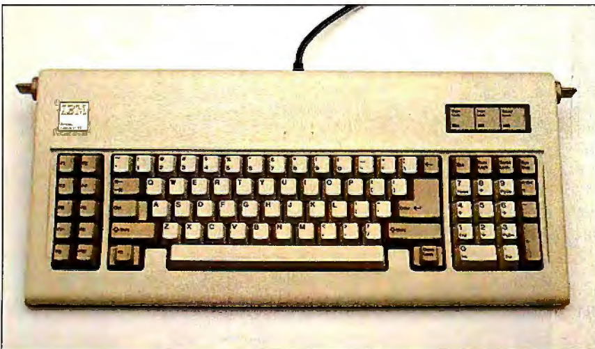
Photo 2: Close-up of the IBM PC AT keyboard shows the repositioning of the grave accent, Print Screen, Escape, and backslash keys.
