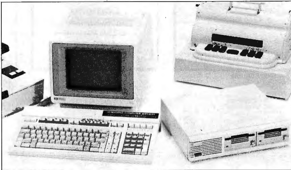
The Total Talk PC system based on the HP 150, along with some optional peripherals.
