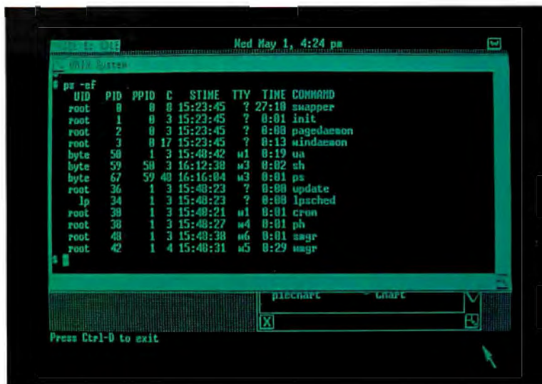
Photo 3: A UNIX window. This window is running the Bourne shell and behaves like a conventional UNIX system.
