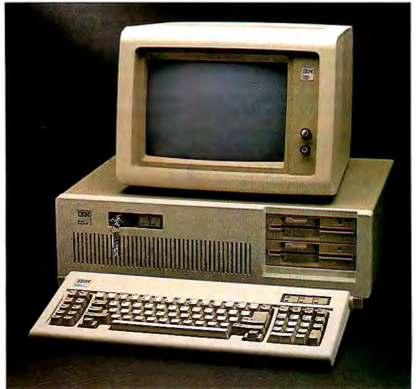
Photo 1: The IBM PC AT with a 20-megabyte hard-disk drive, 1.2-megabyte floppy-disk drive, and 360K-byte floppy-disk drive.
