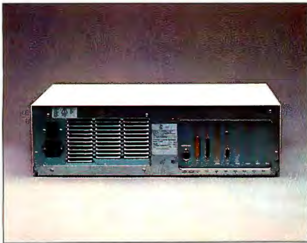
Compaq Deskpro with the serial/clock card in slot 1, the floppy-disk-controller/parallel-printer interface in slot 2, and the dual-mode display adapter in slot 4.
