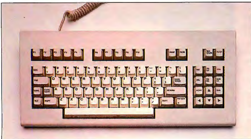
Photo 2: The Mindset keyboard includes two connectors for a mouse or joystick. Note the inverted-T cursor-key arrangement. The Sys Config key calls up the Configuration program stored in ROM.
