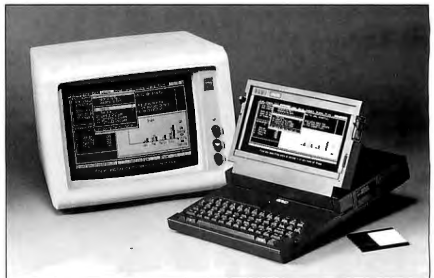
Photo 2: The GRiDCase III with the video-out option hooked up to an IBM color monitor. Ashton-Tate's Framework package is displayed on the screens. PC Master/Slave software allows easy cable connection from the GRiDCase to the IBM PC.
