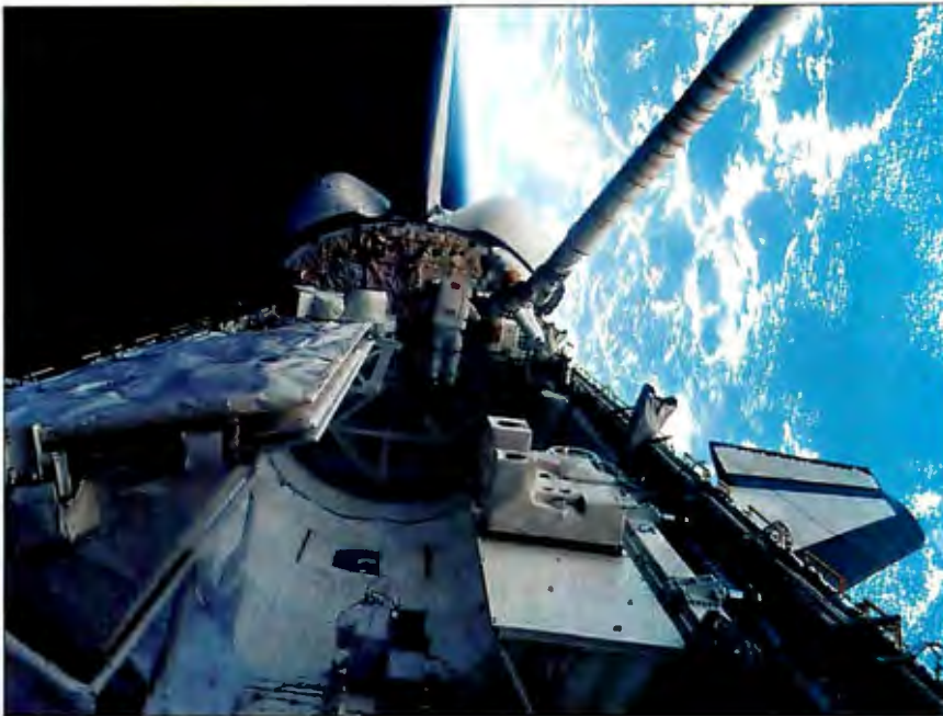
Photo 5: The SIR-B radar antenna in the payload bay of the spacecraft during the mission. The antenna, at the left, was built in three rectangular segments that were folded together when not in use. This was the case when this photo was taken. You can see most of the antenna's triangular support base, one of the hinges on which the segments of the antenna unfold, and, at the far left, a clasp that locked the antenna closed. The entire apparatus is covered with a white thermal fabric. Photo courtesy of NASA.
