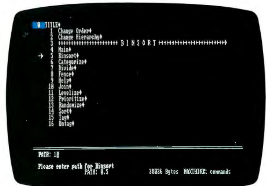
Photo 3: Binsort is one of the Brainstorm commands that make it easy to restructure MaxThink outlines. Binsorting is the manual process of assigning topics to groups or bins. You designate any number of bin topics (in this case two), and MaxThink inserts the Binsort separator line beneath them. You then point to each of the other topics and type the number of the bin where you want to put it as a subtopic. You could accomplish the same result with the Move command but not as quickly.
