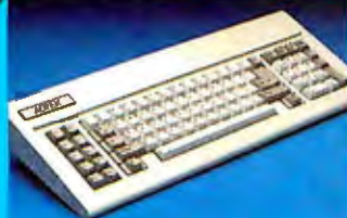
AT compatible keyboard. LED on cap, num and scroll lock keys.
