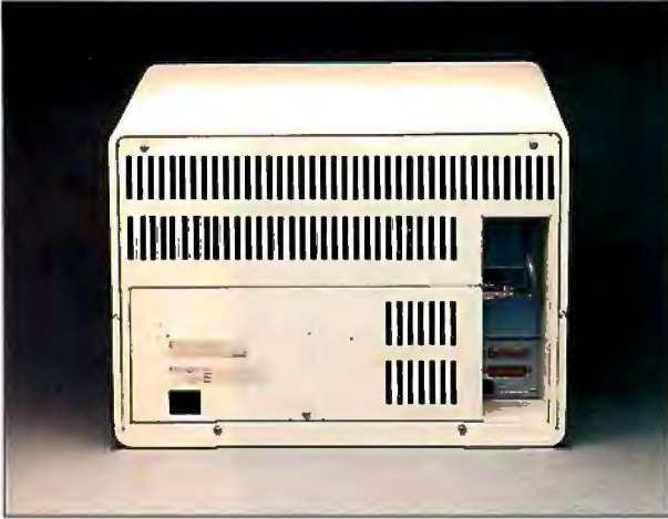
The rear of the NCR PC Model 4. The power supply is at left, the RS-232C and parallel ports are at right.
