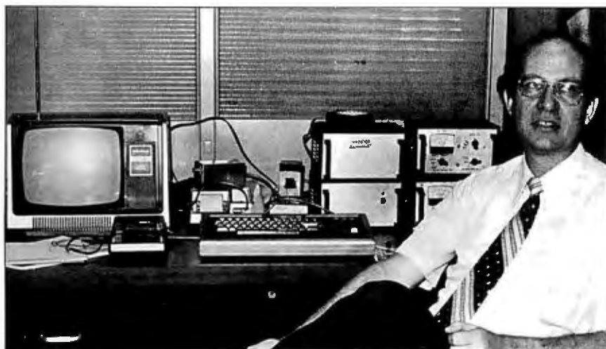
Photo 1: Laboratory testing of an early (1979) data-logging system for photoelectric astronomy. Developed by the author (right), this system used an early Radio Shack TRS-80 Model I microcomputer with 16K bytes of RAM. Programs and data were stored on cassette tape. The four electronic boxes on the right contained the computer interface, photometer DC amplifier, and high- and low-voltage power supplies.
