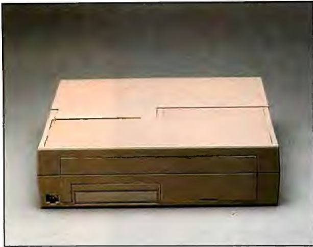
The rear panel of the Pro-Lite. Note the connector in the lower left corner for the AC/DC power adapter and the silver door that leads to the rear bus connector.
