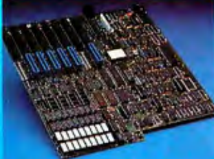
80286 motherboard, 256K standard memory, upgradable to 1M. Clock upgradable to 8MHz.
