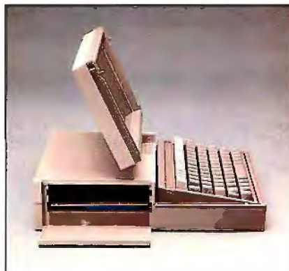
Photo 4: Behind the door on the Pro-Lite's left are the two slots for plugging in options: an RS-232C interface, 300-bps modem, external color monitor interface, or Solid State Software drawer.
