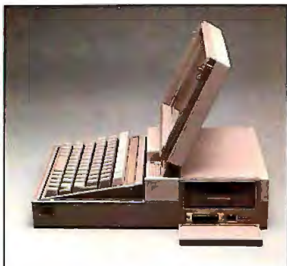
Photo 3: Behind the door on the Pro-Lite's right side is the 3½-inch disk drive, parallel printer interface, and power connector for a TI Portable Printer.
