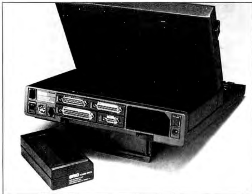
Photo 3: The GRIDCase back panel (left to right): the DIN connector for the IBM PC keyboard or 10-key keypad, the built-in 300/1200-bps modem (Hayes Smartmodem-compatible), RS-232C serial interface, external bus connector for external GRiD peripherals and access to the IBM PC expansion chassis, Centronics parallel interface, color (RGB) video-out for external monitors, built-in rechargeable/exchangeable battery pack.
