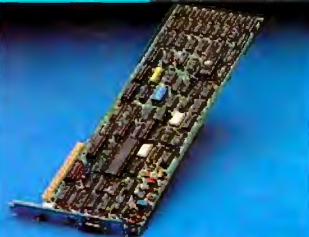
Video display and printer adaptor boards are fully interfaced with SERIES 286AT system.
