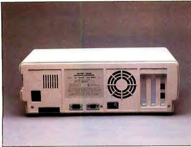
The rear panel of the Tandy 1000. Note the three expansion slots on the right, one of which is occupied by an internal modem.
