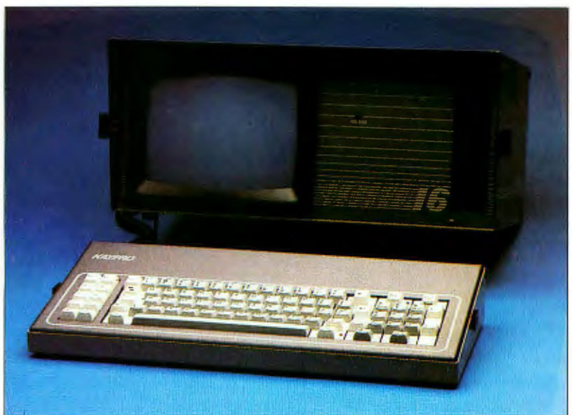
Photo 1: The Kaypro 16, an IBM PC- and XT-compatible featuring two floppy-disk drives or one floppy-disk and a 10-megabyte hard-disk drive (the latter combination is shown).
