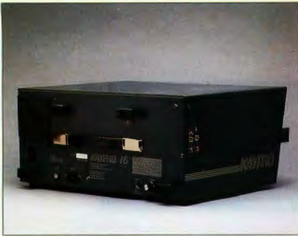
On the back of the Kaypro 16 are the on/off switch, power supply, keyboard interface, and display brightness control. On the left side are the parallel, serial, RGB, and composite video outputs.
