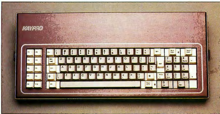
Photo 2: The Kaypro 16 keyboard with 83 keys, 10 IBM PC-compatible function keys, calculator keys, and Caps Lock and Num Lock indicator lights.
