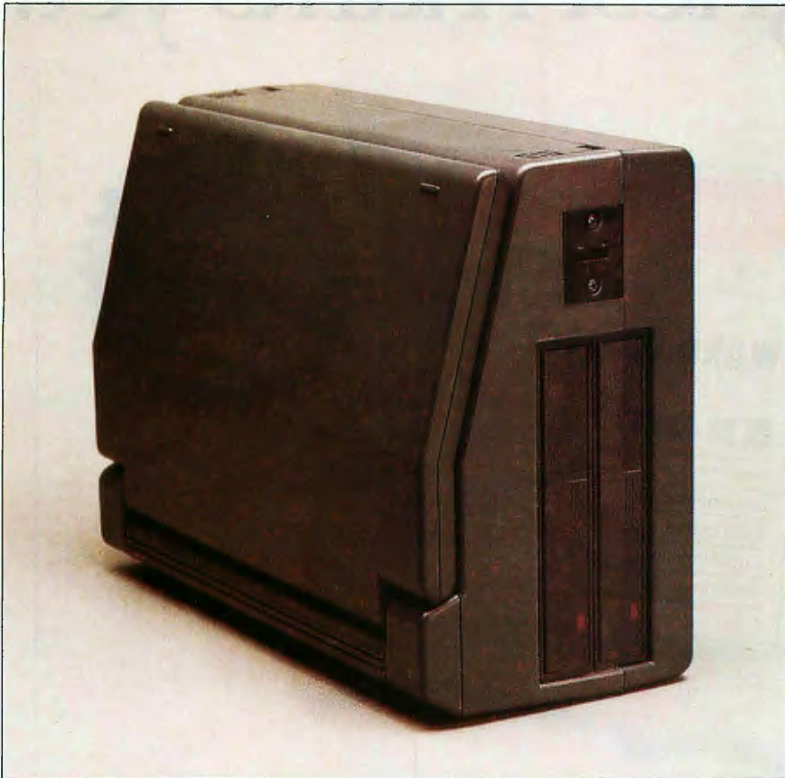
Photo 4: The right side of the Osborne 3 contains the two 5 1/4-inch floppy-disk drives.
