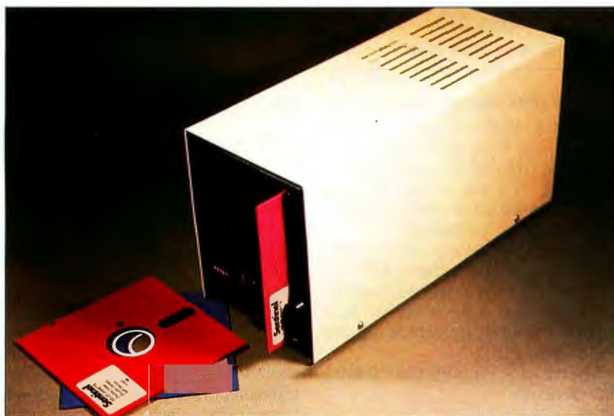
Photo 4: The enclosure from photo 3 is shown with the cover on. The only additional hardware necessary to use the system is a serial terminal.
