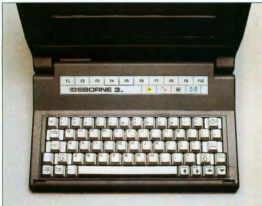
Photo 3: Close-up of the Osborne 3 keyboard shows the rows of special function and icon keys above the alphanumeric keys.
