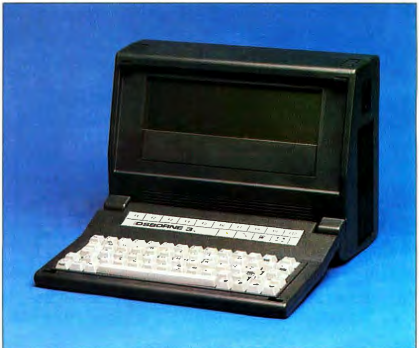
Photo 1: The Osborne 3 with an 80-character by 16-line liquid-crystal display and two 5¼-inch floppy-disk drives.
