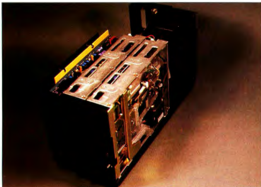
Photo 3: The SB180 can be packaged in many off-the-shelf enclosures advertised in BYTE. It fits comfortably to the left of a pair of half-height 5¼-inch disk drives in a case available from Disk Plus. This enclosure also includes the power supply.
