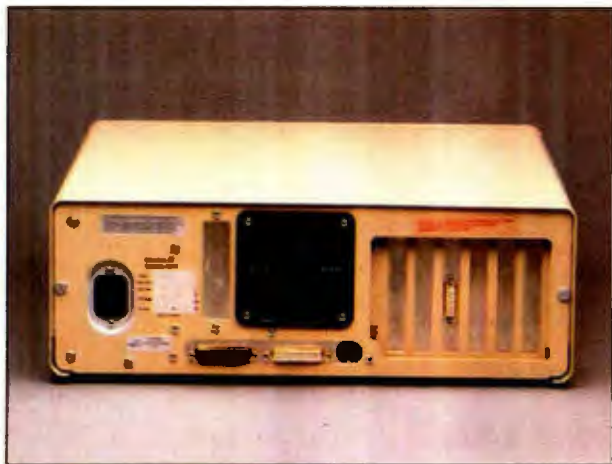
Rear view of the main unit showing the serial and parallel ports and output connectors from expansion ports.
