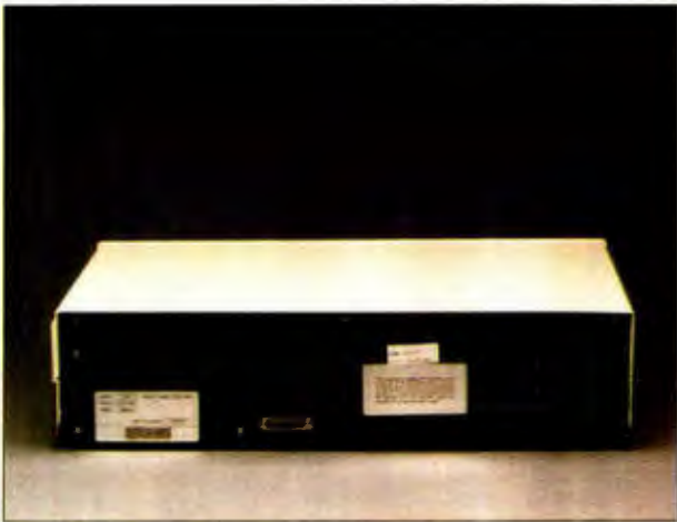
The rear panel of the Stearns has an asynchronous serial port and, to the right, a serial printer port.
