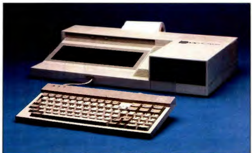
Photo 1: The STM Personal Computer with two 5¼-inch floppy-disk drives and an 80-character by 25-line LCD with electroluminescent backlighting.
