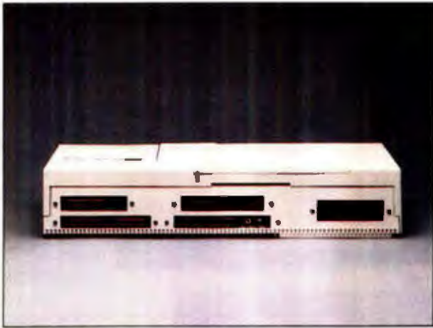
The rear view of the STM shows a full complement of connectors.
