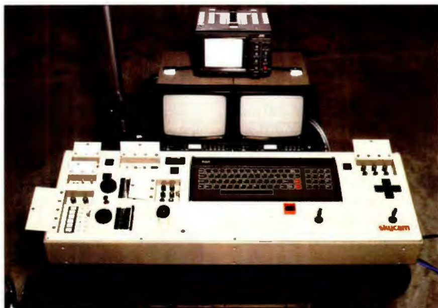
Photo 2: The Skycam console with the camera operator's panel at the left and the pilot's joysticks on the right.
