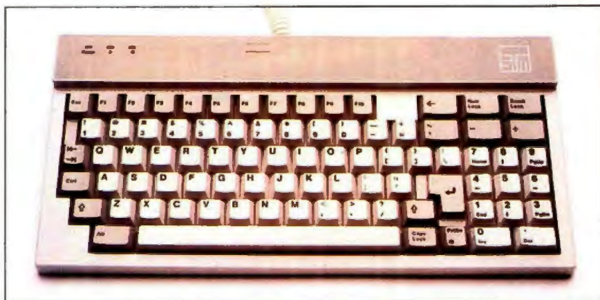
Photo 3: Keyboard for the STM Personal Computer. Note the enlarged return key and the special function keys on top of the alphanumeric keys.
