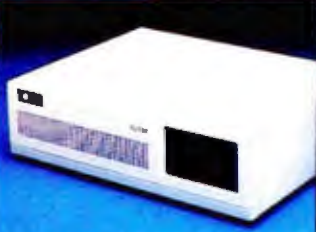
Fully AT compatible chassis, optional lock. Mounts standard floppy and fixed disk drives.
