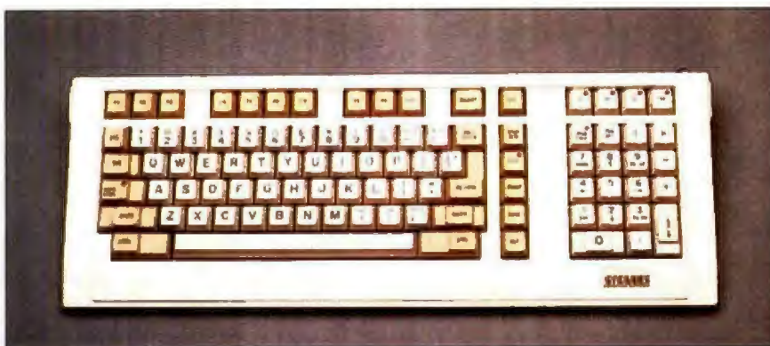
Photo 2: The Stearns keyboard. Note the placement of the Control, Alternate, and function keys.
