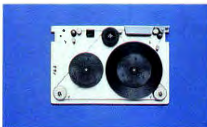
The Cartrex cartridge design (upper left) uses the N2 principle which creates head-to-tape tension by applying a mechanical differential at the rear pulley between a stiff transport belt and a stiff tensioning belt, indicated in green and yellow in the color schematic (upper right).
