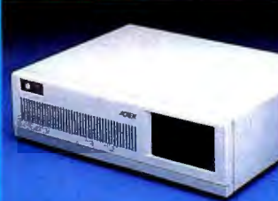
Fully AT compatible chassis with LEDs and lock. Mounts standard floppy and fixed disk drives.
