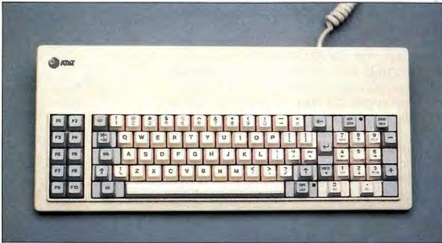
Photo 2: The AT&T PC 6300 keyboard. Note that the keyboard layout is similar to the IBM PC's except for the Num Lock and Caps Lock keys, which contain LEDs.
