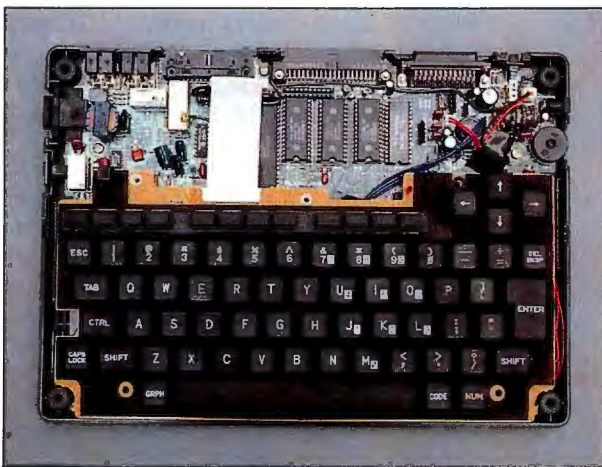
The Tandy 200's internal circuitry.
