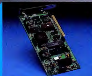
AT compatible disk controller handles 2 floppies, 2 Winchester.
