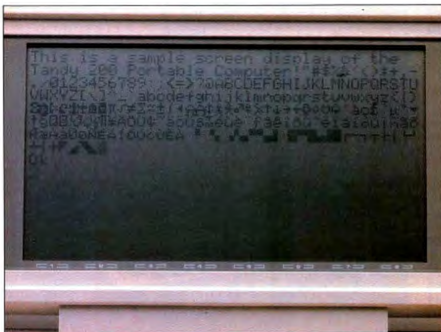
Photo 3: The Tandy 200's LCD displays 16 lines of 40 characters each.
