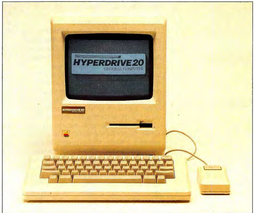
Photo 1: A Macintosh computer with a GCC HyperDrive 20 20-megabyte hard disk in it.
