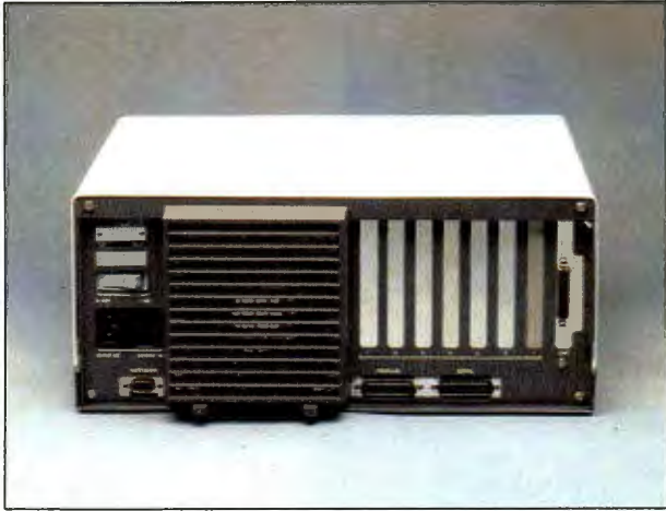
Rear view of the AT&T PC 6300 showing connectors for the serial port, parallel port, keyboard, and monitor. Note the oversized cooling fan, protective shroud, and connector access slots for the seven expansion boards.
