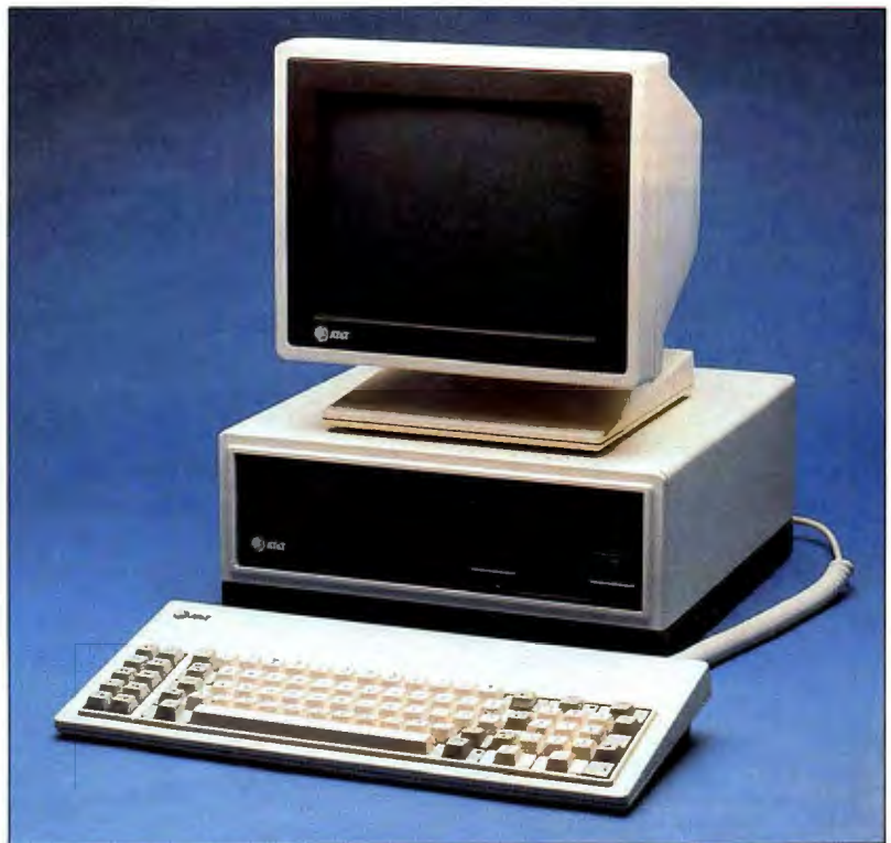
Photo 1: The AT&T PC 6300 with one floppy-disk drive, monochrome monitor, and keyboard.
