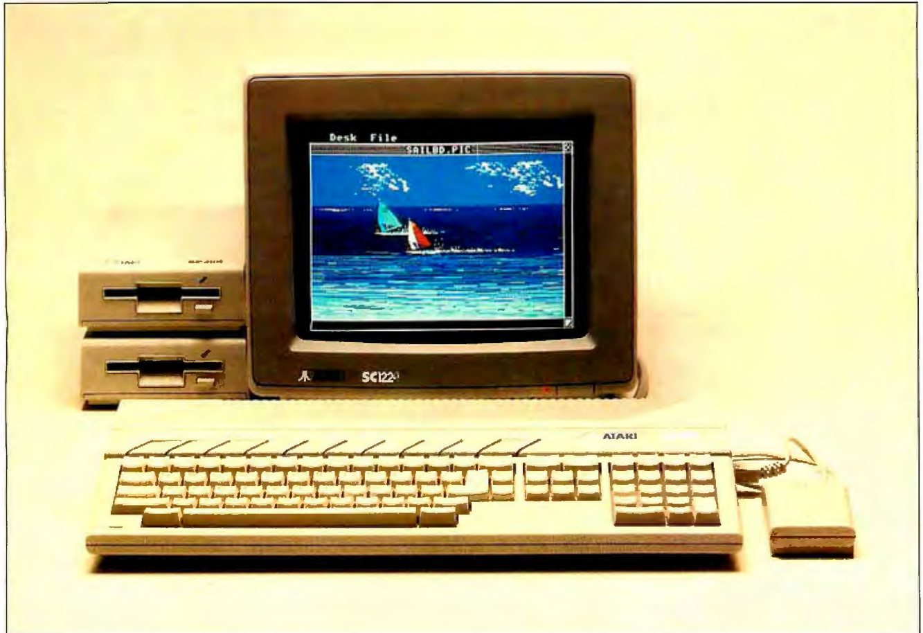
Photo 1: The Atari 520ST, shown here with the color monitor and two single-sided double-density disk drives. (a) On the right side of the keyboard unit are two joystick/mouse ports. (b) On the left is the 128K-byte ROM cartridge port. (c) The rear of the disk drives has specific ports for I/O in and I/O out.
