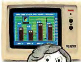
HX-12E. High resolution RGB monitor 640x350 lines noninterlaced - .28 mm dot pitch -Compatible with IBM Enhanced Graphics Adapter -Nonglare screen -$785
