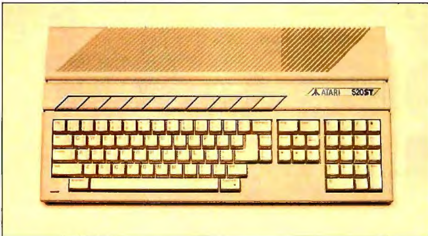
Photo 5: The 520ST keyboard. Wider keytops and the rhomboid shape of the function keys lessen the utility of an otherwise full-featured, well-designed layout.
