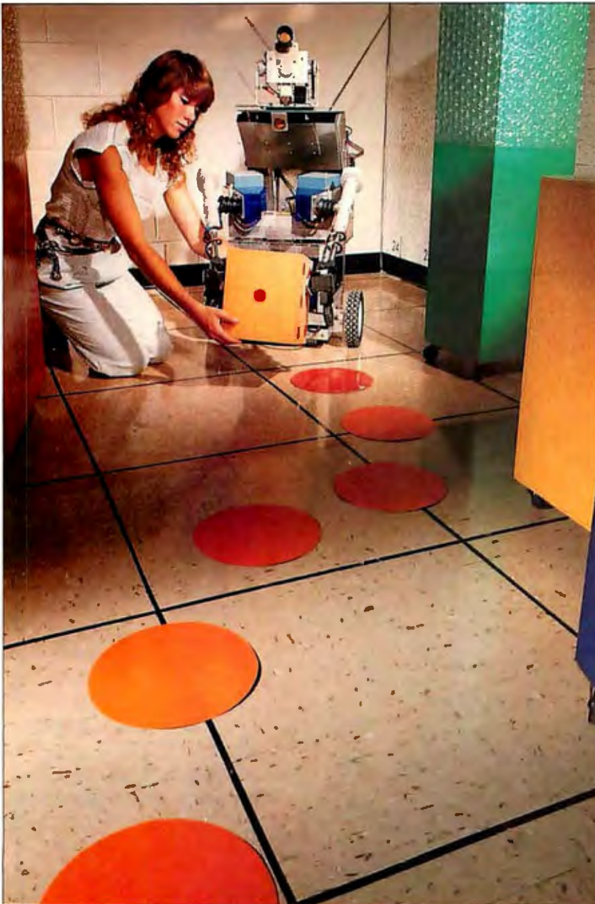
Photo 1: HERMIES (right) and friend. Notice the bubble wrap on the obstacles and the two-foot-square floor grids.
