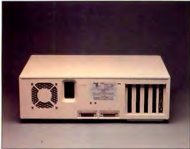
The rear view of the Canon A-200 shows (from left to right) the blower fan, power cord receptacles, serial port and parallel port, and expansion slots.
