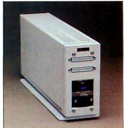
Photo 2: Rear view shows extra connection for daisy-chaining.
