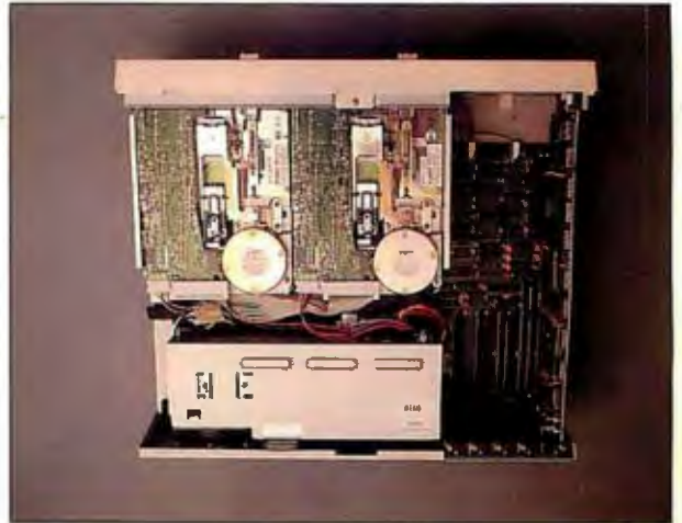
Inside the A-200. At the lower right are the expansion slots; the power supply is at the lower left. At the upper left are the floppy-disk drives.
