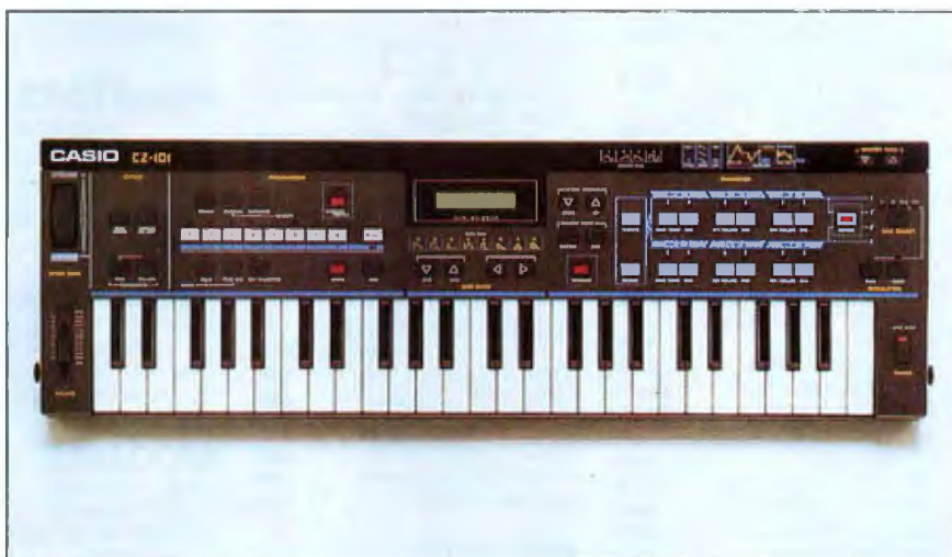
Photo 2: The Casio CZ-101 phase-distortion, programmable digital synthesizer.
