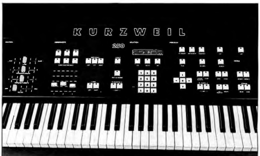
Photo 4: The Kurzweil 250 sampling synthesizer, which includes an optional user-sampling program.
