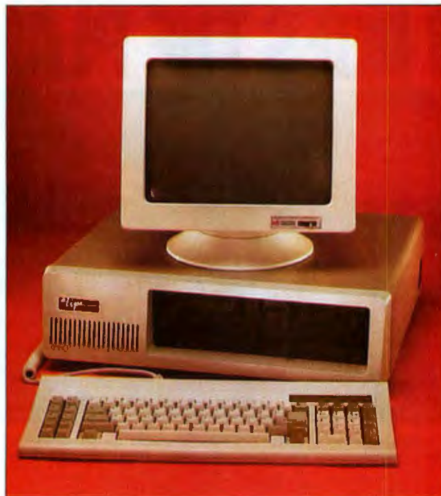
The JC LIPS computer, based on a NEC V40 processor.
