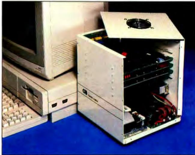
The Amiga Turbo Chassis, with 68020 and 68881 processors.
