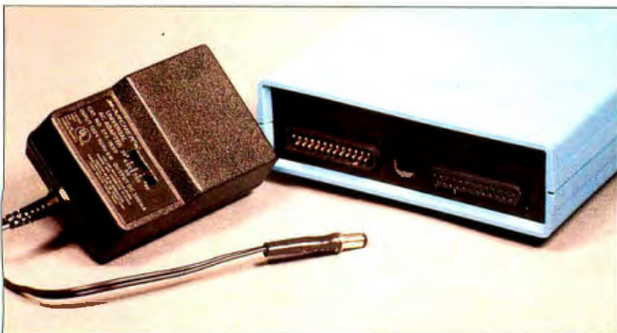
Photo 5: Power is supplied to the data encryptor by the wall-module power supply shown. The power supply plugs into the data encryptor between the two RS-232C connectors on the rear panel.
