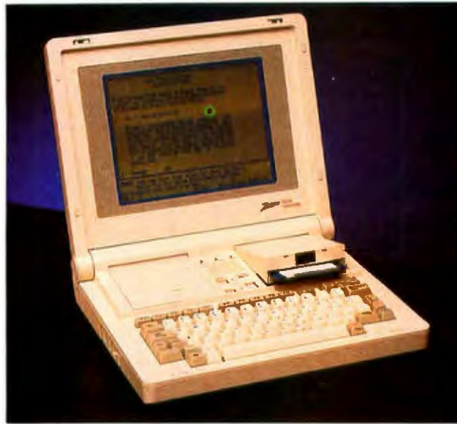
Zenith's Z-181, an IBM PC compatible with 640K bytes of RAM.
