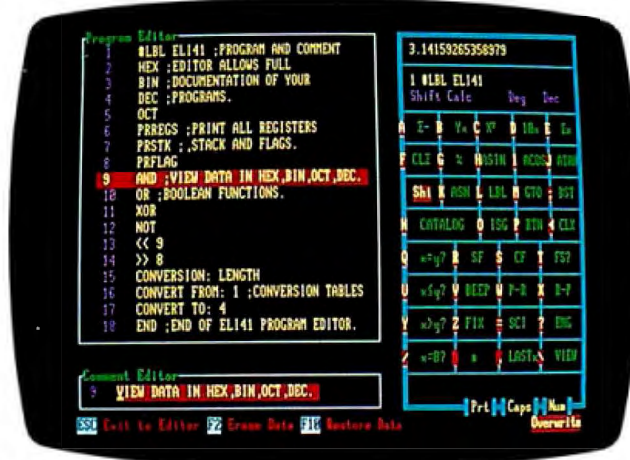
ELI-41 emulates the HP-41, with the calculator's keypad on-screen.
