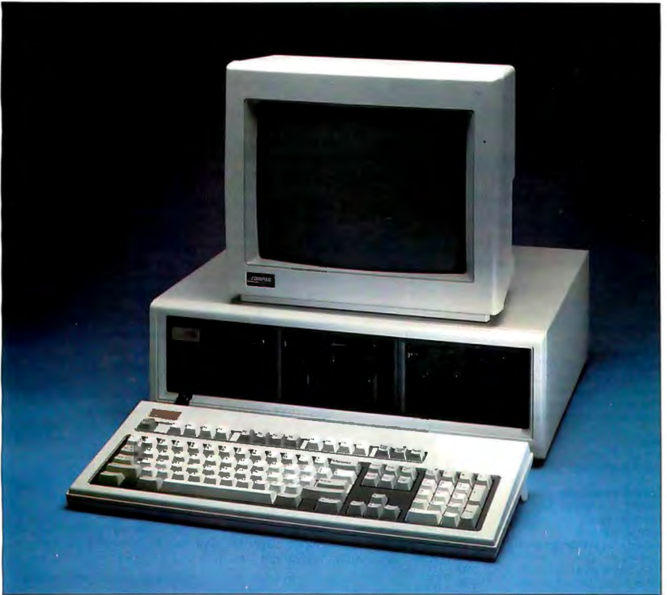
Photo 1: The Compaq Deskpro 386 with optional color monitor, 40-megabyte backup unit, and extra 1.2-megabyte floppy disk drive.
