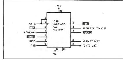
Figure 8: The HOLD PAL portion of the DSI-32 schematic.
