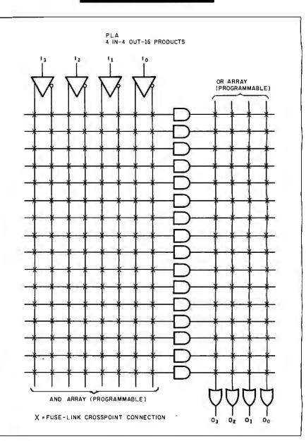
Figure 2: A simplified diagram of a PLA showing that both arrays are programmable.
