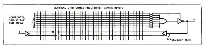
Figure 1: A logic cell from a 16L8 PAL. Notice the inverter between the OR gate and the output.
