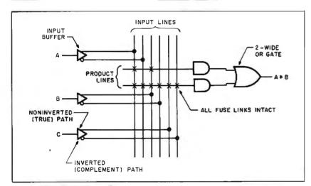
Figure C: Portion of the PLD array programmed to implement A\*B. Having all fuses intact in the second product line causes a logic zero to be input to the second AND gate, which does not contribute to the sum at the OR gate.
