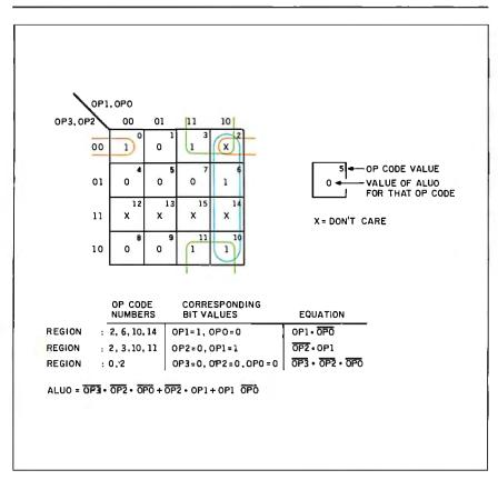
**Figure 5:** To show how the Boolean equations in figure 4 were derived from table 4, here is the Karnaugh map used to minimize the ALUO Boolean equation. The Xs are the don't-care bits, and the number in the upper right corner of each box is the op code.
