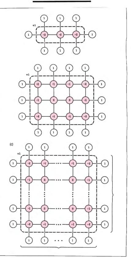
Figure 3: An example of block relaxation. By relaxing a block of nodes at once, we can eliminate redundant computations and greatly facilitate the solution of the cross section. The three figures show the templates for I by 3, 3 by 4, and m by n blocks. In all cases, each red node has its NODE value increased by I, and all nodes have their RESID values changed by the amount shown inside the circles. See the text for the details on constructing an m by n block template.
