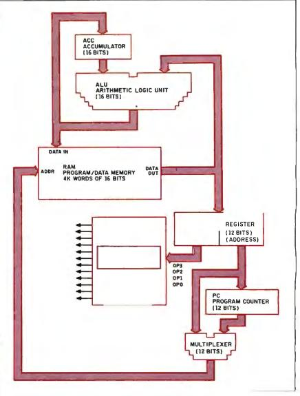
Figure 1: Toy architecture block diagram.
