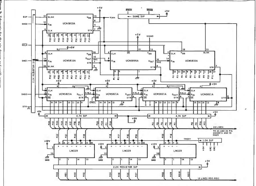
Figure 3: Schematic for the pin drivers and verify circuits.
