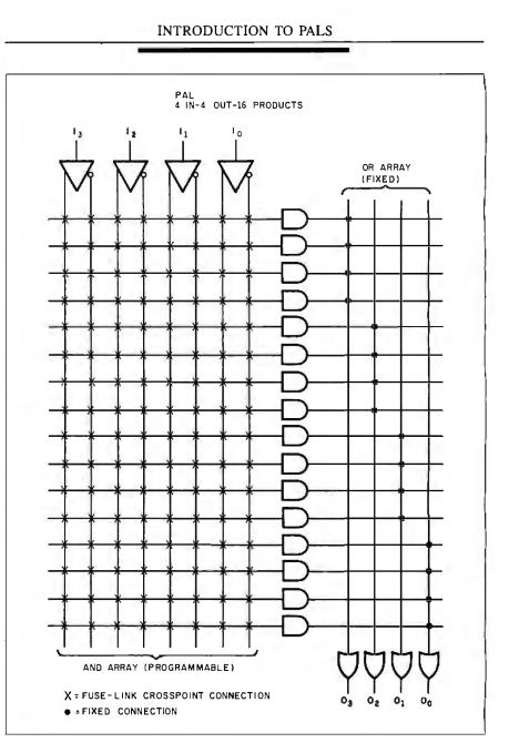
**Figure 3:** A simplified diagram showing the programmable-AND/fixed-OR array structure of a PAL device.
