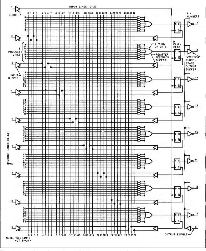
Figure 5: The actual logic diagram of the PALIGR8. Notice the D-type flip-flops at the outputs.
