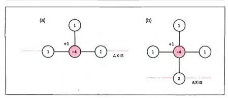
**Figure 5:** Symmetry in one dimension. When you relax only the unique half of a symmetrical cross section, the relaxation template changes for a node on the axis of symmetry (5a) or one node away from the axis (5b).
