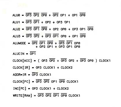
Figure 4: Logic equations for Toy's hard-wired implementation.
