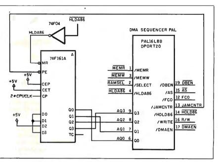
Figure 2: The DPORT20 portion of the DSI-020 schematic.
