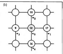
**Figure 1:** An intuitive analysis of node interrelationships. With a little arithmetic, we can see that node  $w_0$  in figure 1a (red) is correct because its value is the average of its four neighbors. Node  $w_0$  in figure 1b is not correct because it is less than the average of its neighbors.
