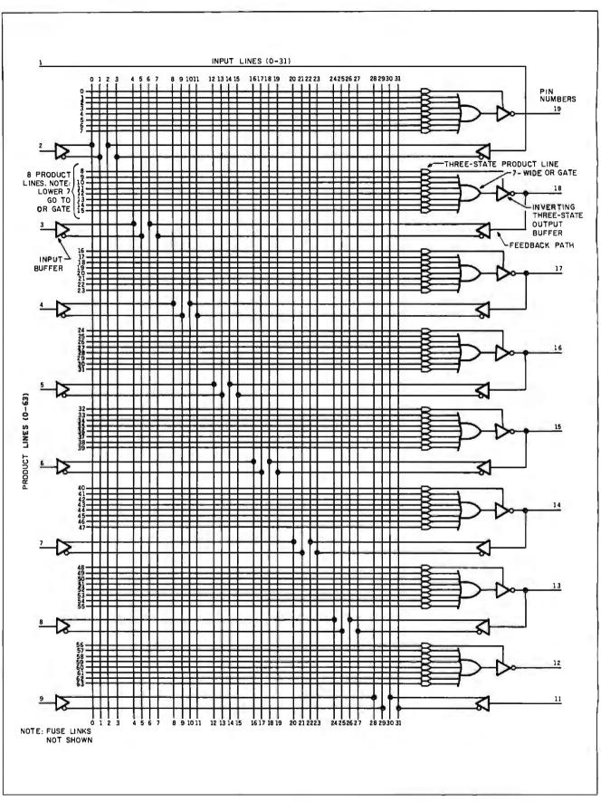
Figure 4: The actual logic diagram of the combinatorial PALI6L8. The fuse links are not shown so that a logic designer may place an X at those points where a fuse should be left intact.
