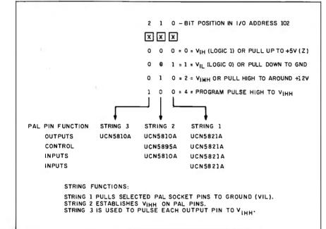
Figure 4: Relationship between a programming value written into ZAP-A-PAL's I/O port and the pin drivers.
