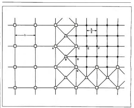
**Figure 7:** An example of using a graded grid. You can switch from a coarse grid (squares) to a finer grid (dark circles) by using a transition layer of nodes (triangles). In this way, you can get more precise answers in an area of interest without having to use the finer grid for the entire cross section. See figure 8 for the relaxation templates of the nodes marked A through G.
