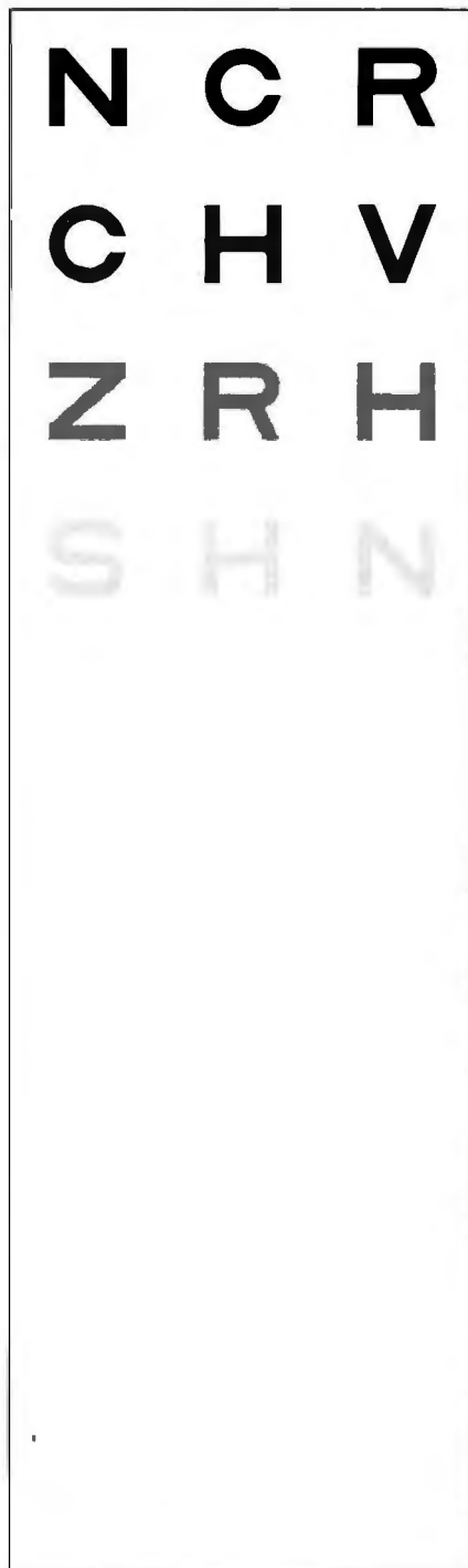
Figure 6: Pelli-Robson Letter Sensitivity Chart produced by listing 5 on a Linotype L300 at 2540 dots per inch. Copyright 1987 by Denis G. Pelli.
