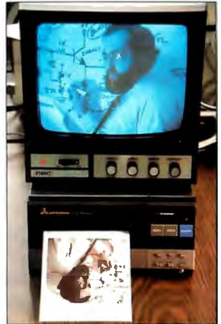
Photo 3: This is how a picture of me standing in front of a blackboard in Connecticut would be received by an ImageWise display/receiver board in California. A video printer like the Mitsubishi unit shown here can save the current scene while another is being transmitted.
