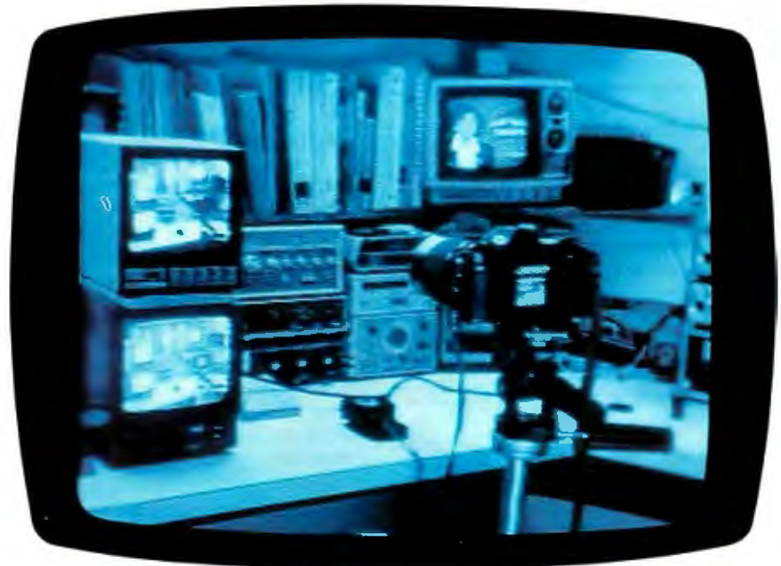
Photo 4: The equipment counter in the Circuit Cellar where I took most of the photos with the setup you see. The interesting point to realize here is that this picture is completely digitized. A video camera (out of view) is pointed at the two stacked monochrome monitors and the film camera. The monitor on the bottom displays the picture as it is produced by the video camera and input to the digitizer/transmitter board. The display on top shows the output of the display/receiver board after it receives the data from the digitizer. It is the object of view by the film camera. This picture is the screen of the top monitor.
