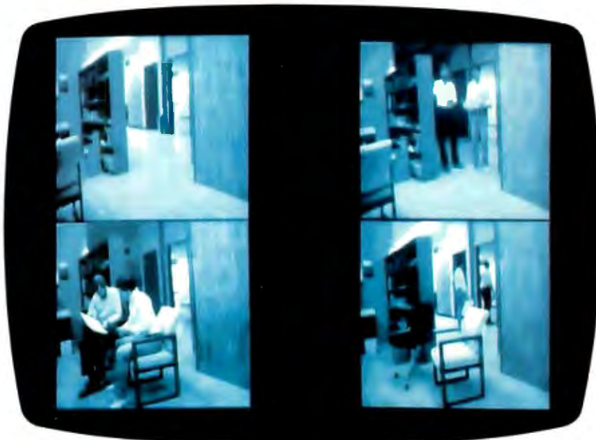
Photo 2: The ImageWise digitizer captures a high-quality gray-scale image that can be used in areas like security and pattern recognition. In the surveillance application shown here, an empty room is entered, used, and then exited. To save space in this presentation, all four scenes are displayed on a GT180 (in 16-level gray scale).
