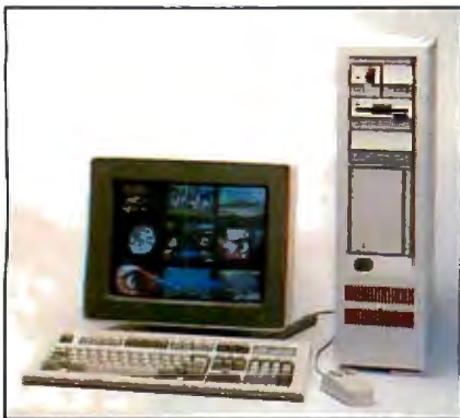
The PS/2 Model 80: IBM's first 80386-based computer.
