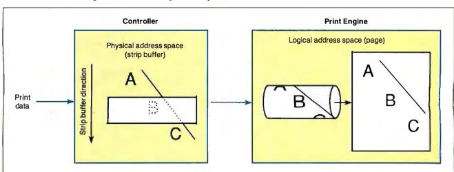
Figure 1: At any given time, the strip buffer contains only a partial-page bit image. In a process similar to virtual-memory techniques, the physical address space of the strip buffer scrolls across the much larger logical space of the printed page.
