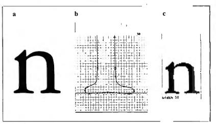
Figure D: Some type styles are not representable at resolutions below 800 dpi. The lowercase n (detail a) from Garamond #3 has wavering strokes and serif features that cannot be fit to conform to the grid (detail b). To get the effect of a finely wrought type face using 300 dpi, designers often trick the eye by adding dots where they don't belong (detail c).
