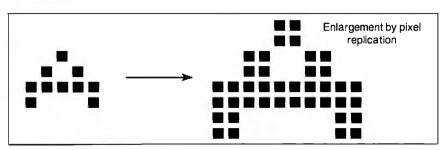
Figure 4: This shows the only method of enlarging a character stored in bitmapped form—pixel replication.
