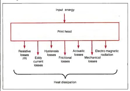
Figure 1: Types of losses associated with a DMI print head.
