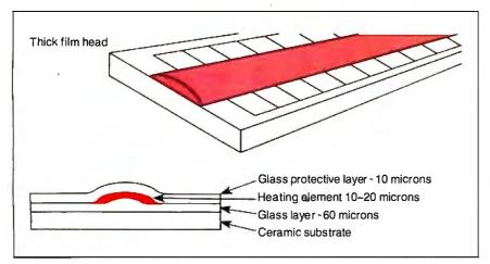
Figure 2: Thick-film heads offer durability and greater leeway in manufacturing tolerances.
