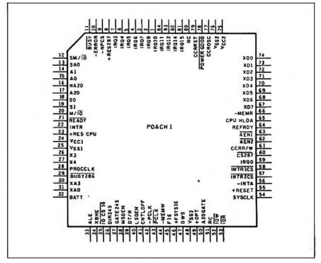
Figure 2: A pin-out diagram for the POACH1 chip.
