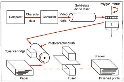
**Figure 1:** A schematic diagram of a laser printer. Raster-scanned light from a laser is deflected by a mirrored cylinder to expose the surface of a photoreceptor drum. The charged areas attract toner to the drum, which is then transferred to paper and fused on by heat.
