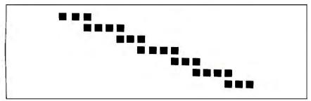
Figure 1: The staircase effect achieved when you try to plot a straight diagonal line on a raster device.
