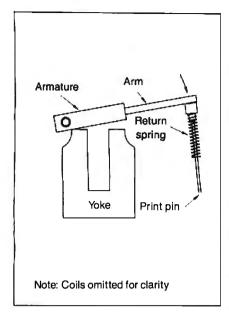
Figure 3: This U-shaped yoke and pivoted-armature model formed the basis of the computer-aided modeling process.
