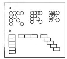
Figure 1: (a) Effects of varying degrees of dot overlap on the clarity of lines with circular dots. (b) Rectangular dots require no overlap for horizontal vertical lines.
