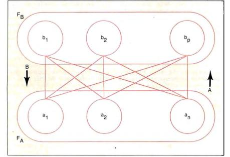
Figure 1: Topology of a BAM, showing the two fields of neurons connected by synapses.
