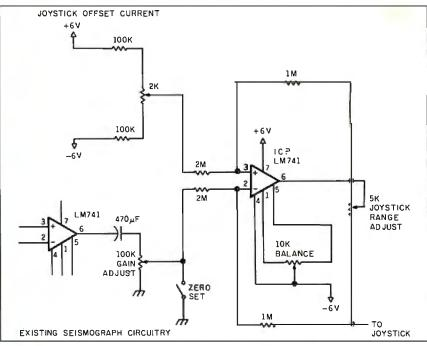
Figure 1: Amplifier circuit for seismograph.
