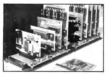
An A-BUS system with two Motherboards
