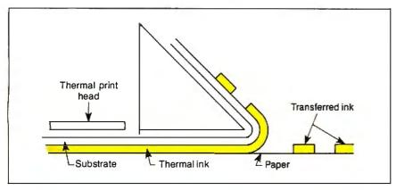
Figure 1: A simplified diagram of the thermal-transfer process.
