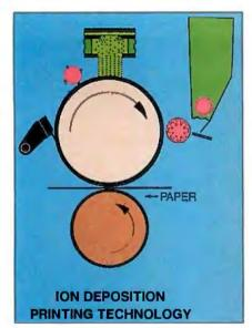
Figure 3: A schematic diagram of an ion-deposition printer. A modulated ion source (top) similar to that in a triode electron tube generates the ions, which are directed onto the drum, forming a latent image. The image attracts toner from the cartridge, which then is pressure-fused onto paper passing between the drum and a pressure roller. (Figure courtesy of C. Itoh Electronics Corp.)
