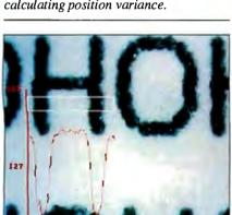
Photo 3: Edge sharpness is measured within the white border. The red graph shows the rate of fall of f from black to white.
