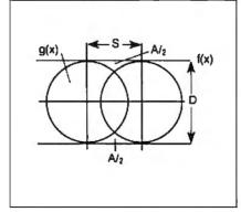
Figure 2: The blank area A is a function of dot diameter D, overlap S, the shape of the line f(x), and the shape of the dot g(x).
