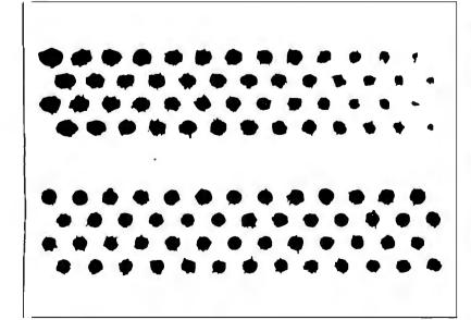
Figure B: An enlargement of a 300-dpi test pattern produced by Laserport, showing the system's ability to vary the dot size over a wide range.
