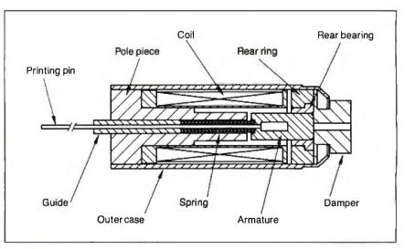
Figure 2: Coaxial solenoid used as an actuator in an early seven-pin design.
