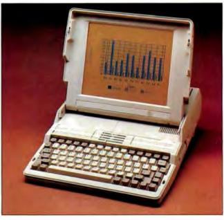
DG's upgraded Model 2T adds a supertwist backlit LCD.
