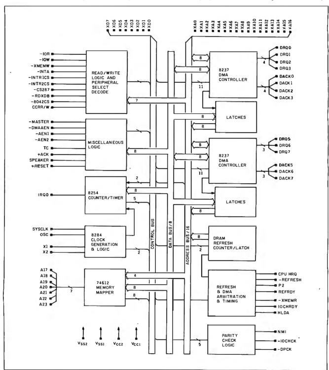
Figure 3: The block diagram of POACH2.
