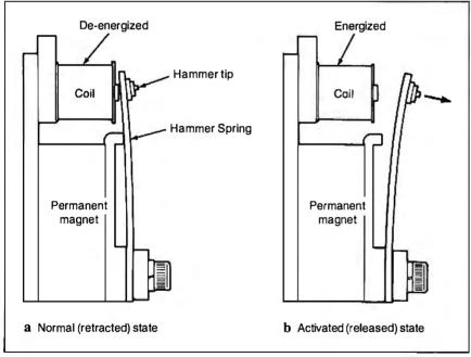
Figure 3: The hammer bank consists of 24 stored-energy print hammers. a) While the coil is de-energized, the permanent magnet holds the hammer in tension.
