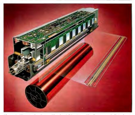
Figure 2: The print-head assembly of an LCS printer. The fluorescent bulb in the head provides light to the shutters, which open and close according to commands from the controller, charging selected dots on the photoreceptor drum. (Figure courtesy of Taxan USA Corp.)
