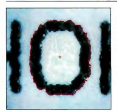
Photo 4: To measure edge roughness, we compare the perimeter of the original object to the perimeter of a smoothed version.
