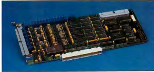
National Instruments' NB-AO-6 adds six DACs to the Mac II.
