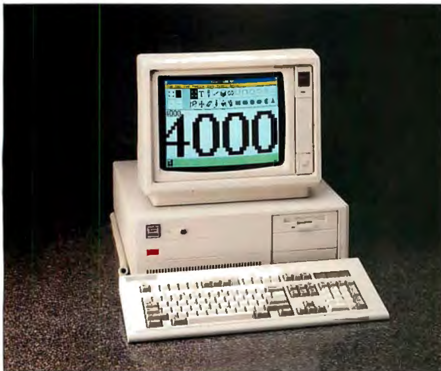
Photo 1: The Tandy 4000, an 80386-based machine.
