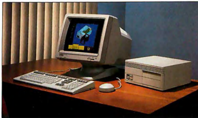
The VAXstation 2000 displays 1024-by 864-pixel color.
