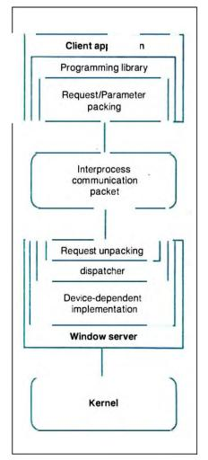
Figure 2: Client-server relationship. The window server manages all interaction with the display device and the input devices. Clients are user applications that request services from the server through the window programming library.
