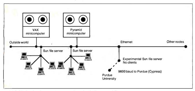
Figure 3: The distributed processing environment used at the University of Chicago.
