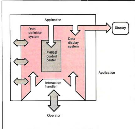
Figure 1: A block diagram of the PHIGS subsystem.
