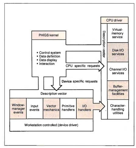
Figure 4: Figaro's CPU and device intelligence.
