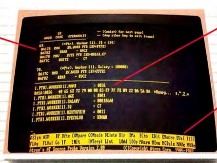
PROBE knows all about your local and complex variables. You can display and change an array of structures as easily as shown in this display.
