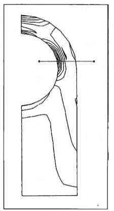
Figure 2: A stress-contour plot for the lifting lug in figure 1, generated in MSC/pal 2. The maximum stress occurs near the horizontal axis of the circular portion of the lug.
