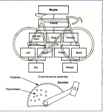
Figure 3: A hierarchical data organization, showing graphics primitives and structure elements.
