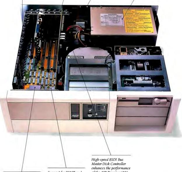
20 MHz, 80386 processor for high performance, AT-compatible desktop computing. Support for 80287 and 80387 coprocessors provides users with a choice for computationintensive applications. Master Disk Controller enhances the performance of the AST Premium/386. Offers users one of the highest performing 80386based, AT-compatible desktop systems available.
