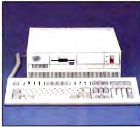
IBM PS/2 Model 50 • 80286, 10 MHz • 128K ROM, 1 MB RAM • 20 MB Hard Drive • 1.44 MB 3.5" Disk Drive
