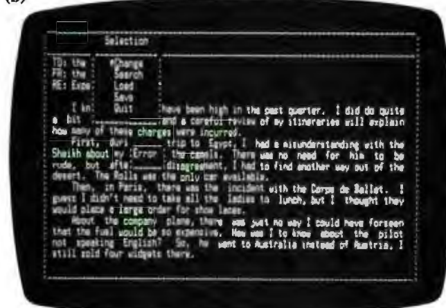
Photos 2a and 2b: BASIC-180's multitasking windows are sophisticated enough to simulate a Macintosh environment on a serial terminal, as shown in (a) and (b) above.
