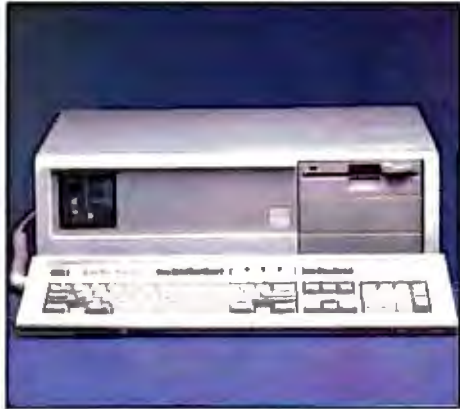
AST Premium Model 140 • 1.2 MB Floppy, 101 Keyboard • FastRAM 1MB • 80286, 10MHz, Zero Wait • AST 3 G Plus Board
