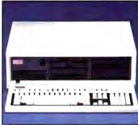
COMPAQ DeskPro 386/20 Model 60 • 80386 Processor, 20 MHz • 1 MB RAM, 1.2 Floppy • 60 MB Hard Drive • Parallel and Serial Ports
