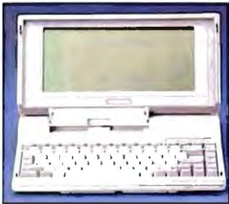
TOSHIBA T-1000 Lap Top • Fully IBM compatible • 512K RAM • 720K 3 1/2" Disk Drive • 640 x 200 Pixels
