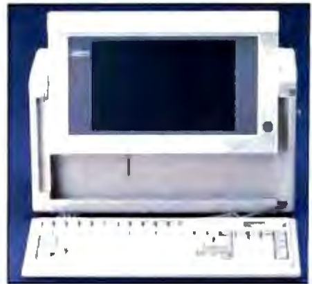
COMPAQ Portable 386 Model 40 • 80386 Processor • 1 Megabyte RAM • 40 MB Fixed Drive • 1.3 MB Diskette Drive
