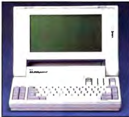
NEC Multispeed EL • Dual 3 1/2" 720K Floppies • 640K RAM, 512K ROM • Backlit LCD Screen • 9.54 MHz CMOS V-30
