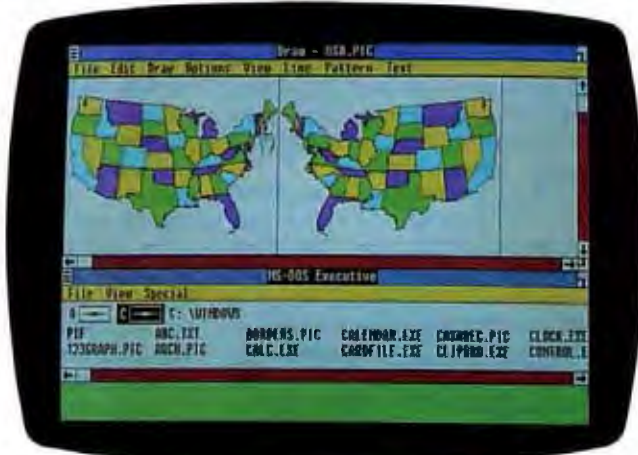
Photos 4 and 5: Microsoft's Windows 1.03 running under EGA (left) and VGA (right) modes illustrates the increased resolution that VGA offers.
