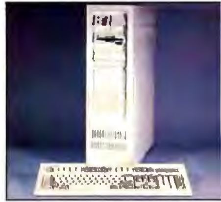
IBM PS/2 Model 80 • 80386, 16 MHz Micro Processor • 1 MB RAM, VGA Display • 40 MB Fixed Disk Drive • 1.44 MB 3.5" Disk Drive
