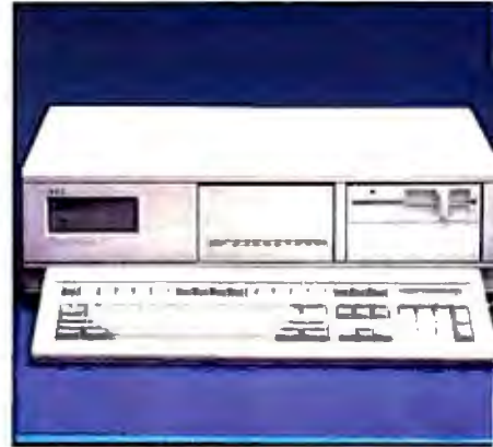
NEC PowerMate II • 1.2 MB Floppy Drive • 640K RAM, 10 MHz • 40 MB Fixed Disk Drive • MS-DOS 3.2 & GW-Basic
