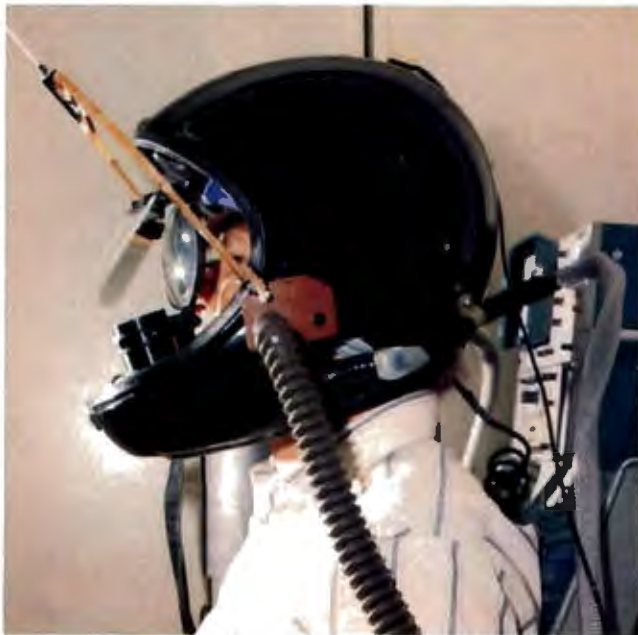
Photo 2: Used as a research tool at NASA's Langley facility, this helmet is a flight simulator that enables pilots to try out technologies such as eye tracking, voice recognition and synthesization, and three-dimensional graphics displays.
