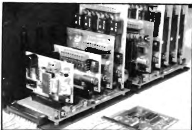
An A-BUS system with two Motherboards A-BUS adapter (IBM) in foreground
