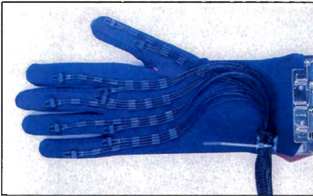
Photo 1: The DataGlove is a device that uses optical fiber sensors to measure and evaluate the range of joint movements, hyperextension, and abduction in the hand.
