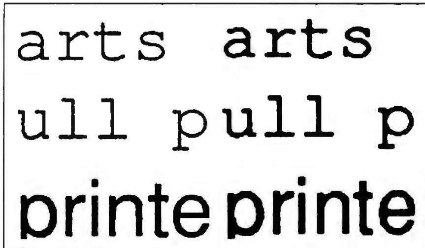
Figure 1: Finer characters are in the sample at left, from the 600-dpi Varityper VT600. The sample at right, from a QMS PS 810, shows 300-dpi resolution.
