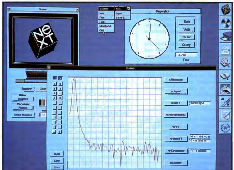
Photo 6: The cube's Workspace. Each window represents a running application. Note that the menu has its own Close box. The icons at the right represent "docked" applications.
