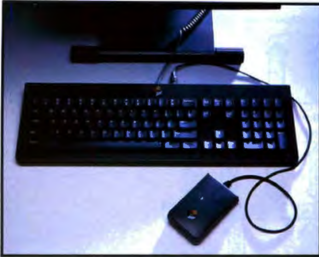
Photo 3: The cube's keyboard. The keys above the cursor keys control the monitor's brightness, the system's power, and sound volume.
