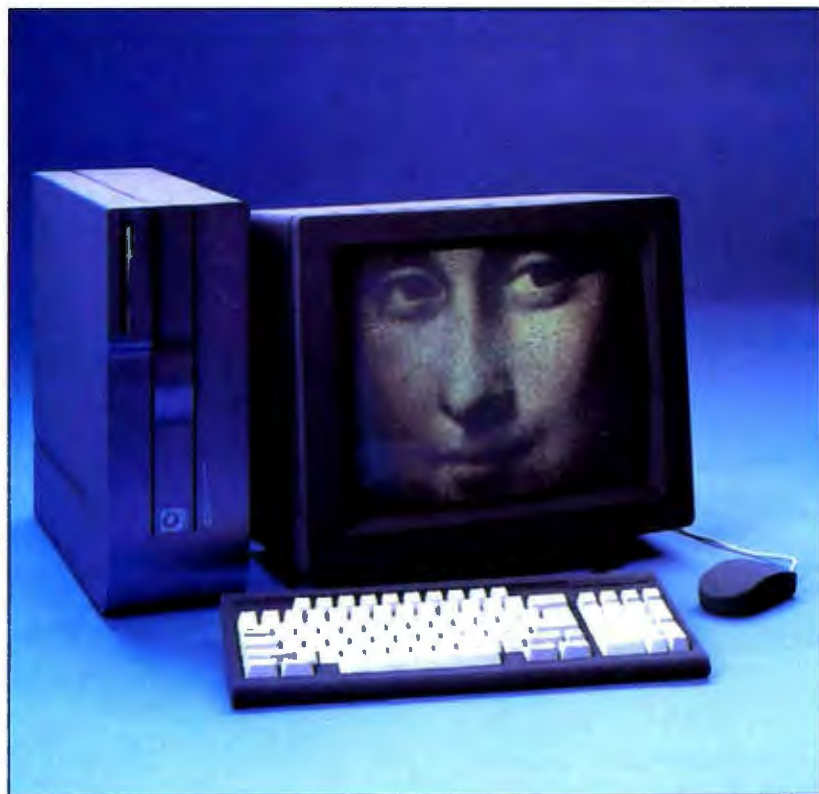
Photo A: Cogent Research's XTM parallel desktop supercomputer, based on the INMOS T800 transputer and Yale University's Linda programming language. (Photo courtesy of Cogent Research, Inc.)
