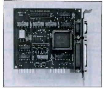
Boca Research's 10AT41 in a 25-pin/9-pin configuration.
