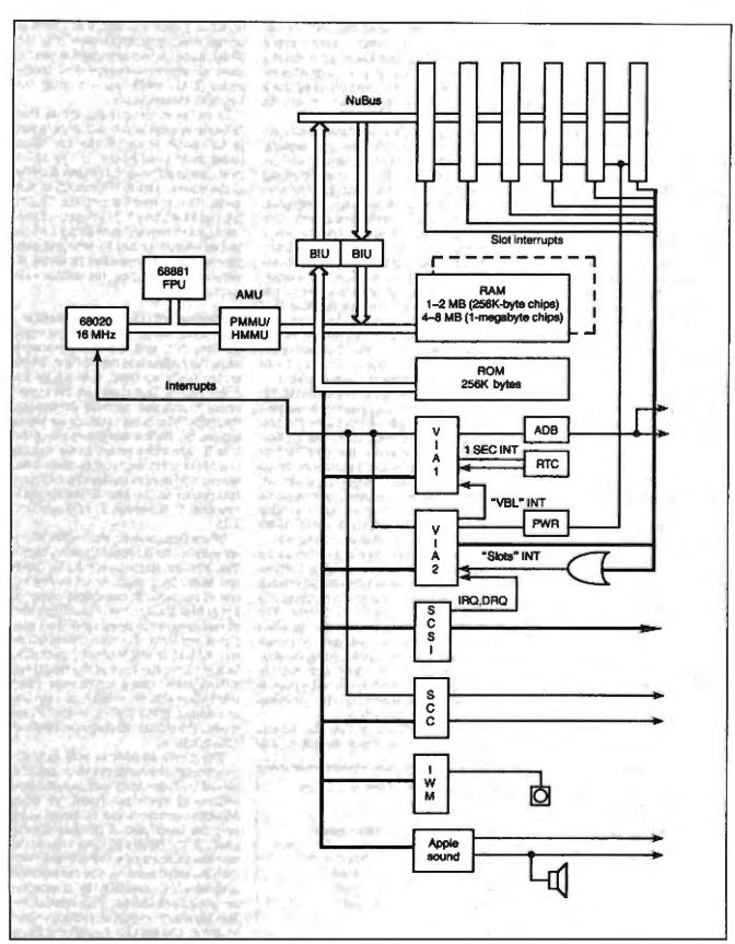
Figure 2: The Macintosh II system components.
