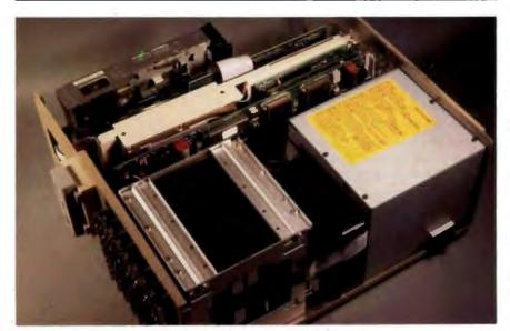
Photo 2: A prototype rack chassis, designed to hold eight cards (for a total of 64 processors). Note that this chassis also houses a Circuit Cellar AT, complete with a hard disk drive.
