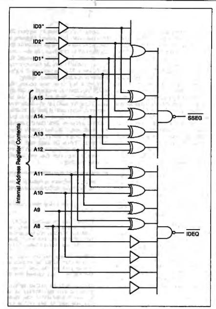
Figure B: Logic diagram of the 74BCT2420's comparator.
