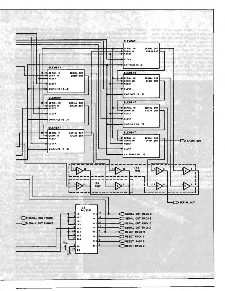
Each card has a single serial output line from all the processors on the card. All eight outputs in a rack are connected in common, so 64 open collector gates are tied together. Because I didn't think connecting 256 gates in four racks together made much sense, the Array Master card has a 74LS21 gate to combine the four signals into one. Remember that only one 8751 will be transmitting data on the serial line at a time, so only one of the 256 gates will be active.
