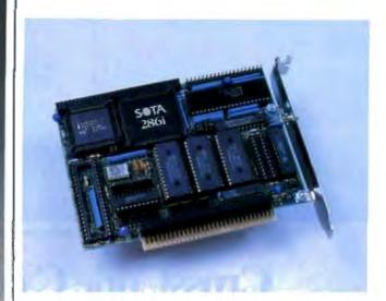
What's going on here is the 286i running the programs with no wait states on most read and write cycles.
