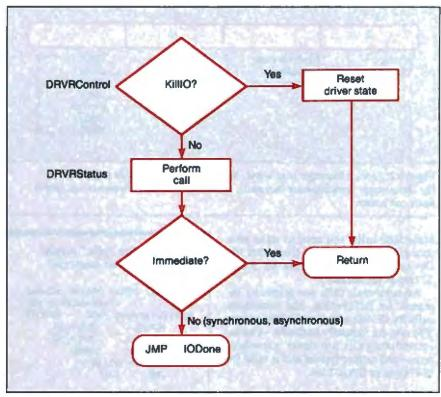
Figure 3: Flowchart illustrating control- and status-completion logic.
