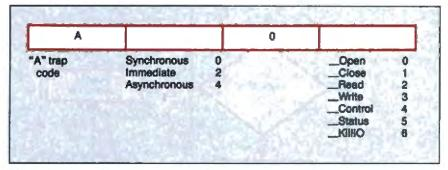
Figure 2: Device Manager trap word. Notice the seven possible traps and the three ways—synchronous (normal), immediate, or asynchronous—in which each can occur.
