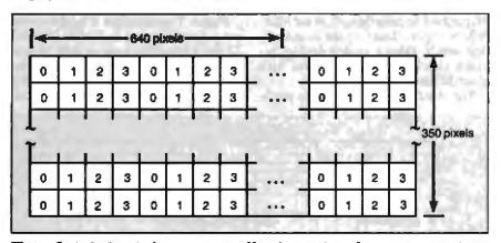
Figure 5: Assigning pixels to processors. If you're running a four-processor engine, the control program assigns pixels to successive processors by moving through the screen buffer horizontally left to right, then down.
