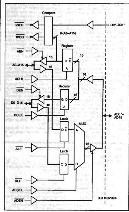
Figure A: Block diagram of the 74BCT2420 logic.
