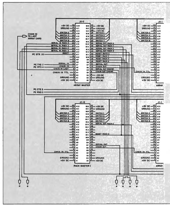
Figure 3: The complete schematic (sans buffers and support chips) for the Mandelbrot engine, detailing how the processors are chained together.
