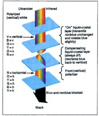
Figure 2: An "on" pixel polarizes light, which is then blocked by the front polarizer and appears as a black pixel on the white background.
