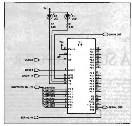
Figure 1: The schematic for one processing element of the Mandelbrot engine.
