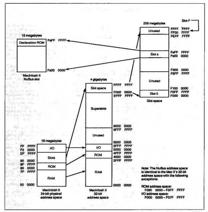
Figure 1: Memory map of the Macintosh II, 24-bit mode and 32-bit mode. Note that in the 24-bit mode, 8 megabytes of the available 16 megabytes is dedicated to on-board RAM. To properly fill the rest of the 24-bit address space, slots must have IDs ranging from 9 to E hexadecimal and are allocated only 1 megabyte.
