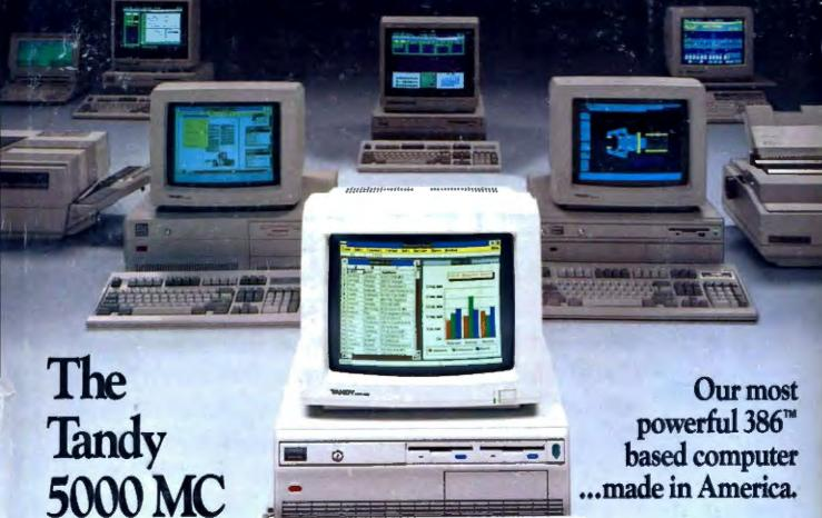
The new Tandy 5000 MC Professional System is pure performance, from the Intel® 80386 processor operating at 20 MHz to the memory cache controller that provides RAM-fast access to data.
