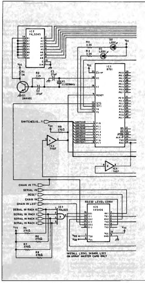
Figure 2: The schematic of a Mandelbrot engine card.
