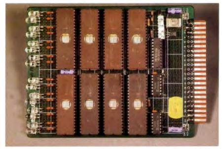
Photo 1: A prototype of one eight-processor card from the Mandelbrot engine. High-efficiency LEDs are along the left of the board, and notice the windows on each CPU for programming the on-chip EPROM.
