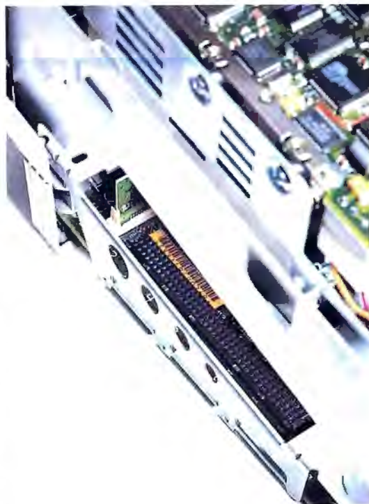
Photo 2a: The cramped insides of the Mac SE/30.
