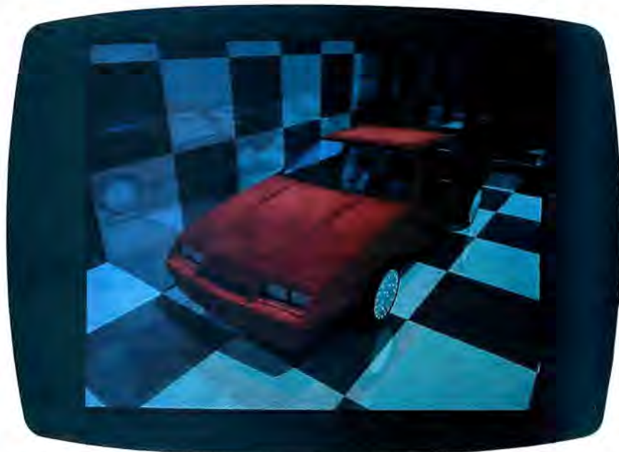
Photo 1: The ray-tracing feature of the HP 9000 TurboSRX engineering workstation from Hewlett-Packard allows you to produce the realistic highlights, reflections, and effect of transmittance seen in this screen shot. (The data to produce this image is courtesy of Chrysler. Photo courtesy of Hewlett-Packard.)
