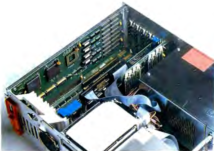
Photo 1: The CPU card is visible in the upper left corner. The card contains the 80386, a socket for an 80387 coprocessor, the 82385, and the SRAM cache chips.
